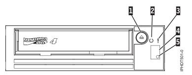
Figure 1. Front view of tape drive
