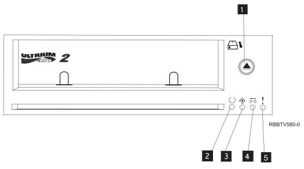
Figure 3. Front view of tape drive
