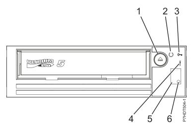
Figure 2. Front view of half high LTO Drive
