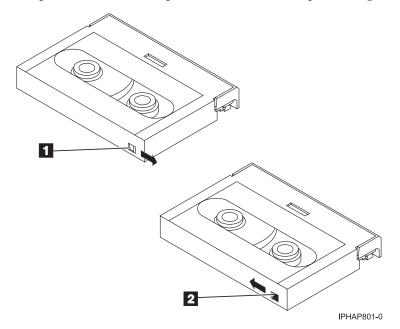
1 2 When the switch is set to the right, data can be written to and read from the tape When the switch is set to the left, data can only be read.
