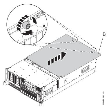
Figure 10. Removing the service access cover
