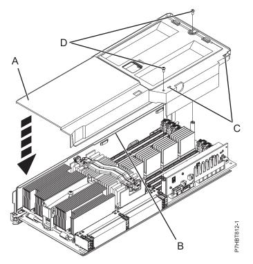
Figure 1. Installing the system processor assembly cover
