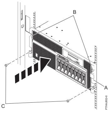
Figure 9. Installing the front cover
