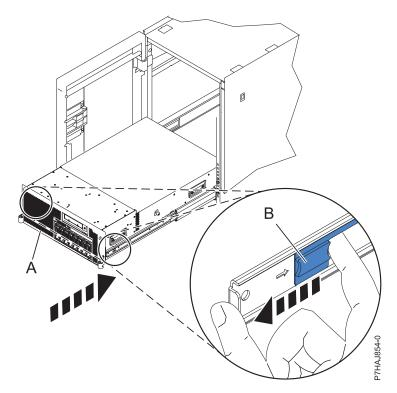
Figure 13. Releasing the rail safety latches
