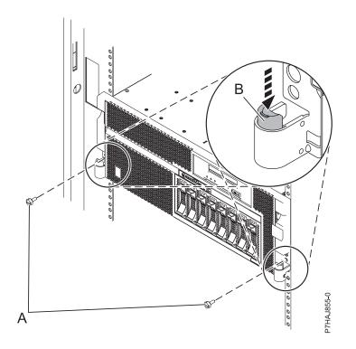
Figure 12. Releasing the rack latches
