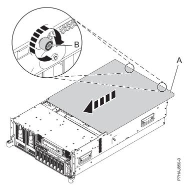
Figure 11. Installing the service access cover
