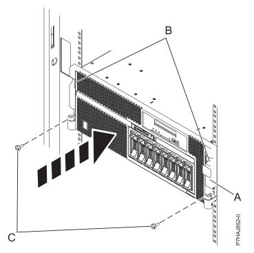
Figure 14. Replacing the thumbscrews
