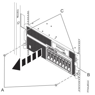
Figure 8. Removing the front cover
