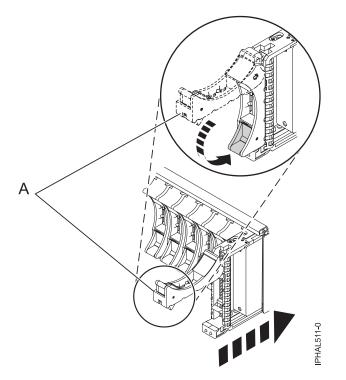
Figure 6. Installing a small-form factor disk drive in the 5803 expansion unit
