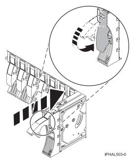
Figure 83. Installing a disk drive
