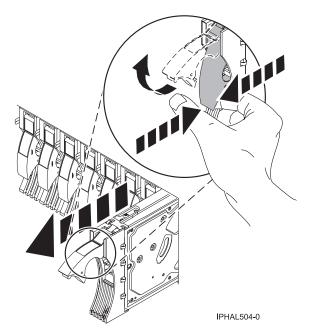
Figure 43. Removing a disk drive
