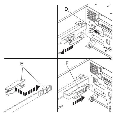
Figure 126. SAS cable connections
