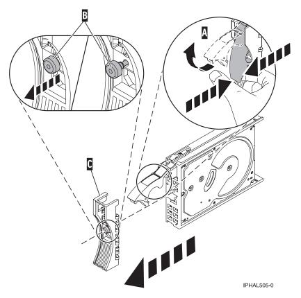
Figure 49. Removing a disk-drive bezel
