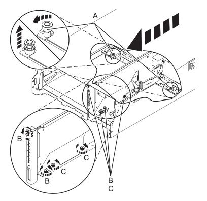
Figure 145. Removing the SAS conduit card and midplane
