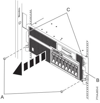
Figure 154. Removing the front cover
