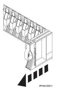
Figure 23. Removing a disk-drive filler from a model .
