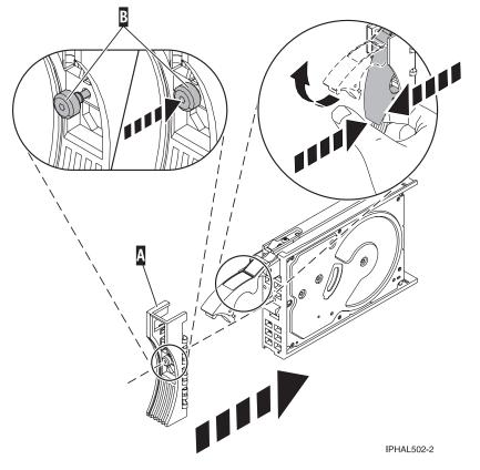
Figure 82. Installing a disk-drive bezel
