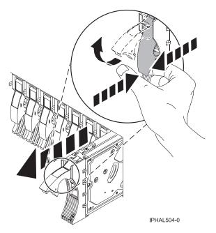
Figure 98. Removing a disk drive from a model or 7311-D20
