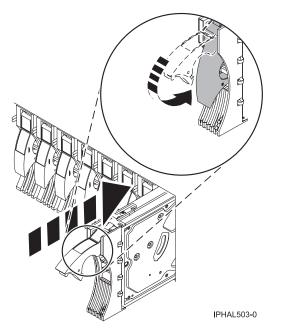
Figure 102. Installing a disk drive in a model a model or 7311-D20
