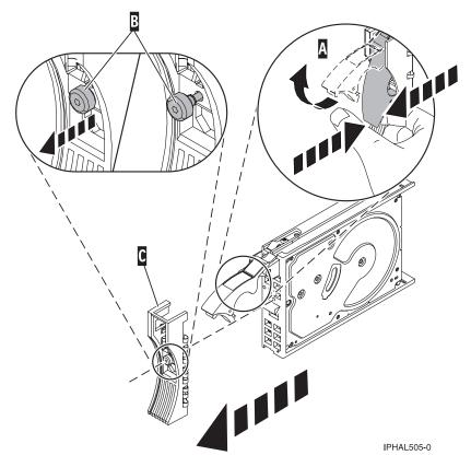
Figure 62. Removing a disk-drive bezel
