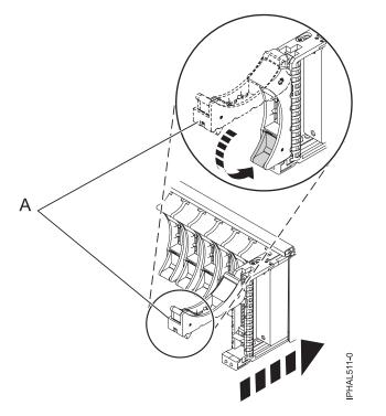
Figure 36. Installing a small-form factor disk drive in the 5803 expansion unit
