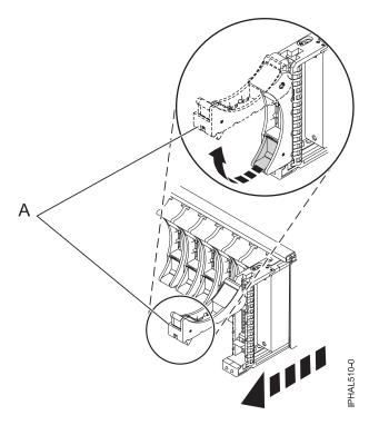
Figure 87. Removing a small-form factor disk drive from the 5803 expansion unit
