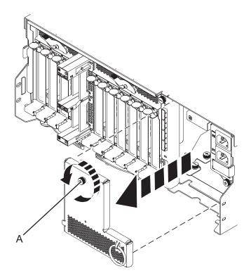
Figure 143. Removing the power cord plate
