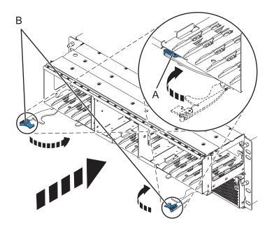
Figure 136. Installing the backplane on a rack-mounted model
