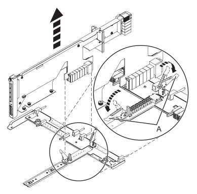
Figure 146. Removing the SAS conduit card from the midplane
