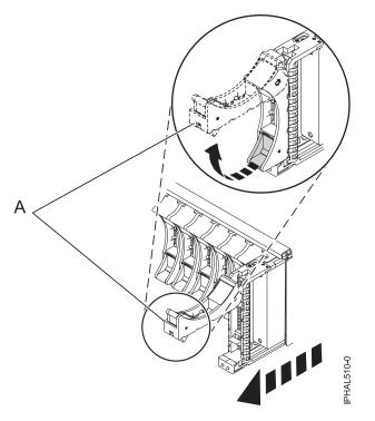
Figure 99. Removing a small-form factor disk drive from the 5803 expansion unit
