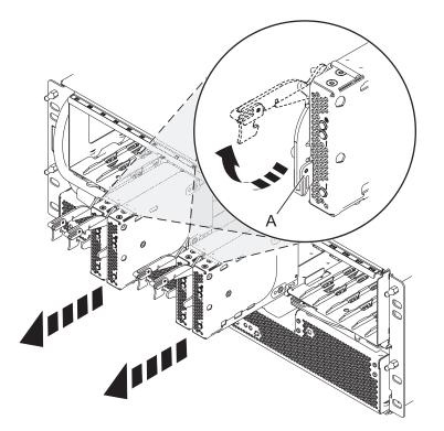
Figure 148. Removing the SAS expander card.
