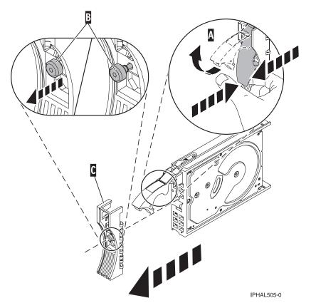
Figure 81. Removing a disk-drive bezel
