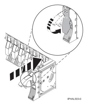
Figure 51. Installing a disk drive in a model
