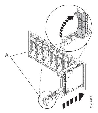
Figure 67. Installing a small-form factor disk drive
