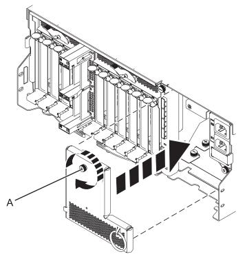
Figure 132. Installing the power cord plate
