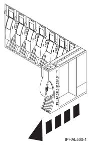
Figure 37. Removing a disk-drive filler from a model
