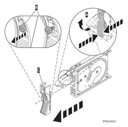
Figure 100. Removing a disk-drive bezel
