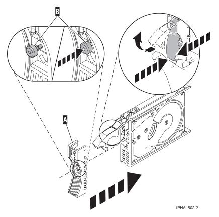
Figure 9. Installing a disk-drive bezel
