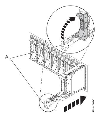
Figure 11. Installing a small-form factor disk drive
