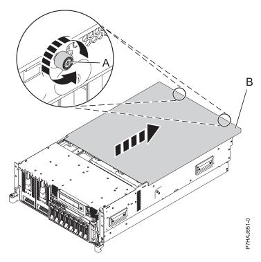
Figure 152. Removing the service access cover
