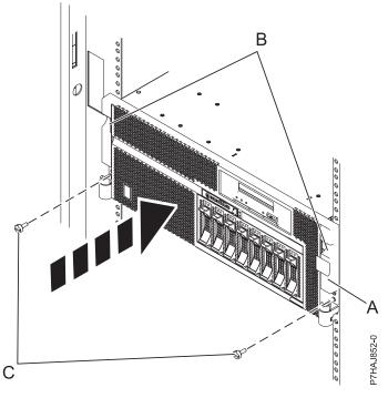
Figure 155. Installing the front cover
