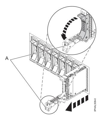
Figure 47. Removing a small-form factor disk drive
