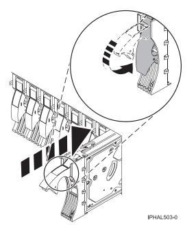
Figure 77. Installing a disk drive in a model or 7311-D20
