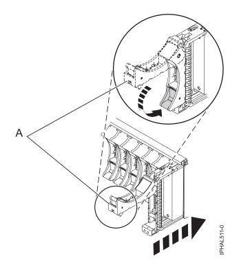
Figure 68. Installing a small-form factor disk drive in the 5803 expansion unit
