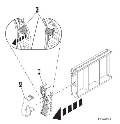
Figure 105. Removing a disk-drive bezel
