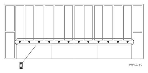
Figure 115. Back view of SCSI disk-drive enclosure concurrent maintenance lights for model 5786, 5787, 7031-D24, and 7031-T24
