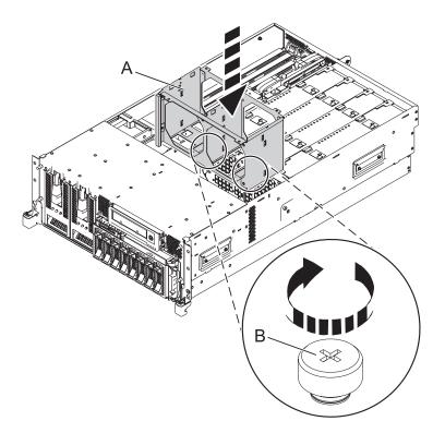
Figure 127. Installing the fan cage in the 8233-E8B or 8236-E8C system
