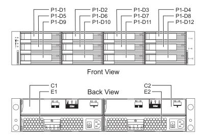
Figure 110. Disk drive locations for the 5886 disk enclosure
