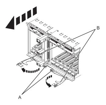
Figure 144. Removing the I/O planar
