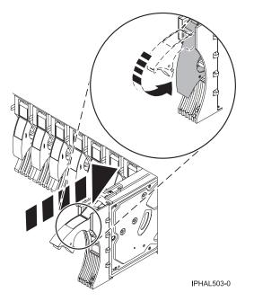
Figure 34. Sliding the disk drive in to the system unit
