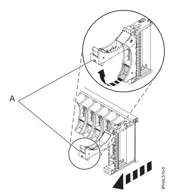
Figure 45. Removing a small-form factor disk drive from the 5803 expansion unit
