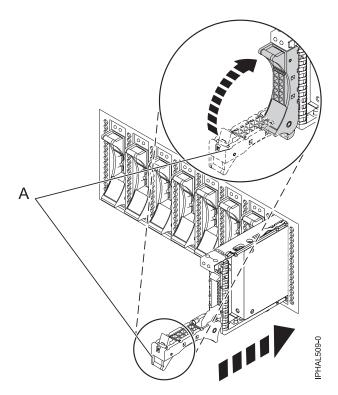
Figure 41. Installing a small-form factor disk drive
