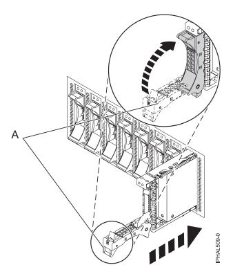
Figure 52. Installing a small-form factor disk drive
