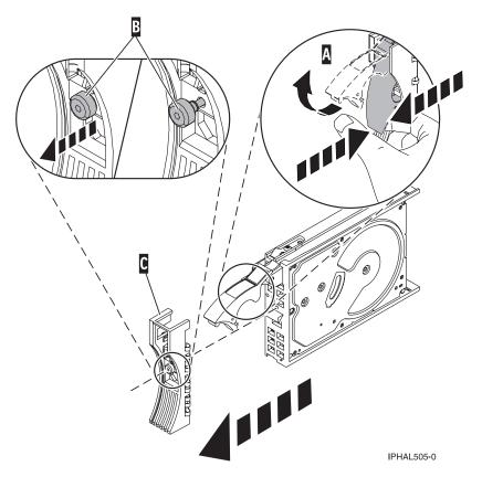
Figure 74. Removing a disk-drive bezel
