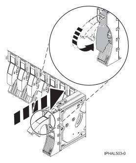
Figure 90. Installing a disk drive
