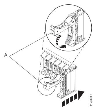
Figure 97. Installing a small-form factor disk drive in the 5803 expansion unit
