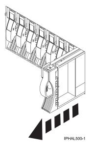
Figure 30. Removing a disk-drive filler
