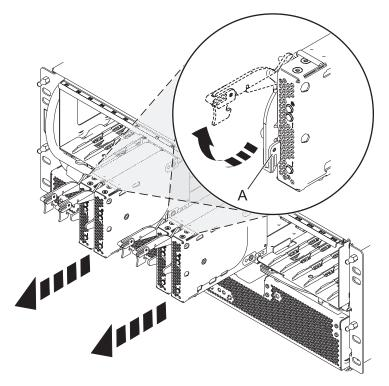
Figure 138. Removing the port card from the backplane
