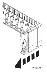
Figure 16. Removing a disk-drive filler from model
