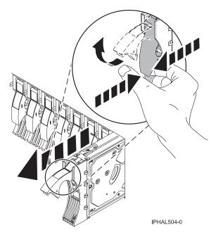
Figure 46. Removing a disk drive from a model
