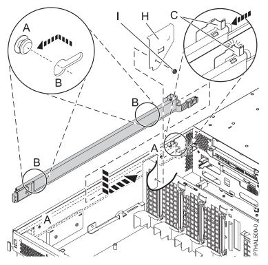
Figure 125. Attaching the SAS cable
