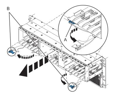
Figure 139. Removing the backplane from the enclosure
