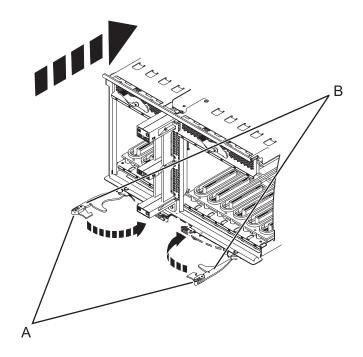
Figure 134. Install the I/O planar on a rack mounted model
