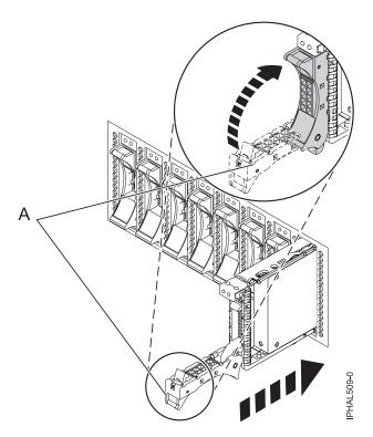
Figure 20. Installing a small-form factor disk drive
