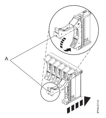
Figure 91. Installing a small-form factor disk drive in the 5803 expansion unit
