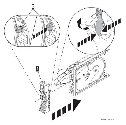
Figure 39. Installing a disk-drive bezel
