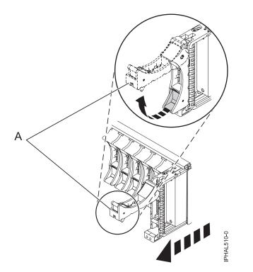
Figure 61. Removing a small-form factor disk drive from the 5803 expansion unit
