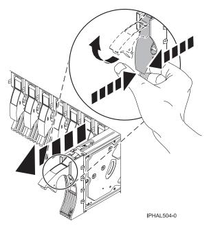
Figure 86. Removing a disk drive
