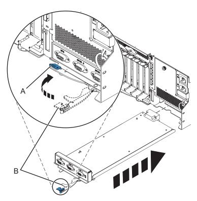
Figure 133. Replacing the enclosure management controller
