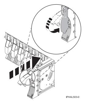
Figure 19. Installing a disk drive in a model
