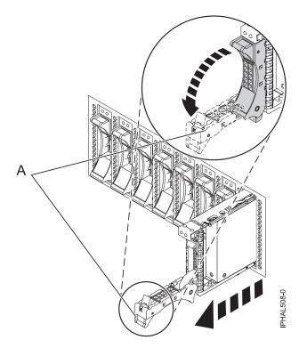
Figure 44. Removing a small-form factor disk drive
