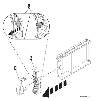
Figure 38. Removing a disk-drive bezel
