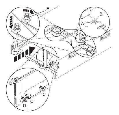
Figure 131. Installing the SAS conduit card and the midplane
