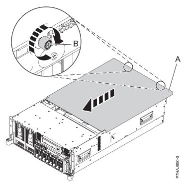
Figure 153. Installing the service access cover
