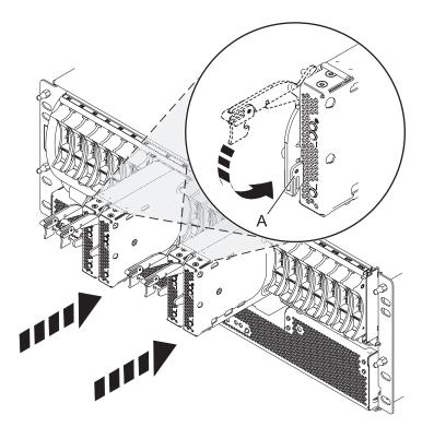
Figure 147. Installing the SAS expander card
