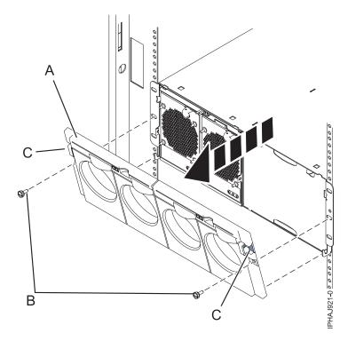
Figure 150. Remove the front cover for model 7314-G30 or 5796
