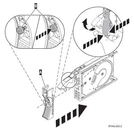
Figure 89. Installing a disk-drive bezel
