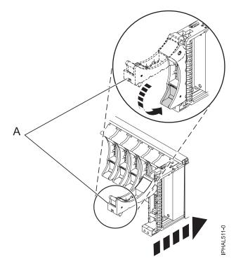
Figure 21. Installing a small-form factor disk drive in the 5803 expansion unit
