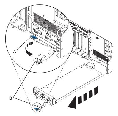
Figure 142. Remove the enclosure management controller
