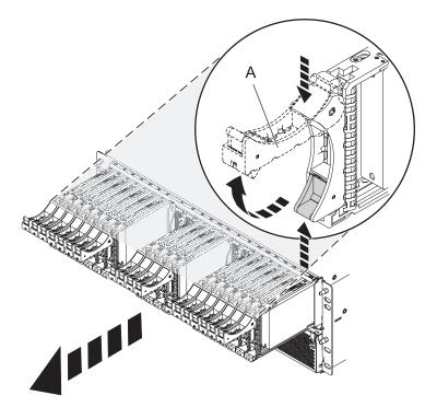
Figure 137. Removing the disk drives from the backplane
