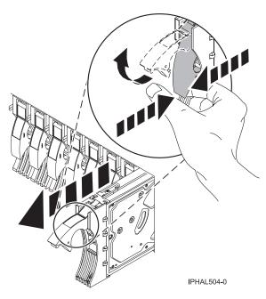
Figure 80. Removing a disk drive
