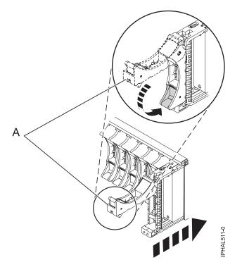
Figure 53. Installing a small-form factor disk drive in the 5803 expansion unit
