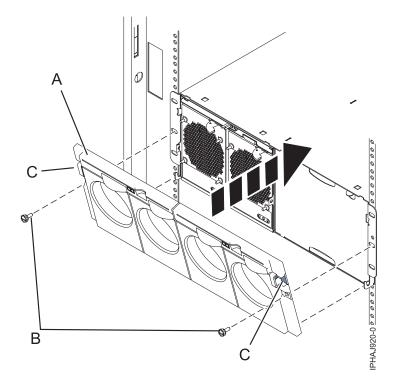
Figure 151. Front cover on a model 7314-G30 or 5796
