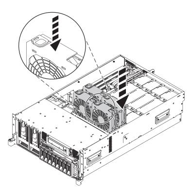
Figure 129. Installing the fans in the 8233-E8B or 8236-E8C fan cage
