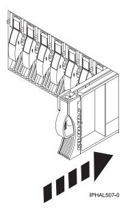
Figure 107. Installing a disk-drive filler
