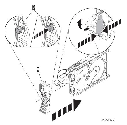
Figure 101. Attaching a disk-drive bezel
