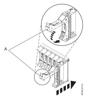
Figure 103. Installing a small-form factor disk drive in the 5803 expansion unit
