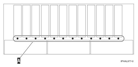
Figure 114. Front view of SCSI disk-drive enclosure concurrent maintenance lights for model 5786, 5787, 7031-D24, and 7031-T24
