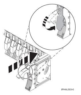
Figure 40. Installing a disk drive in a model
