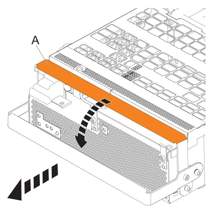
Figure 141. Remove the offline converter assemblies
