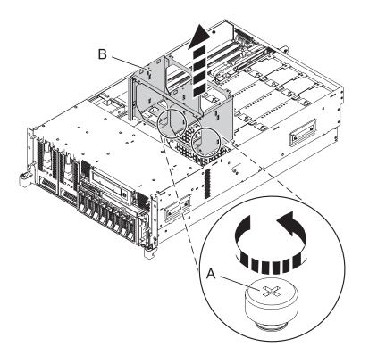
Figure 124. Removing the fan cage from the 8233-E8B or 8236-E8C system
