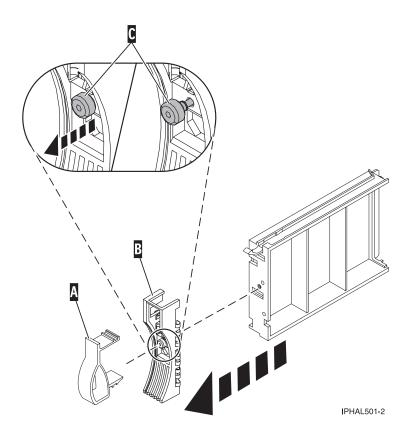
Figure 31. Removing a disk-drive bezel
