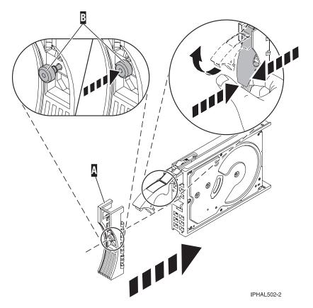
Figure 63. Attaching a bezel to the disk drive
