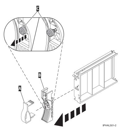
Figure 8. Removing the disk-drive bezel
