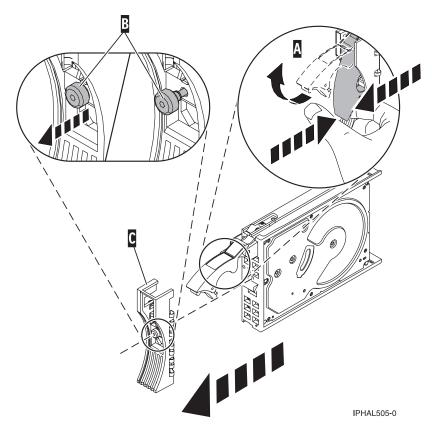
Figure 88. Removing a disk-drive bezel
