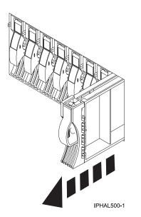
Figure 7. Removing a disk-drive filler from model
