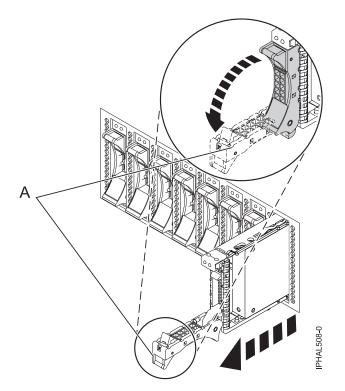
Figure 60. Removing a small-form factor disk drive
