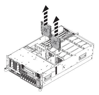
Figure 123. Removing the air baffles from the 8233-E8B or 8236-E8C fan cage
