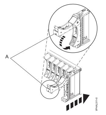
Figure 42. Installing a small-form factor disk drive in the 5803 expansion unit
