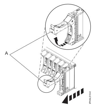
Figure 93. Removing a small-form factor disk drive from the 5803 expansion unit
