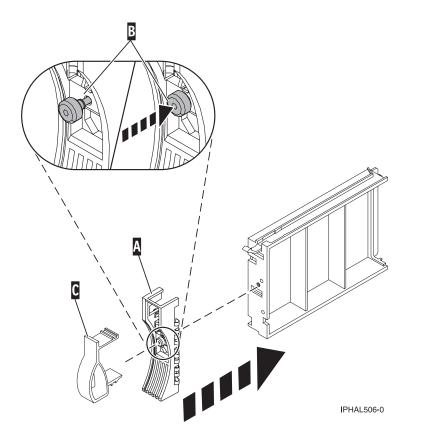
Figure 106. Attaching a bezel to a disk-drive filler
