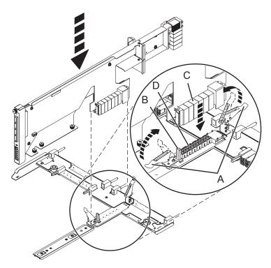
Figure 130. Installing the SAS conduit card into the midplane
