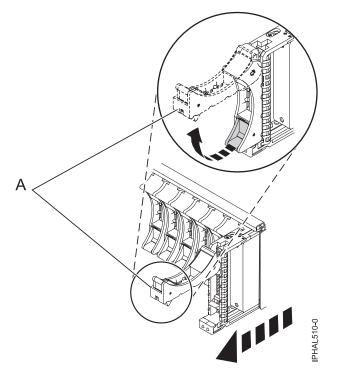
Figure 48. Removing a small-form factor disk drive from the 5803 expansion unit
