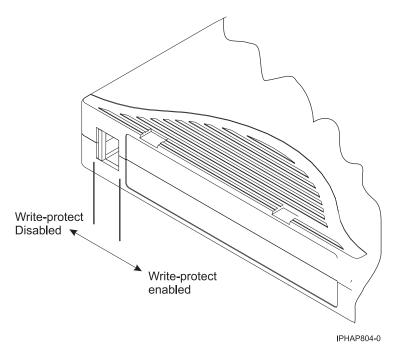
Figure 3. Setting the Write-Protect switch
