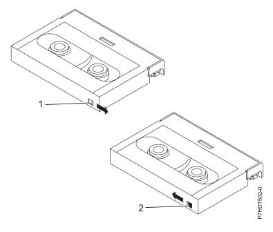
When the switch is set to the right, data can be written to and read from the tape.
