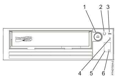
Figure 2. Front view of a half-high LTO tape drive
