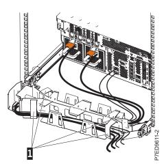
Figure 16. Power cord attachment and routing
