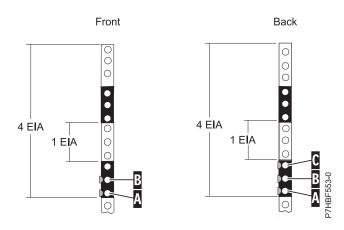
Figure 2. Marking holes on the front and rear of the rack frame
