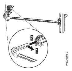
Figure 13. Pin extended with bracket installed into slide rail
