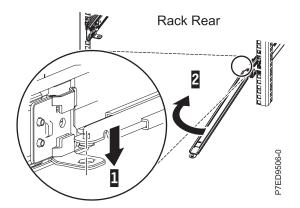
Figure 11. Support arm connection
