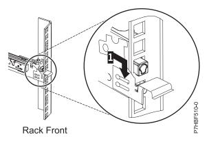
Figure 5. Rack front rail with pins seated
