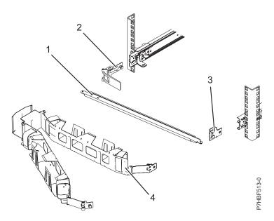
Figure 10. Relative positions of cable-management arm parts before assembly
