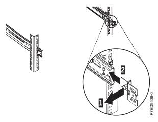
Figure 14. Mounting bracket pin extended and mounting bracket installed into slide rail
