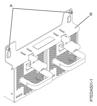
Figure 9. Shipping bracket removal
