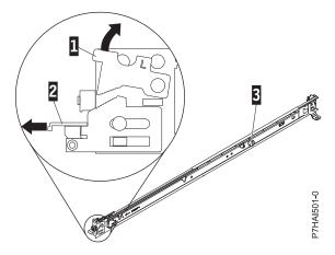
Figure 3. Slide rail and movable tab
