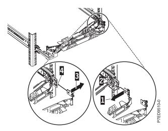
Figure 15. Cable-management arm connection
