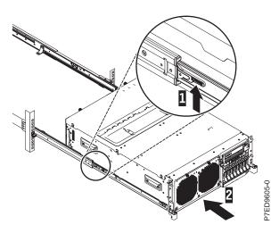
Figure 8. Release latches and server
