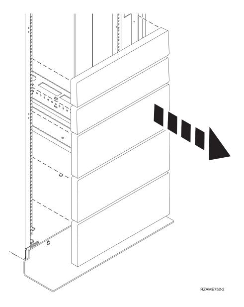
Figure 1. Removing the filler panels
