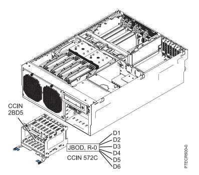
Figure 4. Disk bays controlled by base backplane
