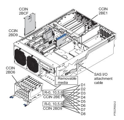
Figure 7. Disk bays controlled by both embedded SAS adapters when using SAS dual-RAID subsystem with external drives
