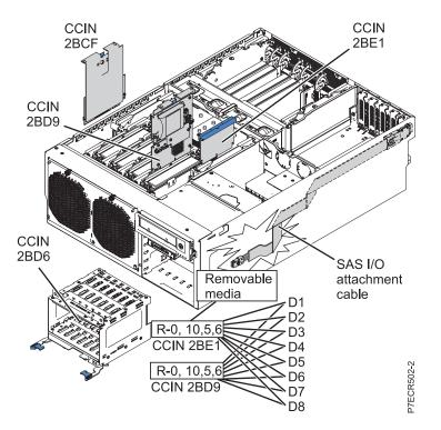
Figure 6. Disk bays controlled by both embedded SAS adapters when using SAS dual-RAID subsystem with internal drives
