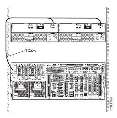
Figure 8. Physical connection to attach external disk enclosures
