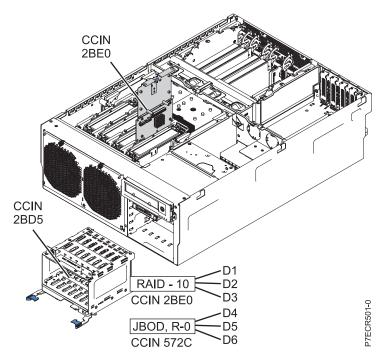
Figure 5. Embedded SAS adapter in a two-way split drive backplane
