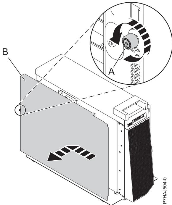
Figure 83. Installing the outside service access cover
