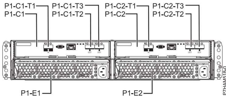
Figure 45. Rear view of the 58/87 disk drive enclosure
