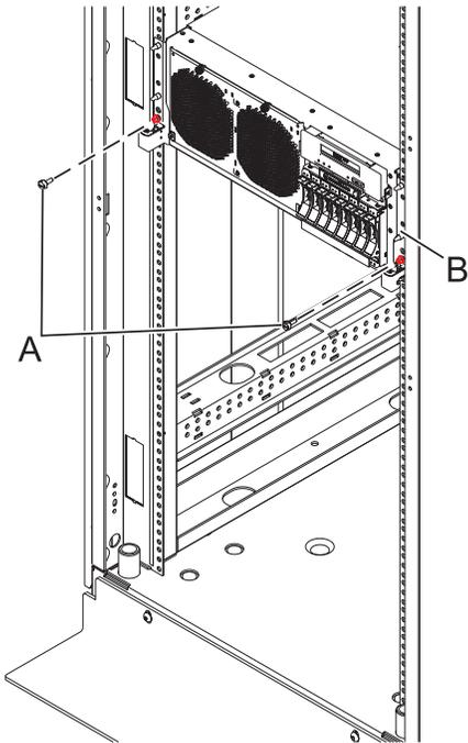
Figure 108. Placing the system in the service position
