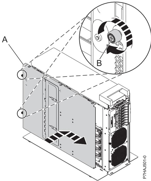
Figure 86. Installing the inside service access cover
