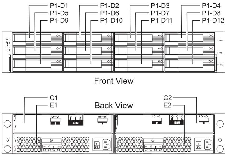
Figure 42. Disk drive locations for the 58/86 disk-drive enclosure
