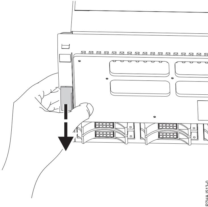
Figure 98. Releasing the cover latches
