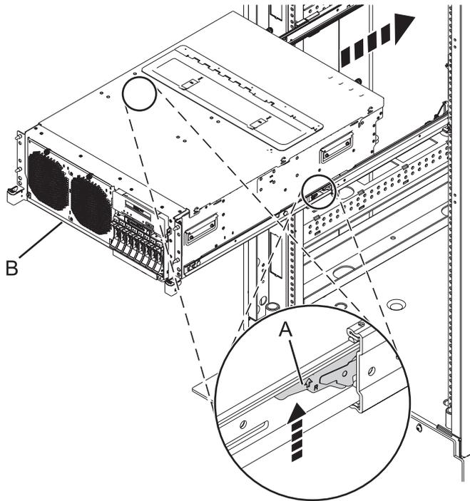
Figure 109. Placing the system into the operating position
