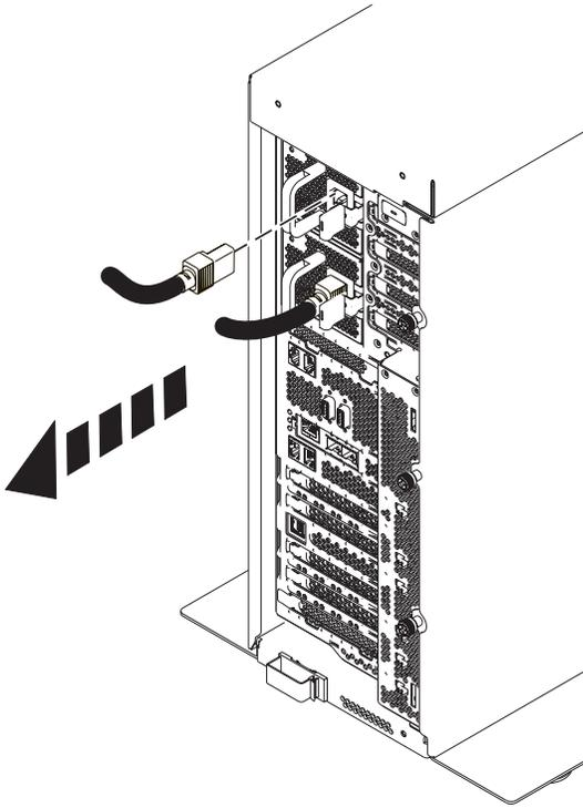
Figure 118. Removing the power cords for a stand-alone system
