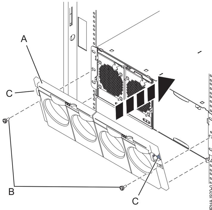
Figure 76. Front cover on a model 14G/30
