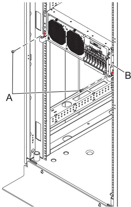
Figure 105. Placing the system in the service position
