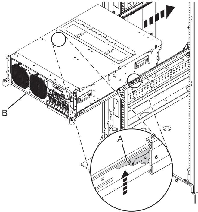
Figure 106. Placing the system into the operating position
