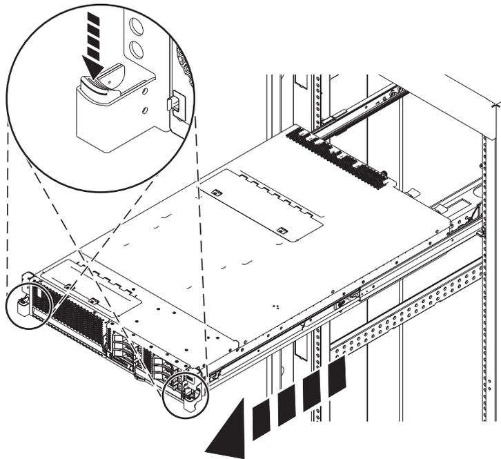
Figure 111. Placing the system in the service position
