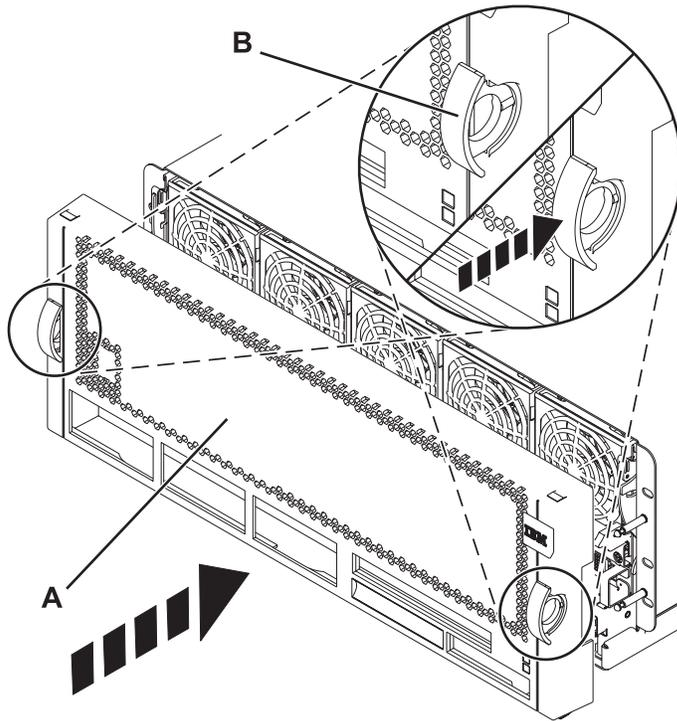
Figure 101. Installing the front cover
