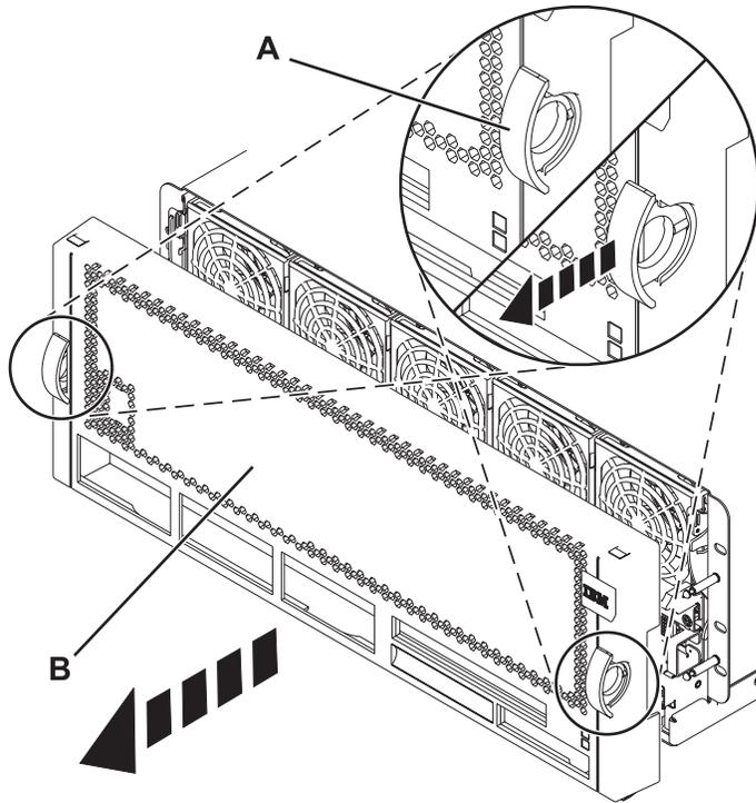
Figure 94. Removing the front cover
