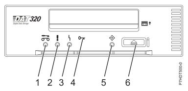
Figure 10. Front view of tape drive
