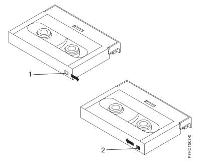
When the switch is set to the right, data can be written to and read from the tape. 2 When the switch is set to the left, data can only be read.
