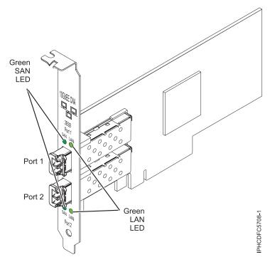
Figure 29. 10-Gb FCoE PCIe Dual Port Adapter
