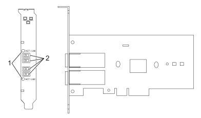
Figure 33. 2-Port Gigabit Ethernet-SX PCI Express Adapter
