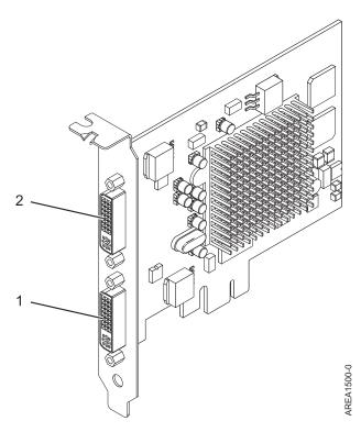
Figure 17. POWER GXT145 PCI Express Graphics Accelerator adapter
