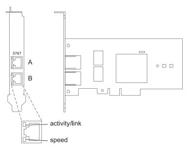
Figure 32. 2-Port 10/100/1000 Base-TX Ethernet PCI Express Adapter
