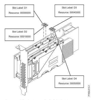
Figure 43. PCIe Dual - x4 3 Gb SAS RAID Adapter
