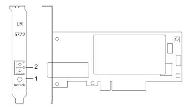
Figure 35. 10 Gigabit Ethernet-LR PCI Express Adapter
