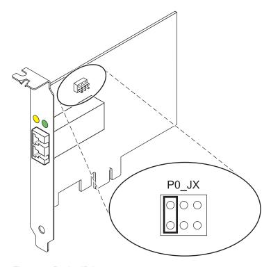
Figure 12. Device ID jumper
