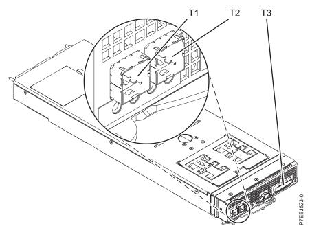
Note: Connectors T1 and T2 are not used on FC 58/88 PCIe storage enclosure.
