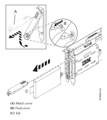
Figure 51. Replacing the 572F/575C cache battery
