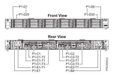
Figure 48. Location codes of the PCIe2 3.1GB Cache Integrated SAS RAID adapter
