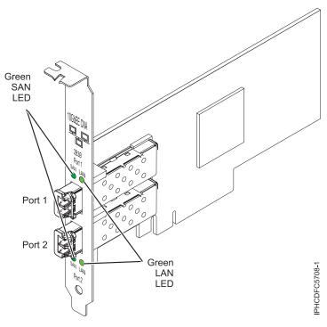
Figure 19. PCIe LP 10-Gb FCoE 2-port Adapter
