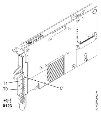
Figure 45. PCIe Dual - x4 3 Gb SAS RAID Adapter
