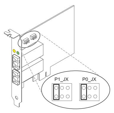
Figure 8. Device ID jumper
