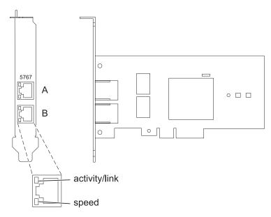
Figure 37. PCIe LP 2-Port 1GbE TX adapter
