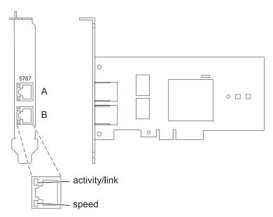
Figure 27. 2-Port 10/100/1000 Base-TX Ethernet PCI Express Adapter
