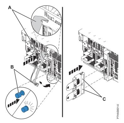
Figure 7. Installing the cable retention bracket
