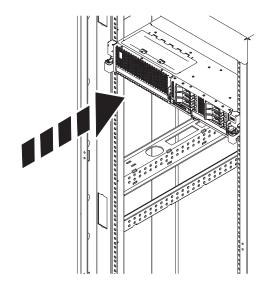
Figure 14. Placing the system in the operating position
