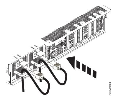
Figure 16. Connecting the power cords
