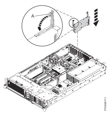
Figure 2. Installing the FC EJ0H in a system
