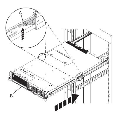
Figure 13. Unlocking the safety rail latches
