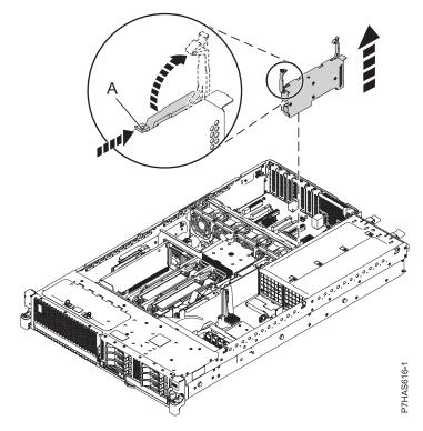
Figure 5. Adapter removal from a system
