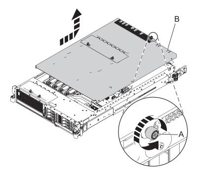
Figure 10. Removing the service access cover
