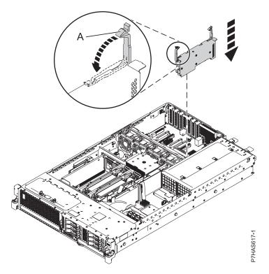
Figure 6. Installing the FC EJ0H GX adapter in a system
