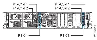
Figure 1. GX adapter slots and location codes
