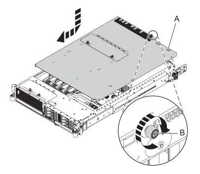
Figure 11. Installing the service access cover
