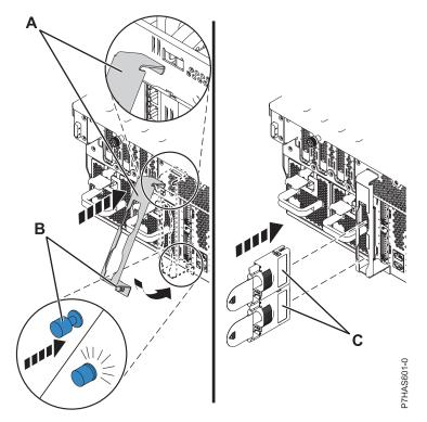
Figure 3. Installing the cable retention bracket
