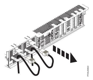
Figure 15. Removing the power cords
