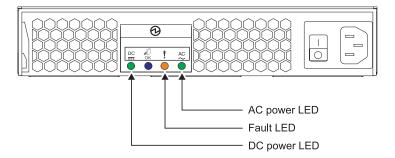
Figure 1. Rear view of power supply
