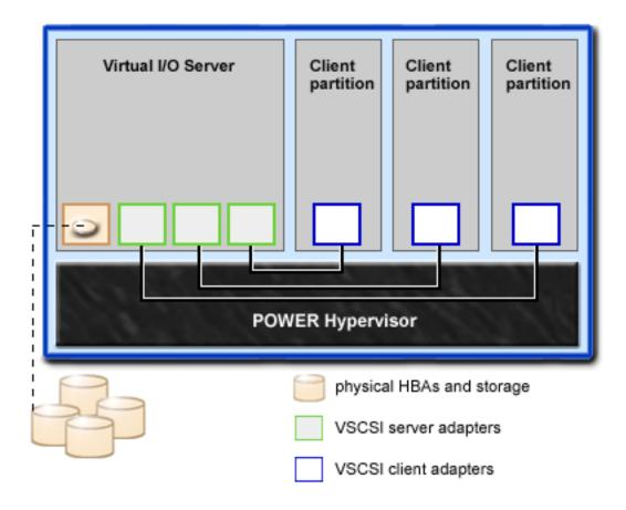
**Note:** In order for client logical partitions to be able to access virtual devices, the Virtual I/O Server must be fully operational.
