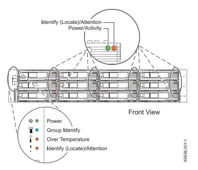
Figure 82. Front view of 58/86 disk-drive enclosure concurrent maintenance lights
