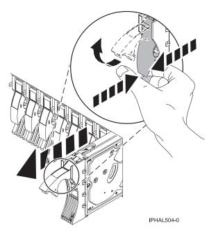
Figure 40. Removing a disk drive from a model or 11D/20
