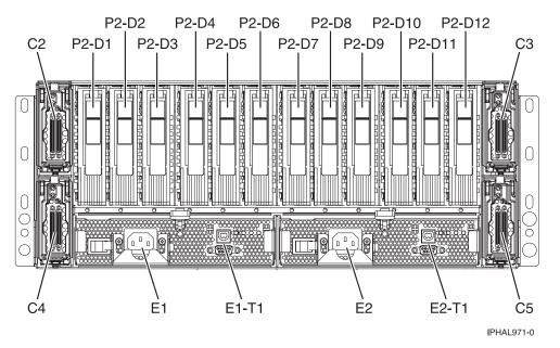
Figure 73. Repeater card location of the and 31D/24 SCSI disk-drive enclosure (drawer models)
