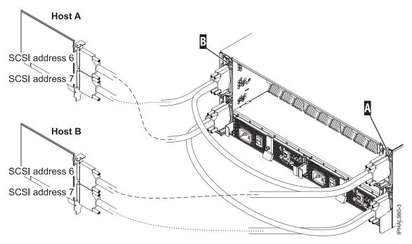
Figure 64. SCSI cable to dual repeater card connected with two SCSI cards
