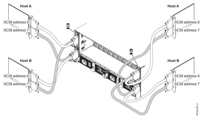
Figure 65. SCSI cable to dual repeater card connected with four SCSI cards
