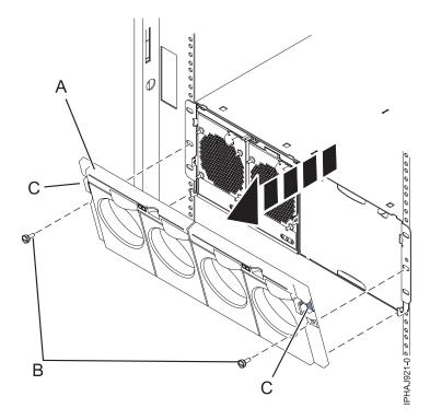
Figure 93. Remove the front cover for model 14G/30
