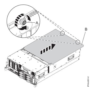
Figure 96. Remove the service access cover from a rack-mounted model
