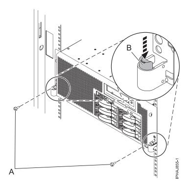
Figure 110. Releasing the rack latches
