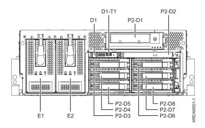
Figure 59. Disk drive locations for the SAS disk drives
