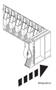
Figure 56. Installing a disk-drive filler
