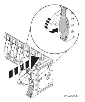
Figure 8. Installing a disk drive in a model
