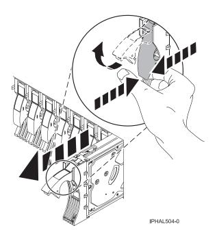
Figure 30. Removing a disk drive from a model or 11D/20
