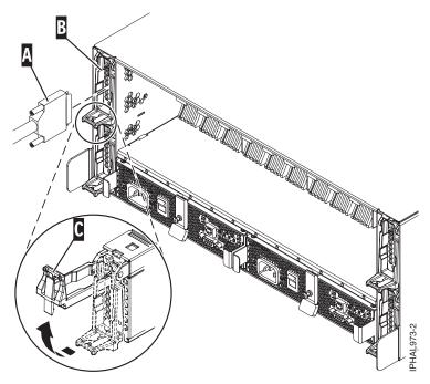
Figure 77. Removing SCSI cable from repeater card
