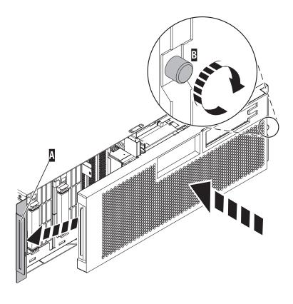
Figure 105. Installing the front cover
