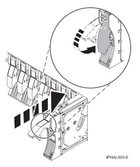
Figure 24. Installing a disk drive in a model
