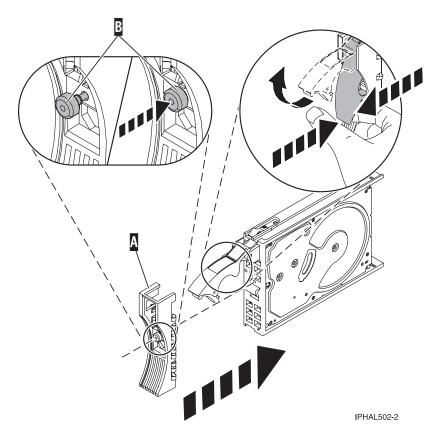
Figure 47. Attaching a disk-drive bezel
