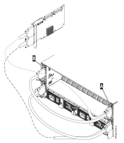
Figure 66. SCSI cable to dual repeater card connected to single repeater card
