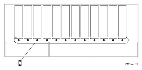
Figure 80. Front view of model 31D/24 or 31T/24 SCSI disk-drive enclosure concurrent maintenance lights
