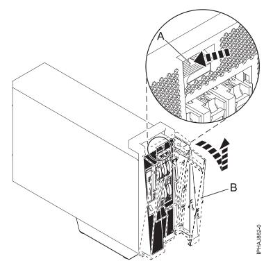
Figure 102. Remove the door from the model
