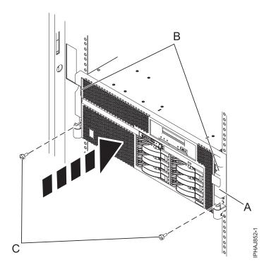
Figure 109. Pushing the system into the rack and attaching the thumbscrews
