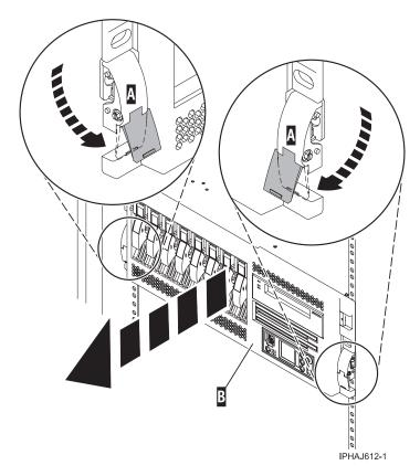
Figure 107. Releasing the rack latches
