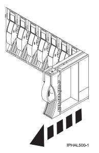
Figure 17. Removing a disk-drive filler from a model
