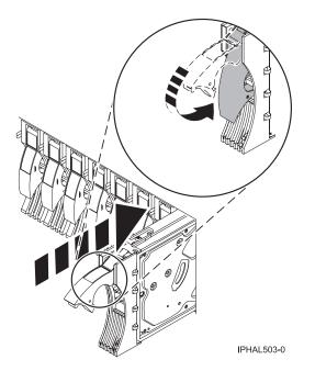
Figure 48. Installing a disk drive in a model or 11D/20
