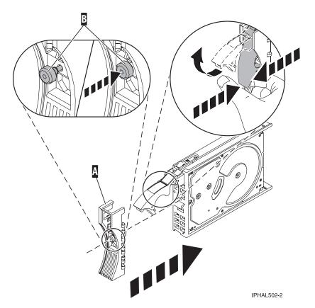
Figure 42. Attaching a bezel to the disk drive
