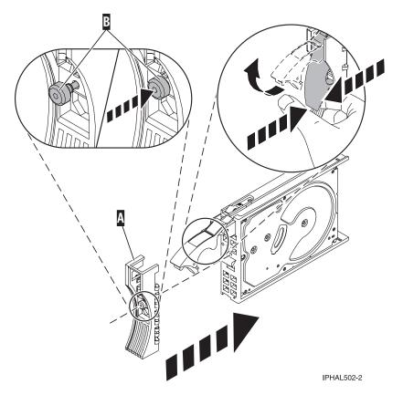
Figure 32. Attaching a bezel to the disk drive
