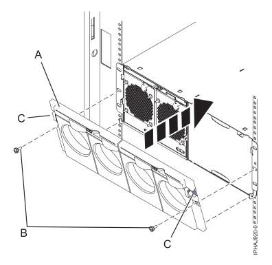
Figure 94. Front cover on a model 14G/30
