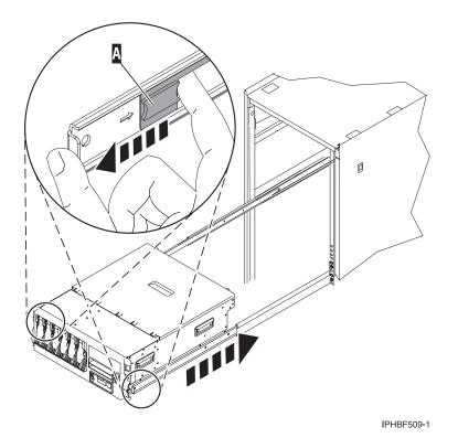
Figure 108. Releasing the rail safety latches
