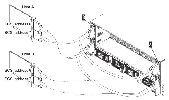
Figure 67. SCSI cable to dual repeater card connected with two SCSI cards
