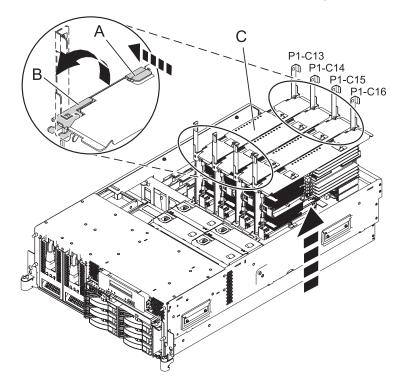
4. Remove the fan cage by turning the thumbscrews **A** to release the cage, **B** then lift the cage out of the system as shown in the following figure.
