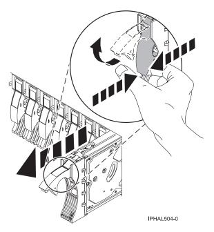
Figure 45. Removing a disk drive from a model or 11D/20
