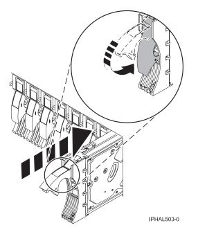
Figure 44. Installing a disk drive in a model or 11D/20
