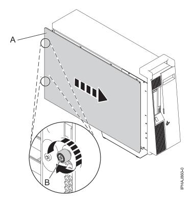
Figure 99. Installing the service access cover on a stand-alone model
