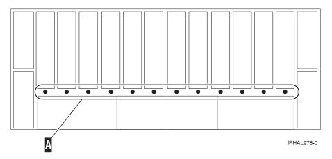
Figure 81. Back view of model 31D/24 or 31T/24 SCSI disk-drive enclosure SCSI disk-drive enclosure concurrent maintenance lights
