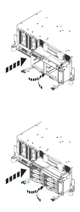
Figure 88. Install the disk drive backplane on a rack mounted model
