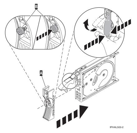
Figure 7. Installing a disk-drive bezel
