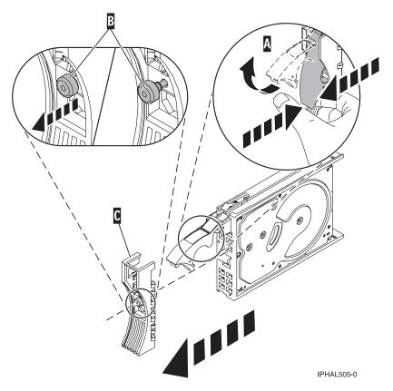
Figure 41. Removing a disk-drive bezel
