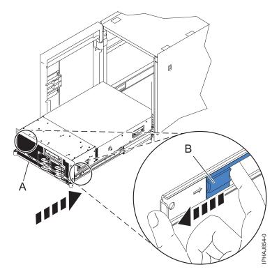
Figure 111. Releasing the rail safety latches
