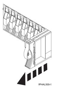
Figure 53. Removing a disk-drive filler from a model or 11D/20
