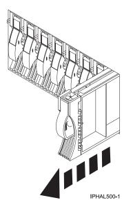
Figure 1. Removing a disk-drive filler from a model .
