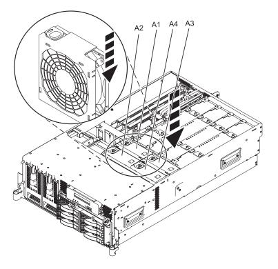
b. Replace the air baffle by inserting the baffle into place and pushing each of the locking tabs down to secure the baffle, as shown in the following figure.
