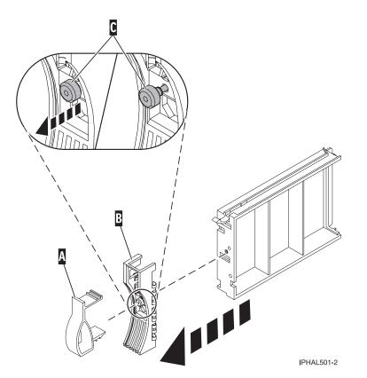
Figure 6. Removing the disk-drive bezel
