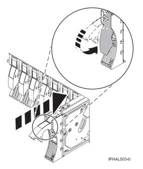
Figure 15. Installing a disk drive in a model
