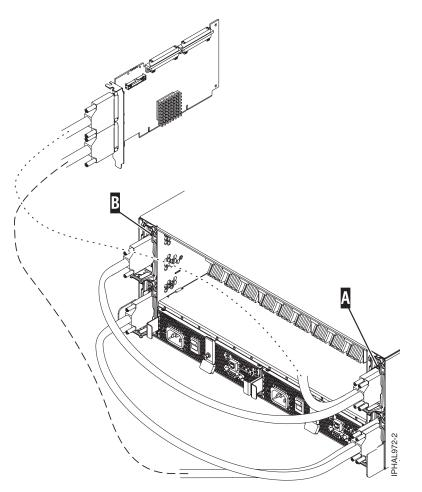
Figure 71. SCSI cable to dual repeater card connected to single repeater card
