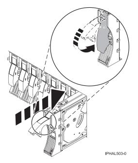
Figure 4. Installing a disk drive in a model
