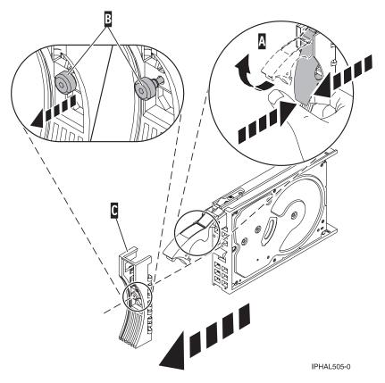
Figure 50. Removing a disk-drive bezel
