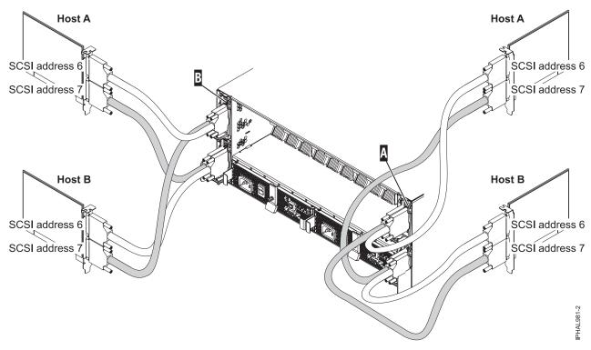
Figure 70. SCSI cable to dual repeater card connected with four SCSI cards
