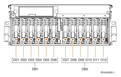
Figure 58. Disk drive locations for the 11D/20 expansion unit
