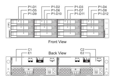
Figure 60. Disk drive locations for the 58/86 disk enclosure
