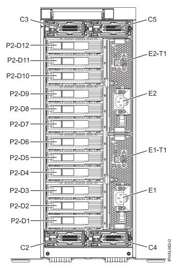
Figure 74. Repeater card location of the and 31T/24 SCSI disk-drive enclosure (stand-alone models)
