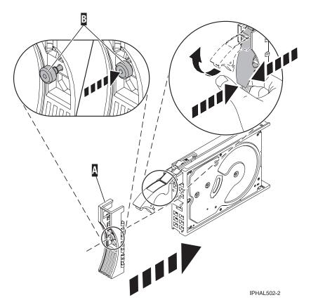
Figure 19. Installing a disk-drive bezel
