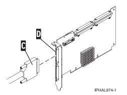
Figure 72. SCSI cable to SCSI interface card
