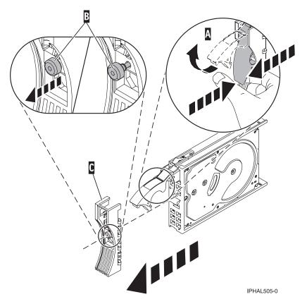
Figure 22. Removing a disk-drive bezel
