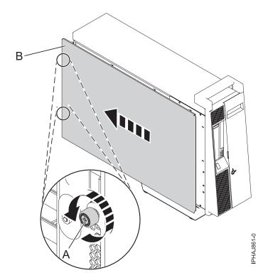
Figure 98. Removing the service access cover from the stand-alone model
