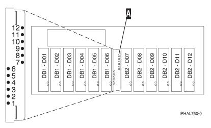
Figure 79. Model 11D/20 disk-drive concurrent maintenance lights
