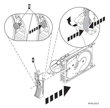
Figure 51. Attaching a disk-drive bezel
