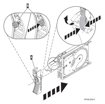
Figure 23. Installing a disk-drive bezel
