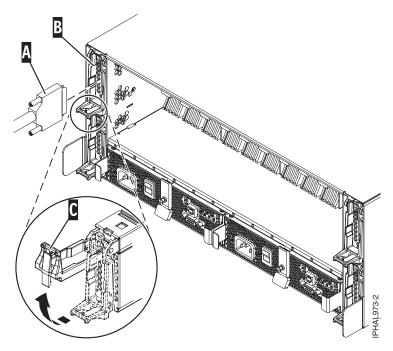
Figure 68. SCSI cable to single repeater card
