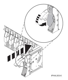
Figure 52. Installing a disk drive in a model a model or 11D/20
