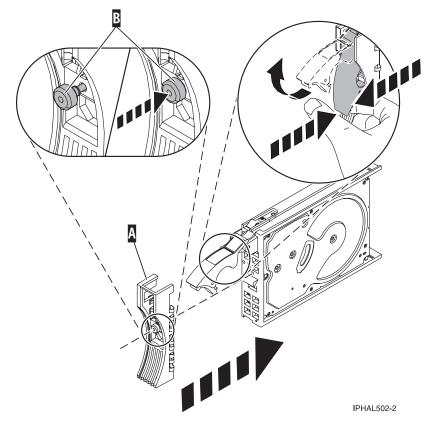
Figure 14. Attaching the disk-drive bezel to the disk drive.
