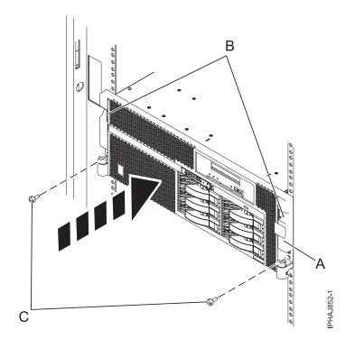
Figure 101. Installing the front cover on a rack-mounted model
