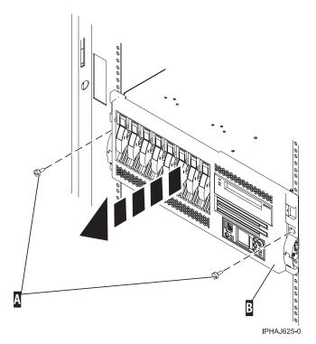
Figure 106. Removing the thumbscrews from the system and rack
