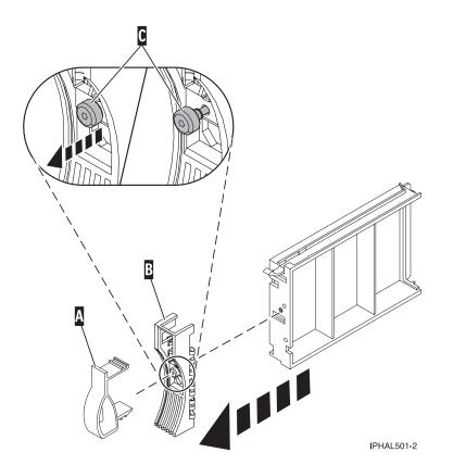
Figure 13. Removing a disk-drive bezel from the disk drive.
