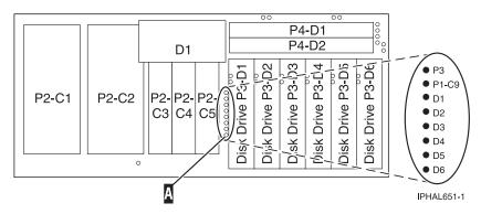
Figure 78. Model disk-drive concurrent maintenance lights
