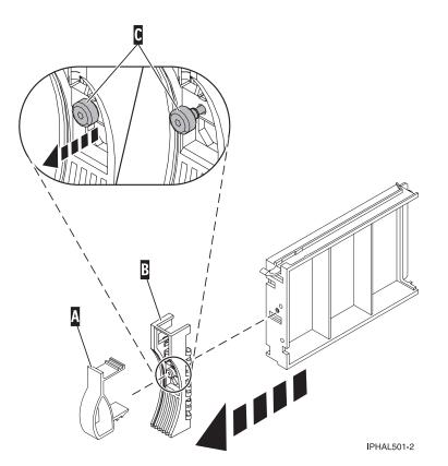
Figure 54. Removing a disk-drive bezel
