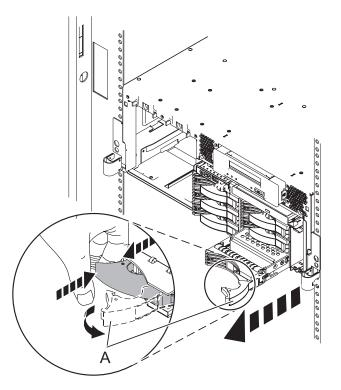
11. Remove the media device by pressing in on the latch **A** and sliding the media device out of the system, as shown in the following figure.
