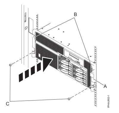
Figure 112. Replacing the thumbscrews
