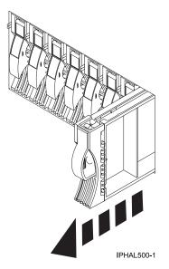
Figure 5. Removing a disk-drive filler from model
