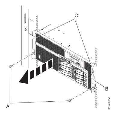
Figure 100. Removing the front cover from a rack-mounted model
