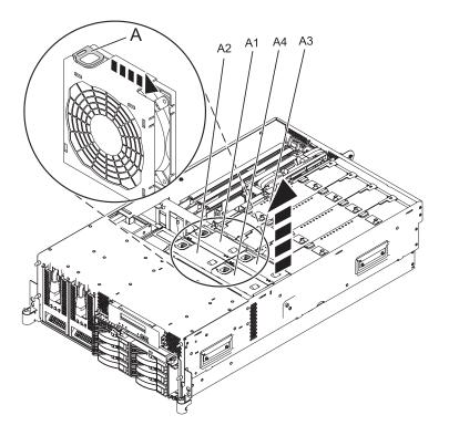
b. Remove the air flow cover **B** by lifting each of the four tabs **A** to release the cover, and lift the cover from the system, as shown in the following figure.
