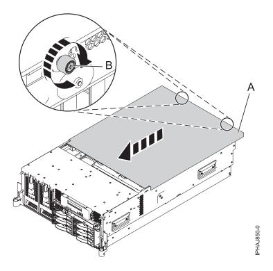
Figure 97. Install the service access cover on the rack-mounted model
