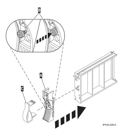
Figure 55. Attaching a bezel to a disk-drive filler
