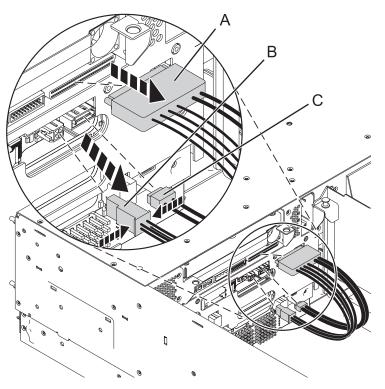
10. Remove the disk drives from the backplane if you need to replace the backplane because of an upgrade or system failure.
