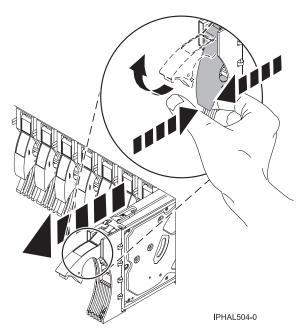
Figure 21. Removing a disk drive from a model
