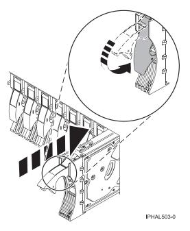
Figure 35. Installing a disk drive in a model or 11D/20
