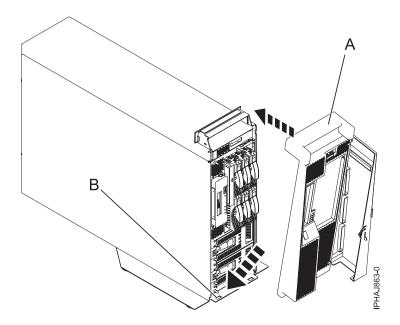
Figure 103. Replacing the cover on the model
