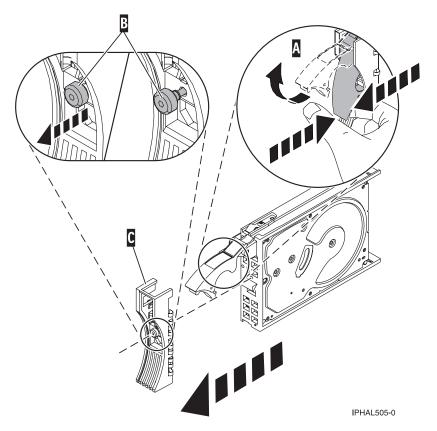
Figure 31. Removing a disk-drive bezel
