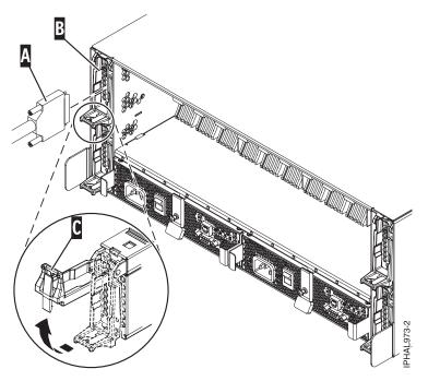
Figure 63. SCSI cable to single repeater card
