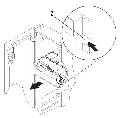
Figure 95. Removing the front cover
