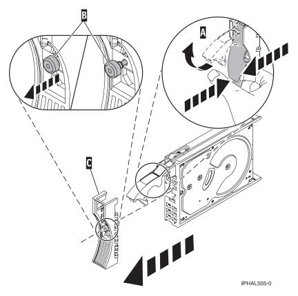
Figure 46. Removing a disk-drive bezel
