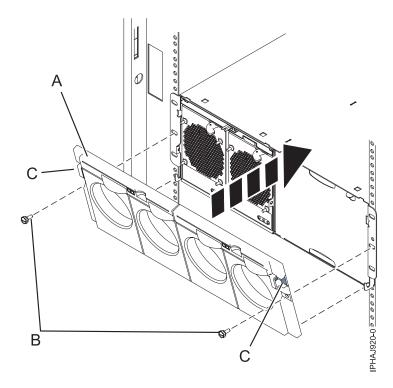
Figure 13. Front cover on a model 14G/30
