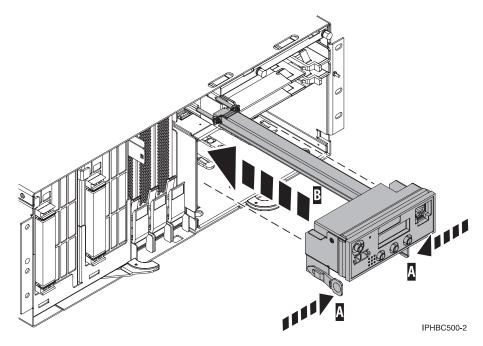
Figure 4. Control panel replacement
