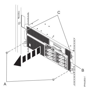
Figure 19. Removing the front cover from a rack-mounted model
