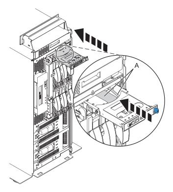
Figure 8. Control panel replacement in a stand-alone system unit
