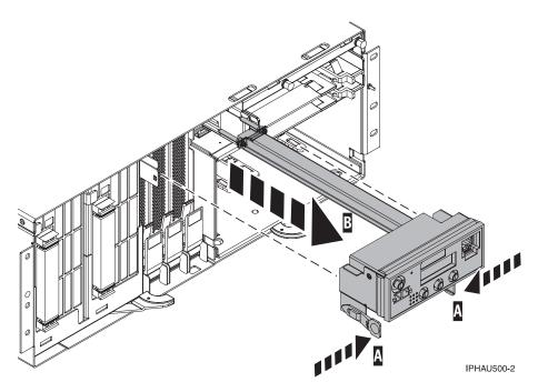
Figure 3. Control panel removal
