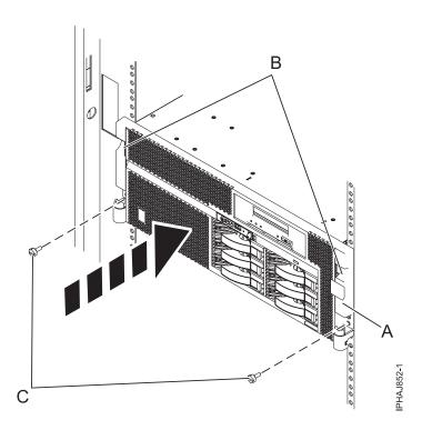
Figure 31. Replacing the thumbscrews
