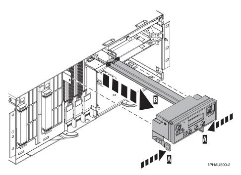
Figure 1. Control panel removal
