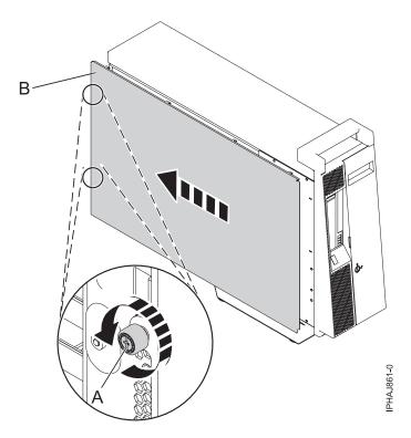
Figure 17. Removing the service access cover from the stand-alone model
