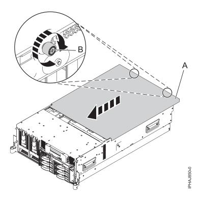
Figure 16. Install the service access cover on the rack-mounted model
