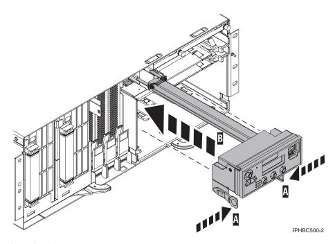
Figure 2. Control panel replacement
