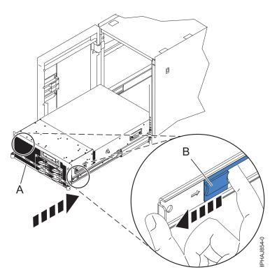
Figure 30. Releasing the rail safety latches
