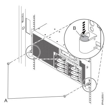
Figure 29. Releasing the rack latches
