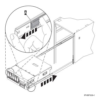
Figure 27. Releasing the rail safety latches
