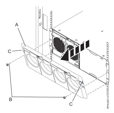
Figure 12. Remove the front cover for model 14G/30
