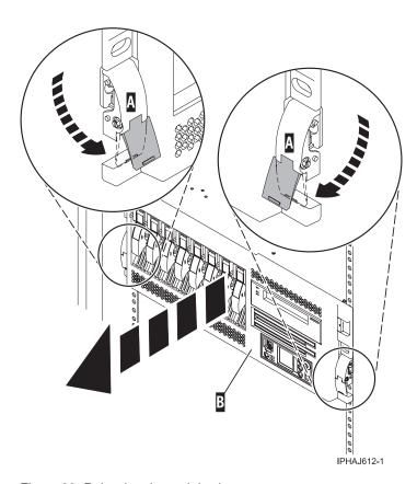
Figure 26. Releasing the rack latches
