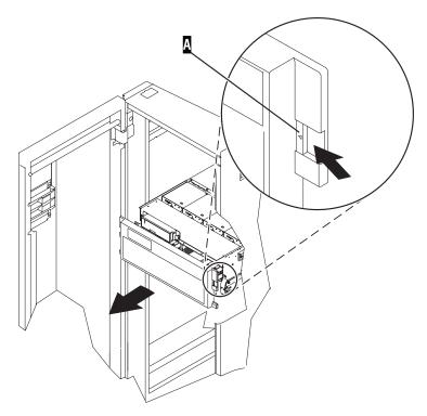
Figure 14. Removing the front cover
