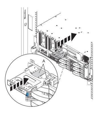
Figure 7. Control panel replacement in a rack-mounted system unit
