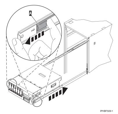
Figure 29. Releasing the rail safety latches
