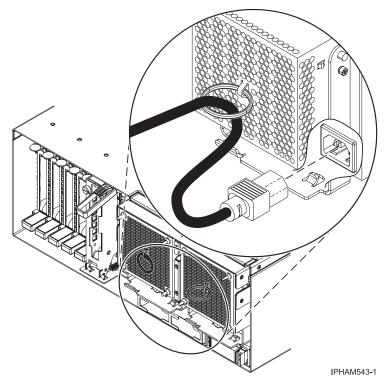
Figure 5. Cable routed through power supply ring
