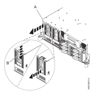
Figure 7. Removing the power supply
