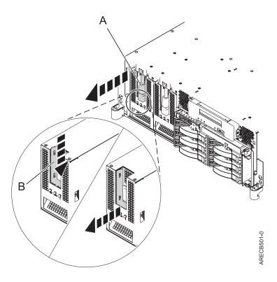
Figure 6. Removing power supply from rack-mounted model
