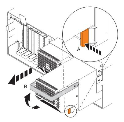
Figure 1. Power supply unlocked
