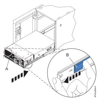
Figure 32. Releasing the rail safety latches
