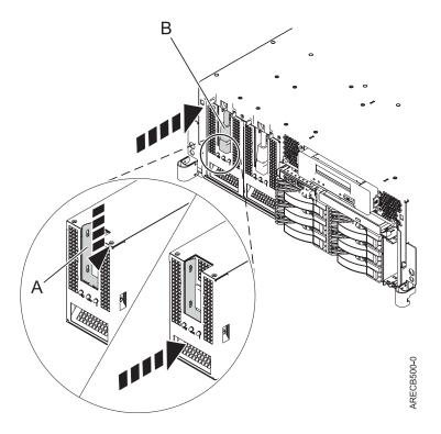
Figure 9. Replacing a power supply
