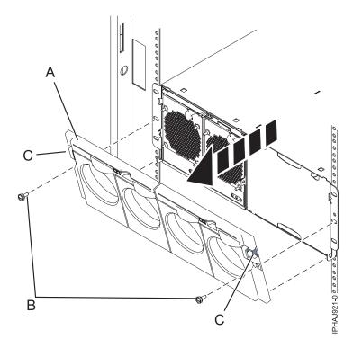
Figure 14. Remove the front cover for model 14G/30
