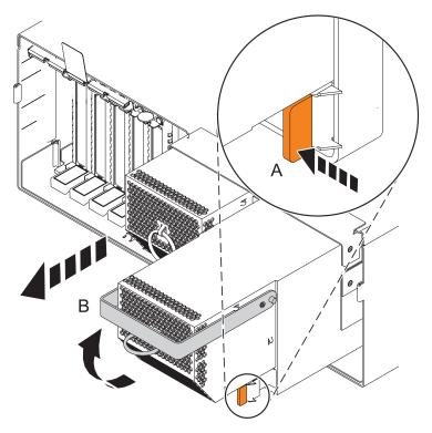
Figure 2. Power supply unlocked
