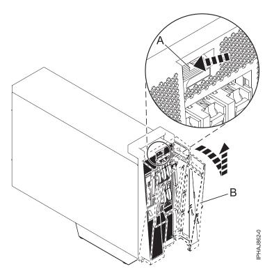
Figure 23. Remove the door from the model
