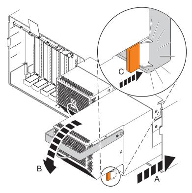
Figure 3. Replacing a power supply
