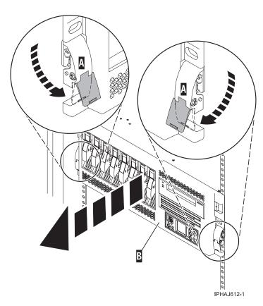
Figure 28. Releasing the rack latches
