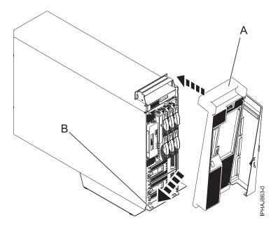
Figure 24. Replacing the cover on the model
