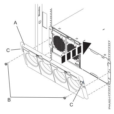
Figure 15. Front cover on a model 14G/30
