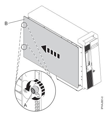
Figure 19. Removing the service access cover from the stand-alone model
