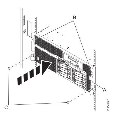
Figure 33. Replacing the thumbscrews
