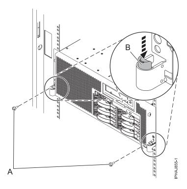
Figure 31. Releasing the rack latches
