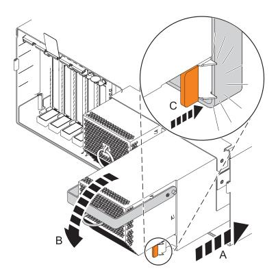
Figure 4. Replacing the power supply
