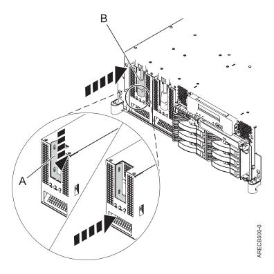
Figure 10. Replacing a power supply
