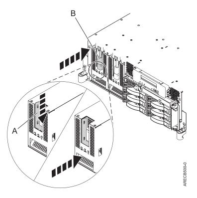
Figure 8. Replacing a power supply
