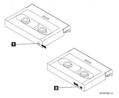
When the switch is set to the right, data can be written to and read from the tape
