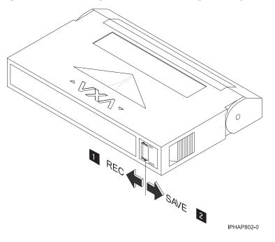
When the switch is set to the left, data can be written to and read from the tape.
