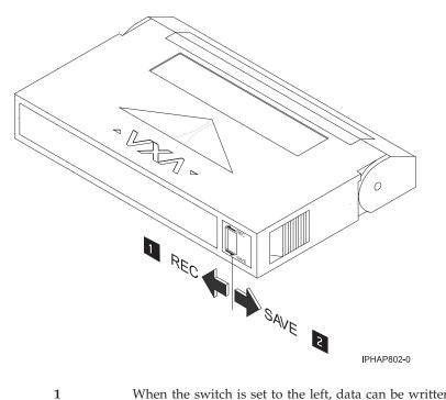
When the switch is set to the left, data can be written to and read from the tape. When the switch is set to the right, data can only be read.
