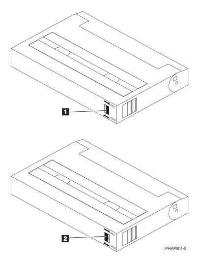
When the switch is set to the left in the SAVE position 1, data cannot be written to or read from the tape (data is saved).
