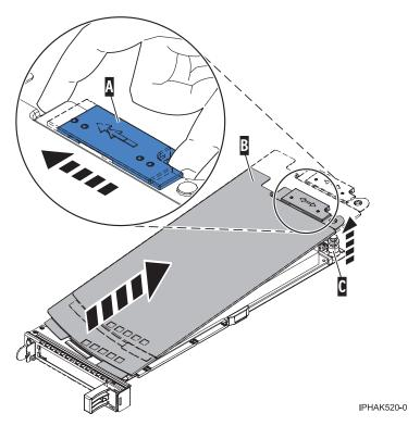
Figure 6. PCI adapter cassette cover removed
