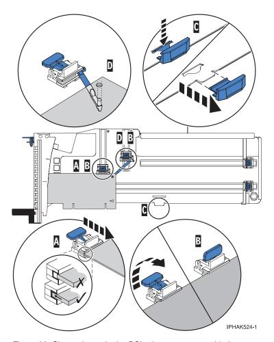
Figure 23. Short adapter in the PCI adapter cassette with the supports and the hookarm in place
