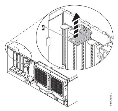
Figure 3. Lift up on the EMC shield
