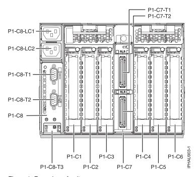
Figure 1. Rear view of unit.
