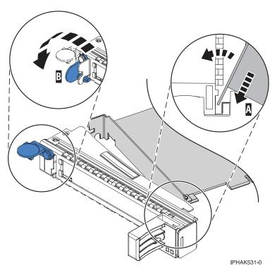
Figure 32. Adapter removed from the PCI adapter single-width cassette
