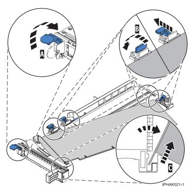
Figure 7. Adapter removed from the PCI adapter cassette
