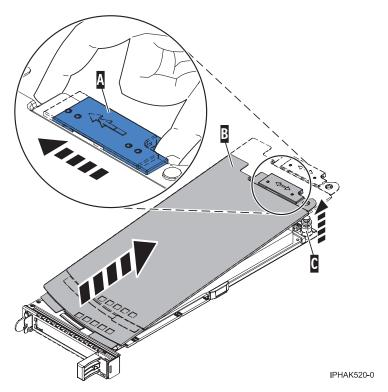
Figure 30. PCI adapter cassette cover removed
