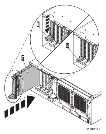
Figure 13. PCI adapter cassette removed from the system unit
