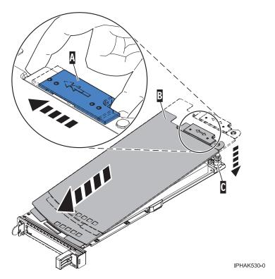
Figure 12. PCI adapter cassette cover replaced
