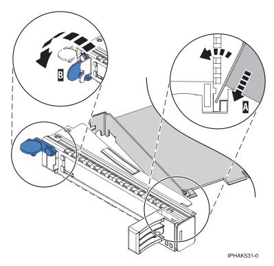
Figure 8. Adapter removed from the PCI adapter single-width cassette
