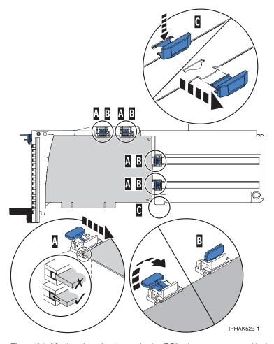
Figure 34. Medium-length adapter in the PCI adapter cassette with the supports in place
