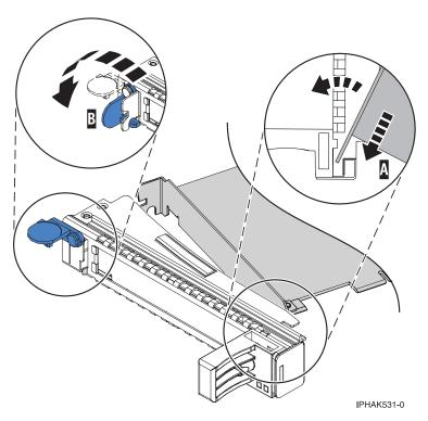
Figure 20. Adapter removed from the PCI adapter single-width cassette
