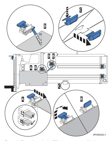
Figure 11. Short adapter in the PCI adapter cassette with the supports and the hookarm in place
