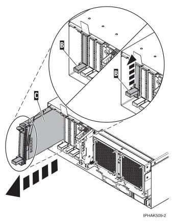
Figure 5. PCI adapter cassette removed from the system unit
