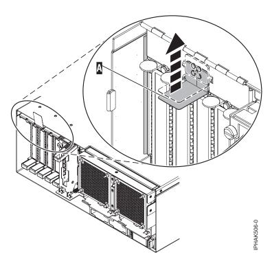
Figure 27. Lift up on the EMC shield
