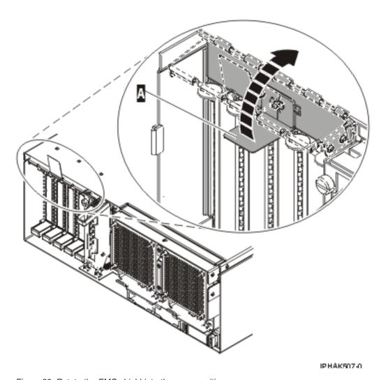
Figure 28. Rotate the EMC shield into the open position
