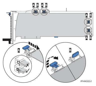
Figure 21. Long adapter in the PCI adapter cassette with the supports and stabilizer in place
