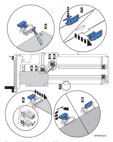
Figure 35. Short adapter in the PCI adapter cassette with the supports and the hook arm in place
