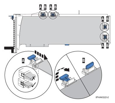
Figure 9. Long adapter in the PCI adapter cassette with the supports and stabilizer in place
