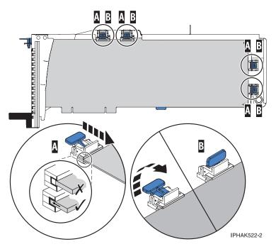
Figure 33. Long adapter in the PCI adapter cassette with the supports and stabilizer in place
