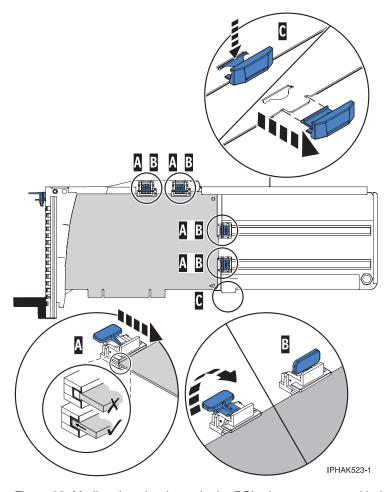
Figure 22. Medium-length adapter in the PCI adapter cassette with the supports in place
