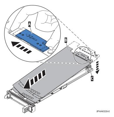
Figure 24. PCI adapter cassette cover replaced
