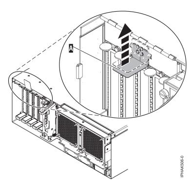
Figure 15. Lift up on the EMC shield
