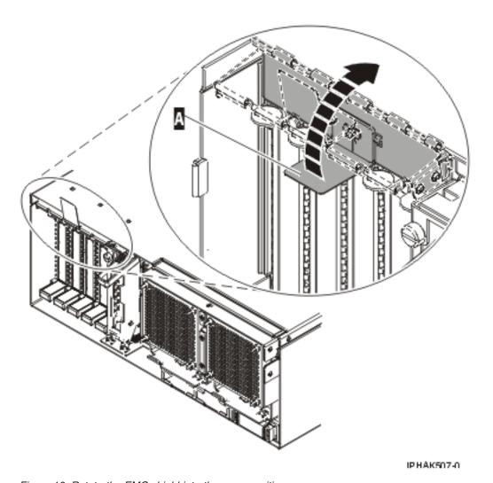
Figure 16. Rotate the EMC shield into the open position
