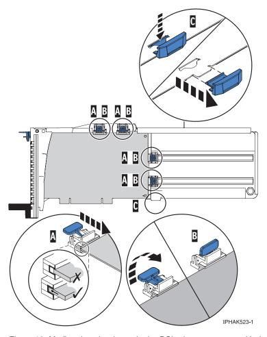
Figure 10. Medium-length adapter in the PCI adapter cassette with the supports in place
