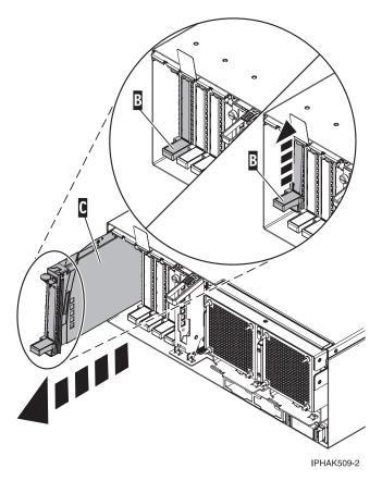
Figure 17. PCI adapter cassette removed from the system unit
