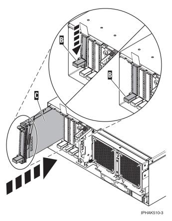
Figure 25. PCI adapter cassette removed from the system unit
