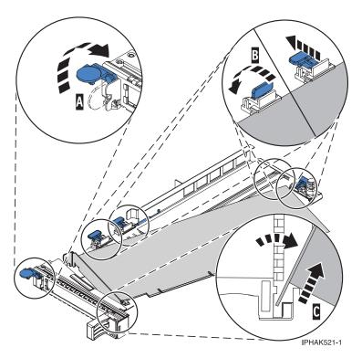
Figure 31. Adapter removed from the PCI adapter cassette
