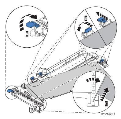
Figure 19. Adapter removed from the PCI adapter cassette
