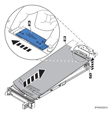
Figure 18. PCI adapter cassette cover removed
