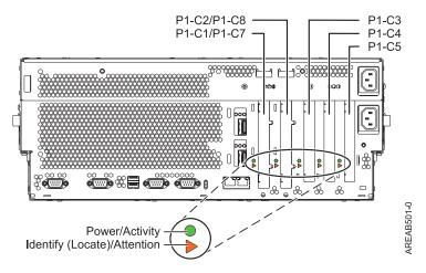
Figure 3. Back view of enclosure with location codes
