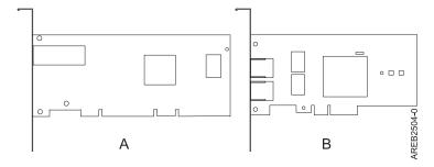
Figure 1. PCI-X adapter and PCIe 4x adapter
