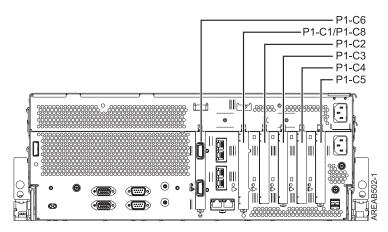
Figure 2. Back view of enclosure with location codes
