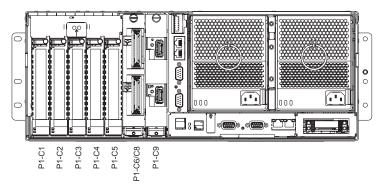
Figure 4. Back view of enclosure with location codes.
