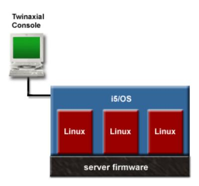
This figure illustrates the IBM i logical partition and the Linux logical partitions that are managed by the IBM i logical partition. The user creates and configures the Linux logical partitions on the server by accessing SST over the twinaxial console.
