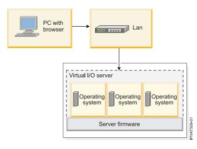
This figure illustrates an IBM Power Systems server or an IBM BladeCenter blade server with POWER<sup>®</sup> Architecture technology. The Virtual I/O Server is in its own logical partition, and the client logical partitions are managed by the Virtual I/O Server logical partition. The browser on the PC connects to the Integrated Virtualization Manager interface over a network, and you can use the Integrated Virtualization Manager to create and manage the logical partitions on the server.
