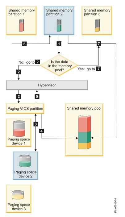
Figure 3. The process of managing data in a shared memory configuration that is overcommitted
