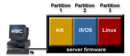
In this figure, you can see the logical partitions and the server firmware on the server. The *server firmware* is code that is stored in system flash memory on the server. The server firmware directly controls the resource allocations on the server and the communications between logical partitions on the server. The HMC connects with the server firmware and specifies how the server firmware allocates resources to the managed system.
