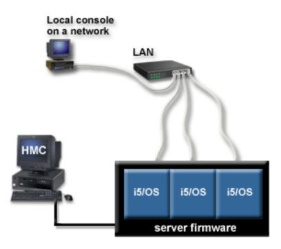
The following figure shows a partitioned IBM System i model with an HMC and local consoles directly attached to the server.
