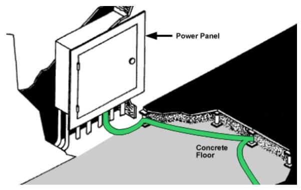
Figure 10. Transient grounding using the raised floor support structure
