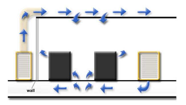
Figure 22. Combination overhead and underfloor air conditioning system
