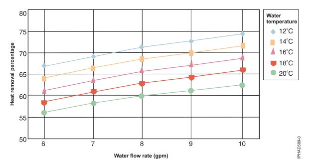
*Figure 26. Typical performance of a rear door heat exchanger, 32 kW heat load.* Percentage heat removal as function of water temperature and flow rate. (24°C rack inlet air, 32 kW rack load, 1530 cfm air through the rear door heat exchanger)
