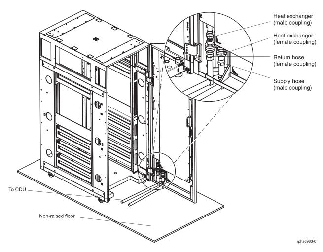
Figure 44. Non-raised floor hose requirements 24-inch EIA-rail rack
