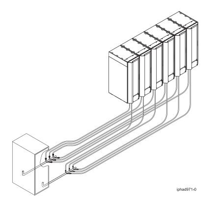
*Figure 33. Typical central manifold (located at a central location for multiple water circuits)* The following figure shows an extended manifold layout.
