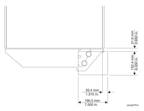
Figure 38. Raised floor hose management example 1; Tile cut out definition and location for 24-inch EIA-rail racks
