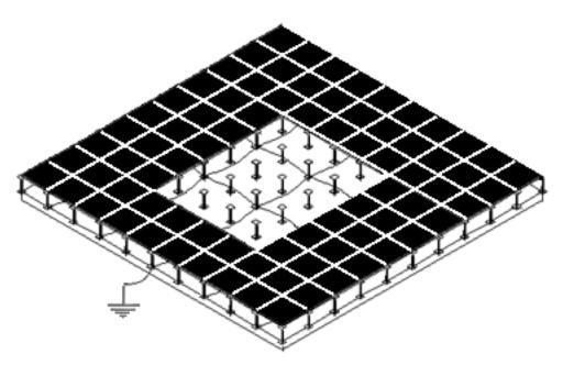
Figure 11. Signal reference grid
