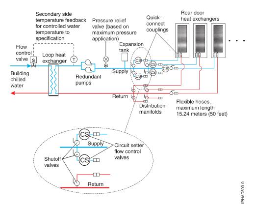
Figure 28. Coolant distribution using a fabricated facilities solution
