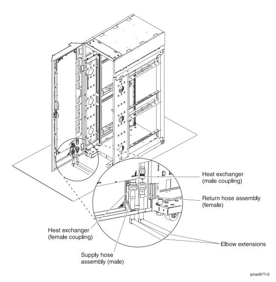
Figure 43. Non-raised floor hose requirements for 19-inch EIA-rail rack
