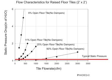
Figure 19. Volumetric flow capabilities of various raised floor tiles
