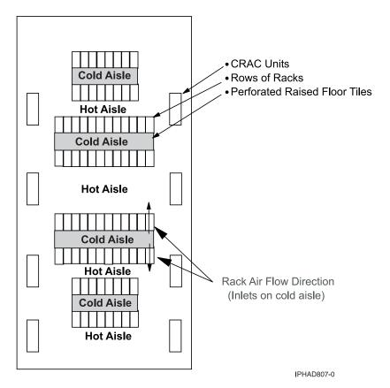
Figure 16. Hot aisle and cold aisle arrangement
