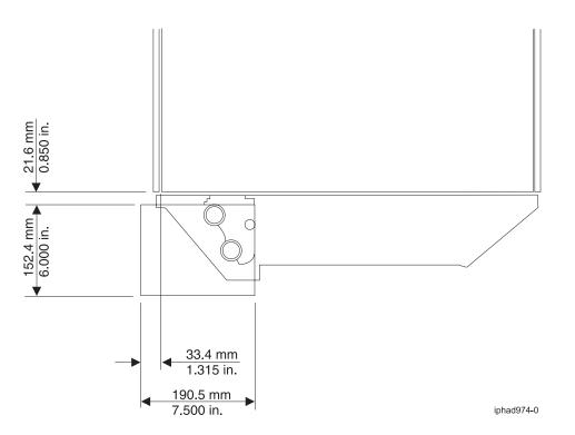
Figure 37. Raised floor hose management example 1; Tile cut out definition and location for 19-inch EIA-rail racks
