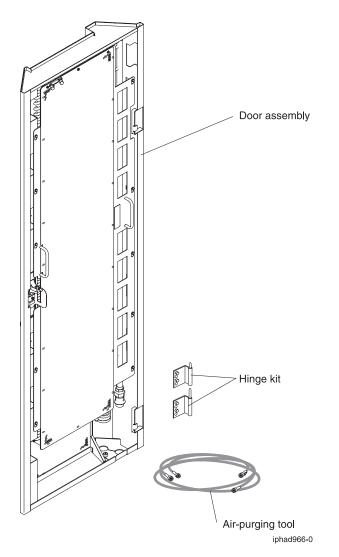
Figure 24. Components of the heat exchanger kit for 19-inch EIA-rail racks
