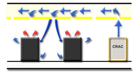
Figure 23. Overhead air distribution system
