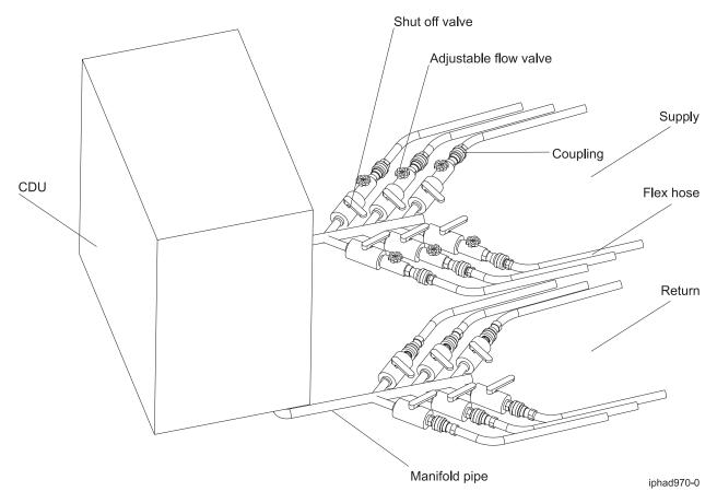
Figure 32. Typical central distribution manifold layout in a central location
