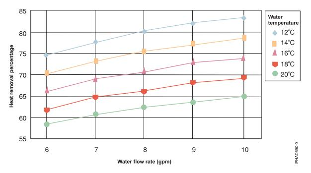
*Figure 27. Typical performance of a rear door heat exchanger, 20 kW heat load.* Percentage heat removal as function of water temperature and flow rate. (24°C rack inlet air, 20 kW rack load, 1530 cfm air through the rear door heat exchanger)
