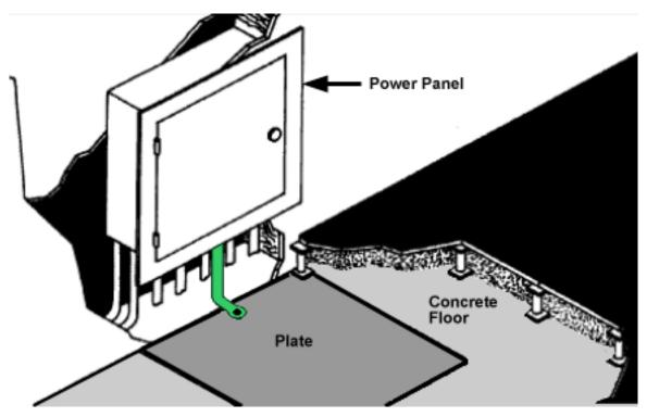
Figure 9. Transient grounding plate
