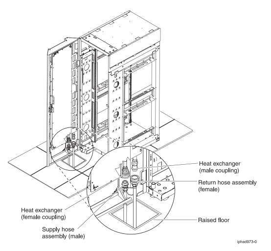
Figure 35. Raised floor hose management example 1; tile cut out size and position for 19-inch EIA-rail racks.
