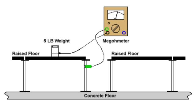
Figure 1. Typical test connection to measure floor conductivity
