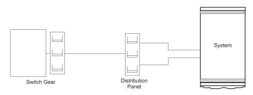
Figure 14. Single distribution panel - Dual circuit breakers
