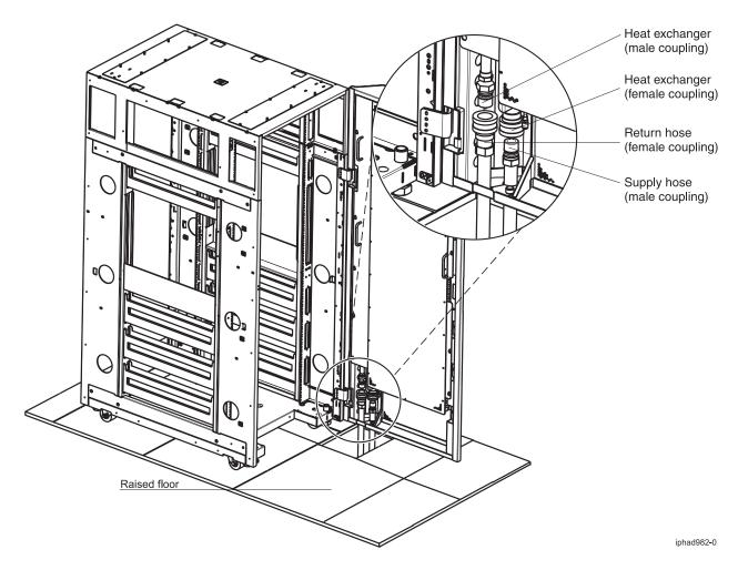
Figure 36. Raised floor hose management example 1; tile cut out size and position for 24-inch EIA-rail racks.
