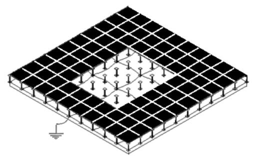
Figure 3. Signal reference ground
