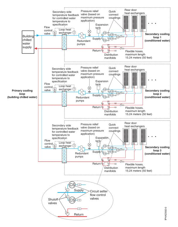
Figure 31. Primary and secondary cooling loops
