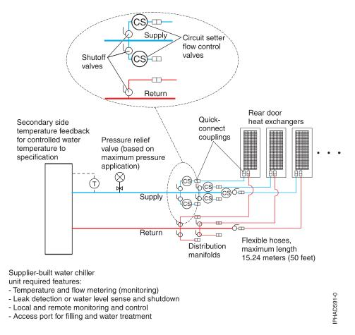
Figure 30. Cooling distribution unit that uses a water chiller unit to provide conditioned water
