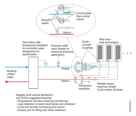
Figure 29. Coolant distribution using off-the-shelf supplier solutions
