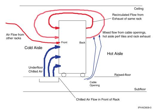
Figure 17. Possible rack airflow patterns
