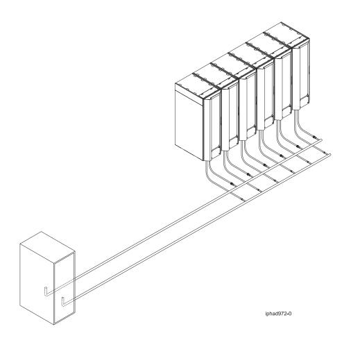
Figure 34. Typical extended manifold (located along aisles between racks)
