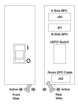
The preceding figure illustrates the back of the machine UEPO panel with the room EPO cable plugging into the machine. After the switch actuator is moved to make the cable connection possible, the room EPO cable must be installed for the machine to power on.
