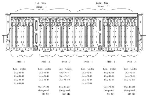
I/O Subsystem Rear View with Numbered Slots
