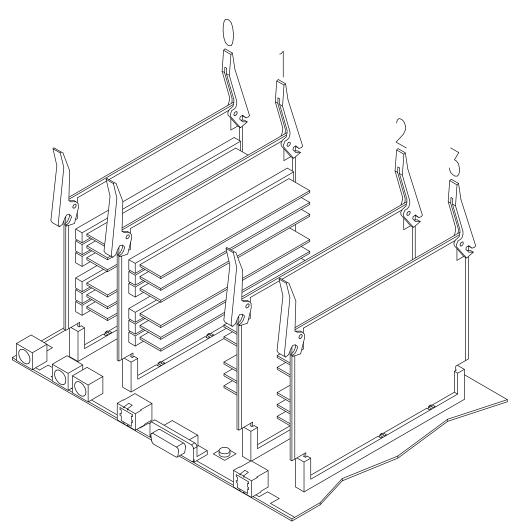
1. Open outward the two hooked clips of the memory riser.
