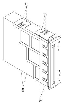
8. Align the device in the designated slot and then slide it inside the system. Secure then the media tightening the corresponding screws.
