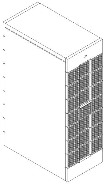
The rack is equipped with a front door which allows the access to the operator controls of the installed drawers and a rear door which allows the access to the back of the drawers for their maintenance.
