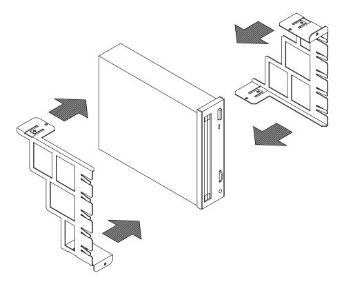
7. Secure the mounting kit tightening the screws.
