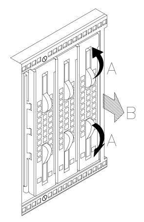
5. Unscrew the mounting screws provided with each installed disk carrier.
