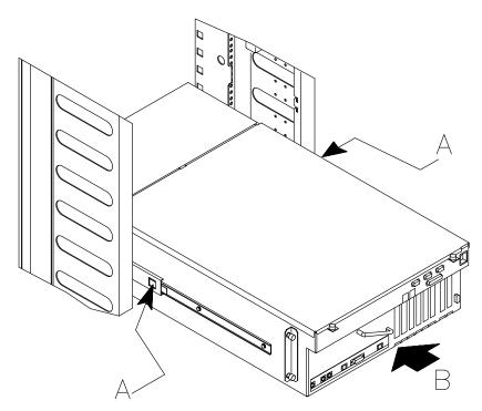
2. Accessing the drawer from the rear, tighten the retaining screws, securing the drawer to the chassis.
