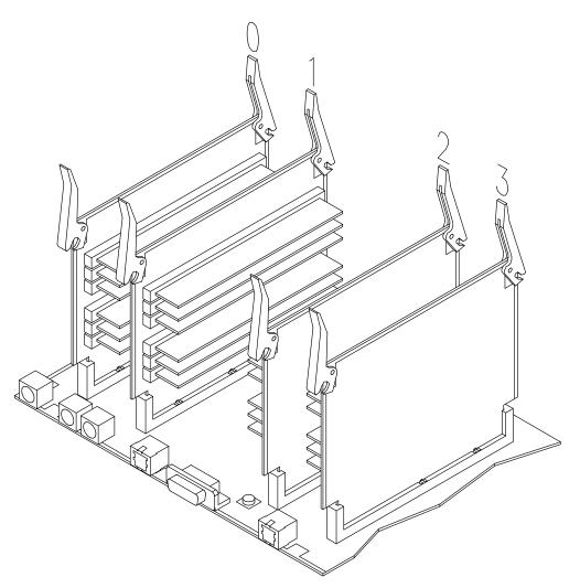
1. Open outward the two hooked clips of one memory riser.
