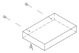
11. Store the removed device in an antistatic envelope.
