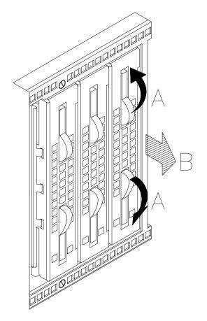
5. Grip the metal support of the light ducts and pull it out of the disk carrier.
