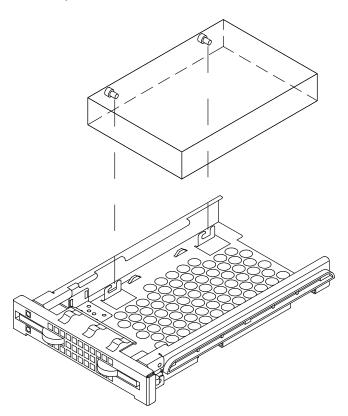
10.Lightly push the drive towards the front side of the disk carrier to seat the screws in the locking brackets (A). Secure the hard disk drive by tightening first the screws on the right side (B) and then the screws on the left side of the disk carrier (C).
