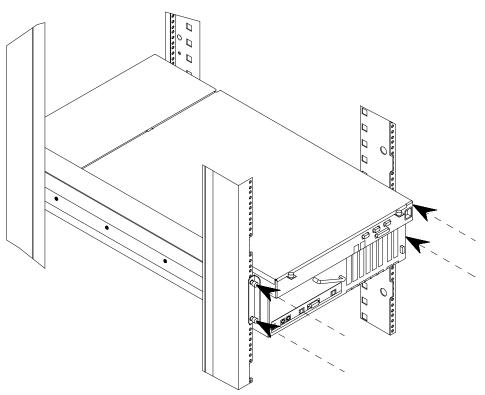
2. Using the handle at the rear of the drawer, slide the drawer out until it is well locked.
