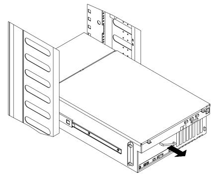
**Note:** In case cables connected to the drawer make the drawer sliding operation difficult, record which connector attaches to which cable and disconnect the cables.
