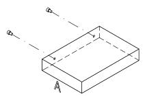
9. Slide the hard disk drive into the disk carrier making sure that the screw threads fit into the locking brackets of the disk carrier. The SCSI connector of the hard disk drive must be kept towards the rear of the disk carrier.
