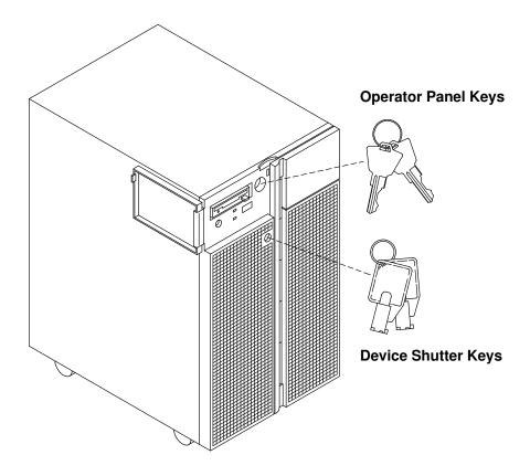
Put the device shutter keys in a safe place because these are not needed now. To go on with the system setup procedure you are required only to insert one of the operator panel keys in the key mode switch.
