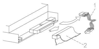
6. Pushing simultaneously the snaps at the sides of the media drive, slide it out from the slot.
