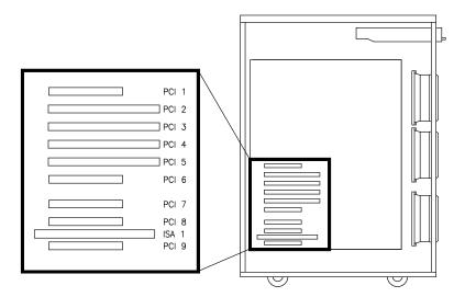
The system provides two native PCI local busses (PCI0, PCI1). PCI bus 0 generates an additional PCI bus through a PCI to PCI bridge (PCI0\_1). It also generates an ISA bus through a PCI to ISA bridge.
