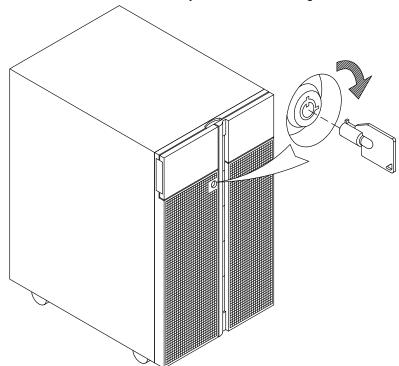
2. Open the device shutter of the front panel.
