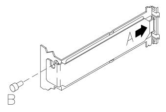
Warning: It is recommended to install a slot cover in any free controller card slot.
