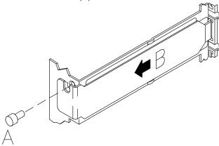
Warning: It is recommended to store the removed slot cover for possible re-installation.
