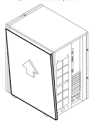
5. Lift the panel from the unit and remove it.
