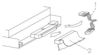
16. Remove the plastic blank on the front panel that corresponds to the slot in which you have just installed the media drive, by performing the following steps:
