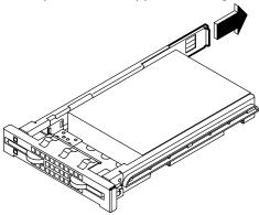
8. Unscrew the screws on the right side of the disk carrier and remove them.
