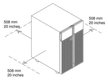
In addition, before installing the system, you should keep into consideration also the space that could be necessary on each side for possible service and maintenance.
