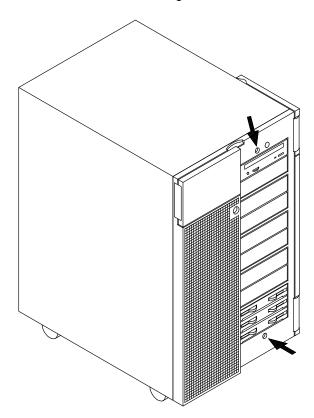
4. Close the device shutter, grip the front panel at the sides and slide it towards you.
