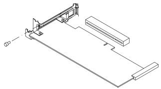
11. Connect any connector cable to the controller card just installed, if any.
