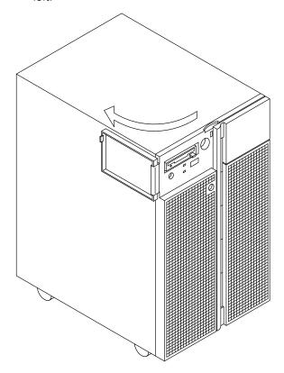
2. Insert the operator panel key in the key mode switch in the position shown in the figure.
