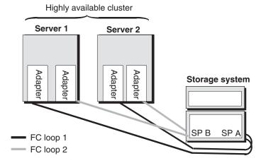
Either SP can control any LUN in the storage system, but only one SP at a time can control a LUN. If one SP cannot access a LUN it controlled (because of a failure), you can transfer control of the LUN to the other SP, manually or via software.
