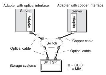
A switch is technically a repeater, not a node, in a Fibre Channel loop. However, it is bound by the same cabling distance rules as a node.
