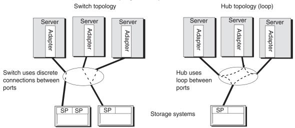
Fibre Channel switches are available with 16 or 8 ports. They are compact units that fit in 2 U (3.5 inches) for the 16-port or 1 U (1.75 inches) for the 8-port. They are available to fit into a rackmount cabinet or as small deskside enclosures.
