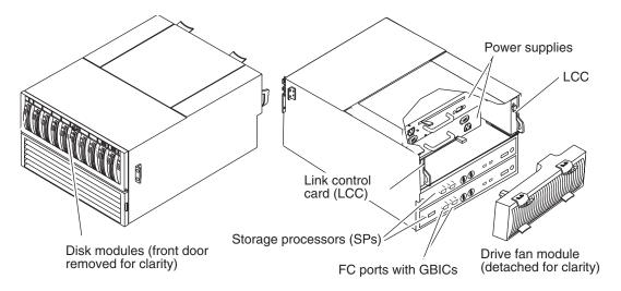
A separate standby power supply (SPS) is required to support write caching. All the shared storage components — rackmount DPE, DAEs, SPSs, and cabinet — are shown in the following figure.
