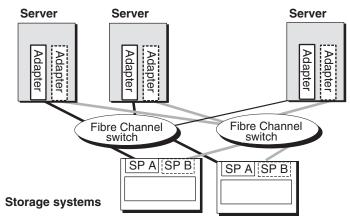
Fibre Channel switches can control data access to storage systems through the use of switch zoning. With zoning, an administrator can specify groups (called zones) of Fibre Channel devices (such as host-bus adapters, specified by worldwide name), and SPs between which the switch will allow communication.
