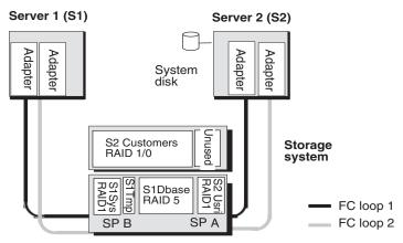
If each disk holds 18 Gbytes, then the storage-system chassis provides Server 1 with 108 Gbytes of disk storage, 90 Gbytes highly available; it provides Server 2 with 90 Gbytes of storage, all highly available. Each server has its own SP, which controls that server's LUNs; those LUNs remain primary to that server. The LUNs are as follows. The LUN capacities shown assume 18-Gbyte disks.
