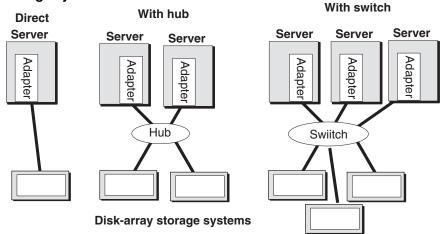
Depending on your server type, you may have a choice of adapters. The adapter is designed for a specific host bus; for example, a PCI bus or SBUS. Some adapter types support copper or optical cabling; some support copper cabling only.
