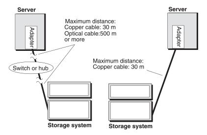
You can use any existing FDDI, multimode, 62.5 micron cable with good connections to attach servers, hubs, and storage systems. These cables must be dedicated to storage-system I/O.
