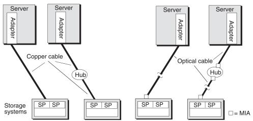
A hub is technically a repeater, not a node, in a Fibre Channel loop. However, it is bound by the same cabling distance rules as a node.
