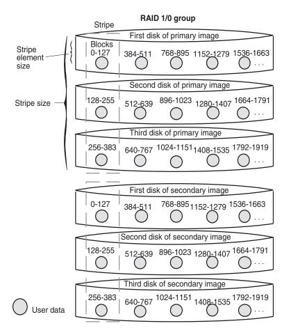
A RAID 1/0 group can survive the failure of multiple disks, providing that one disk in each image pair survives.
