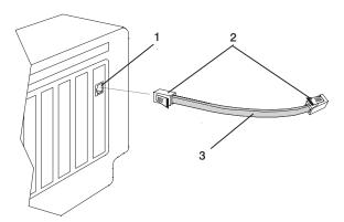
Figure 2. Connecting the Adapter to the Network
