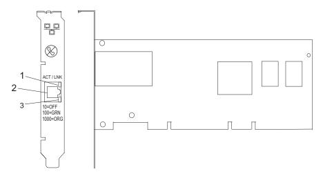
Figure 1. 10/100/1000 Base-TX Ethernet PCI-X Adapter
