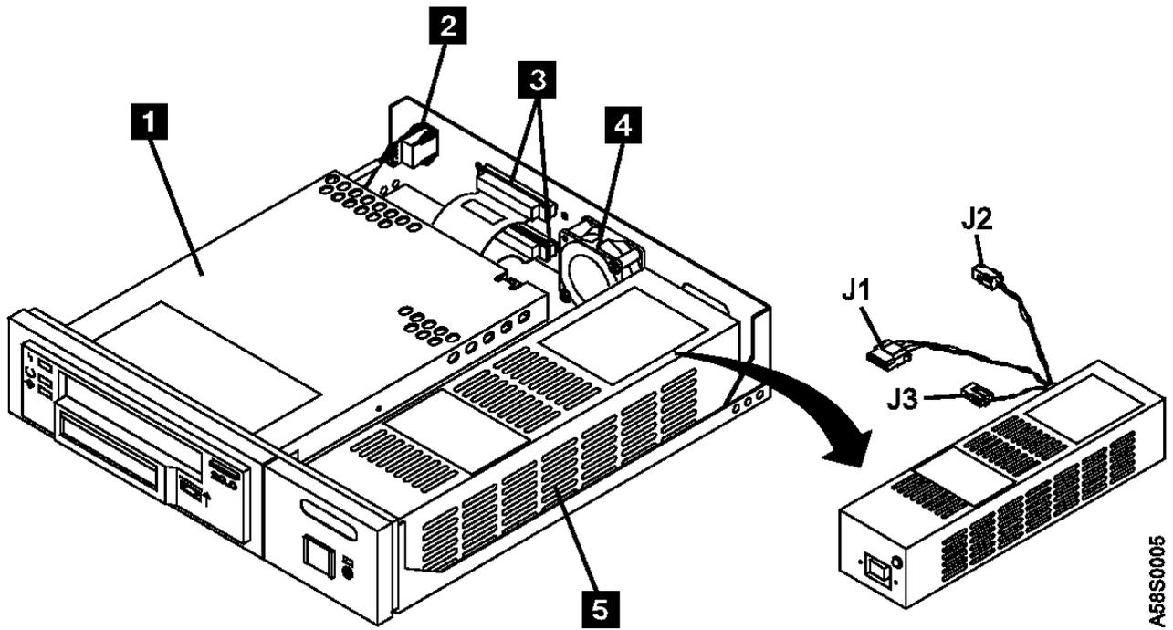
Figure 9. Internal View of the 7208 Tape Drive Model 342
