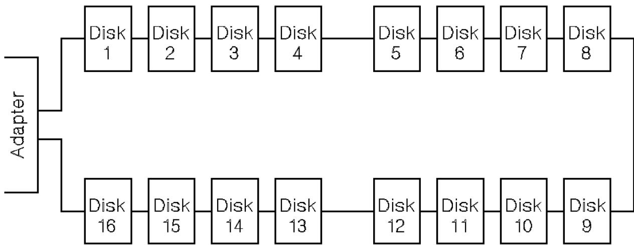
Figure 2-9. One Pair of Connectors in the Loop
