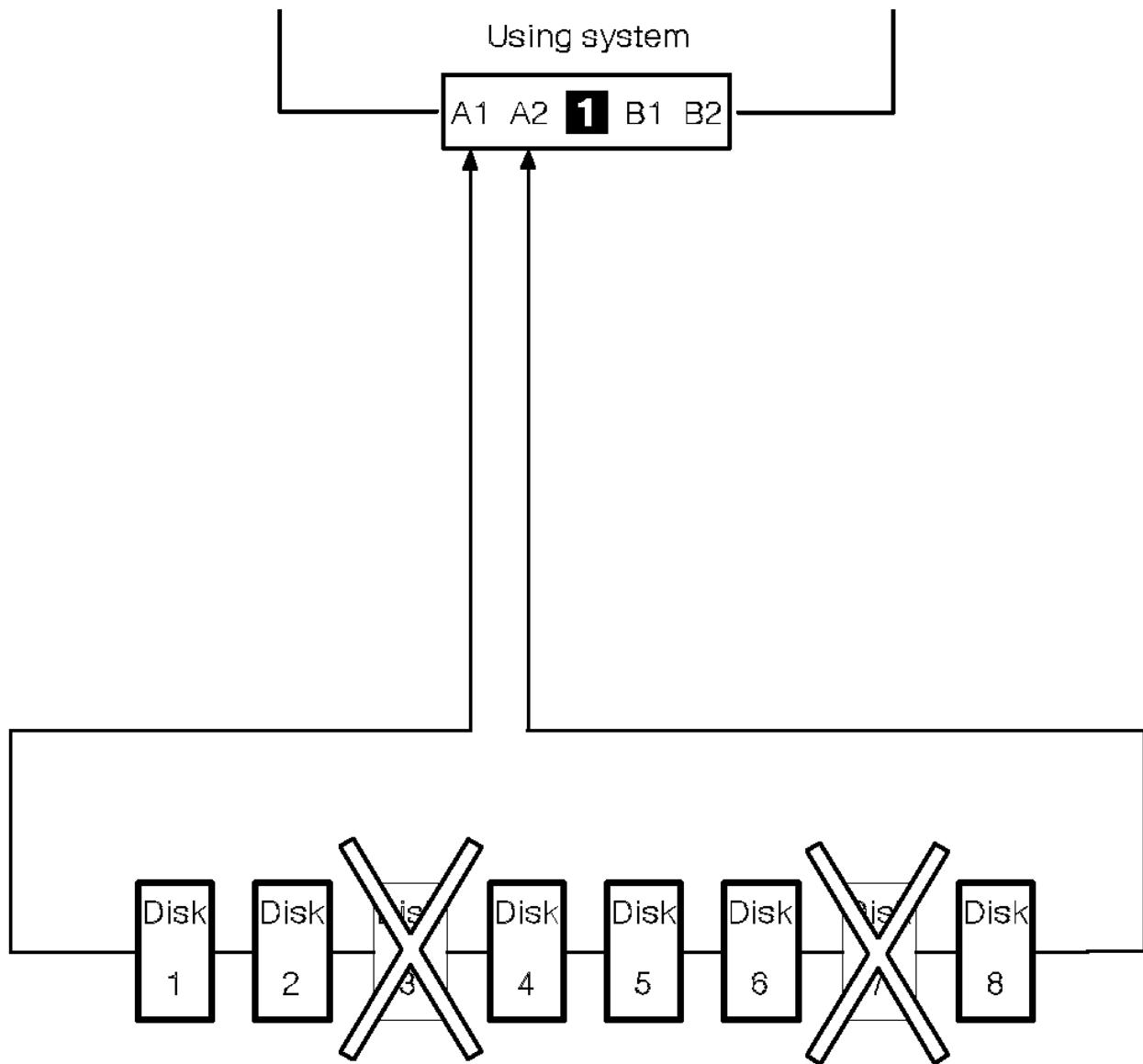
Figure 2-3. Simple Loop with Two Disk Drives Missing
