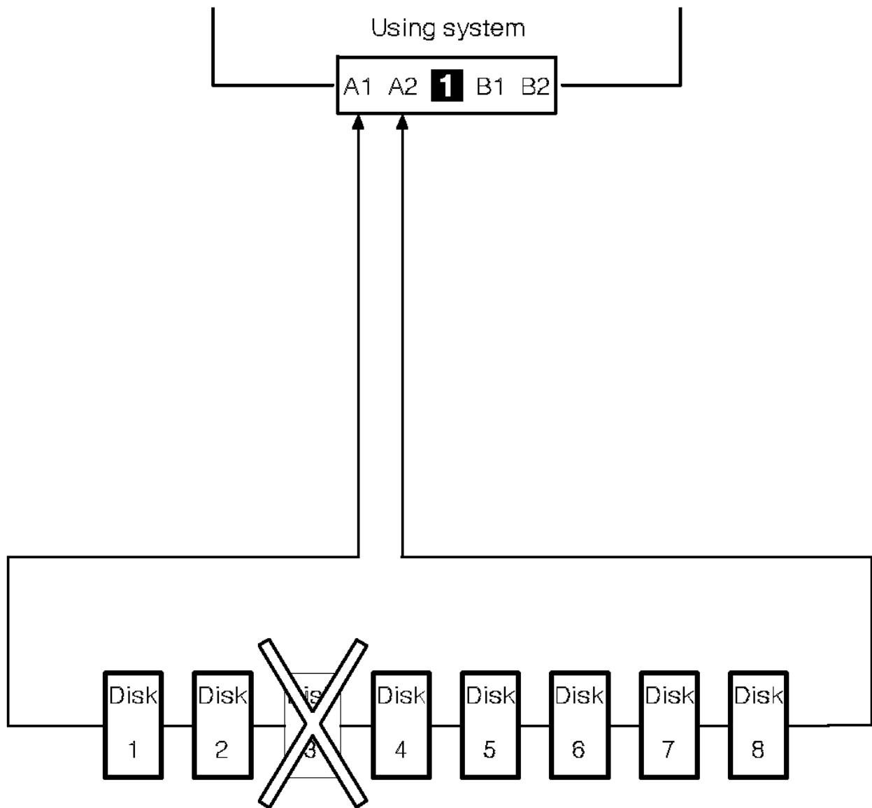
Figure 2-2. Simple Loop with One Disk Drive Missing
