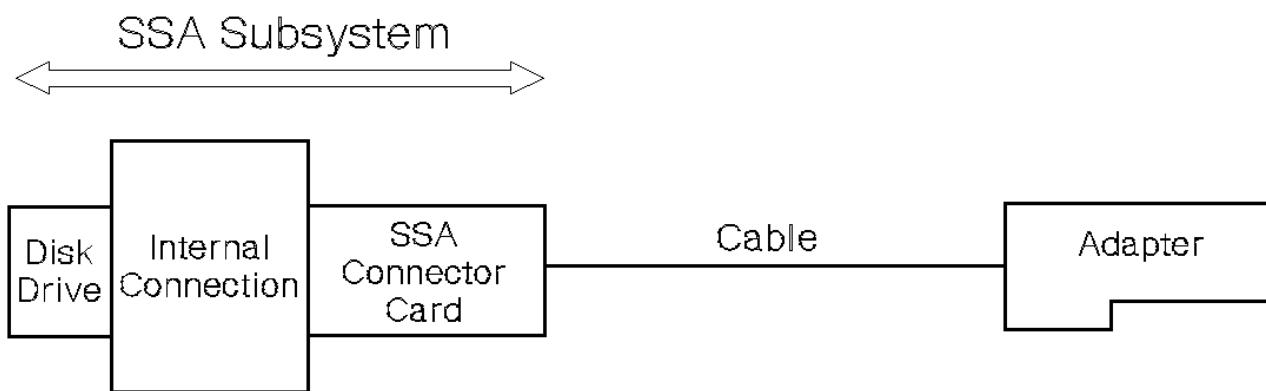
Figure 13-4. Five-Part Link between Disk Drive and Adapter
