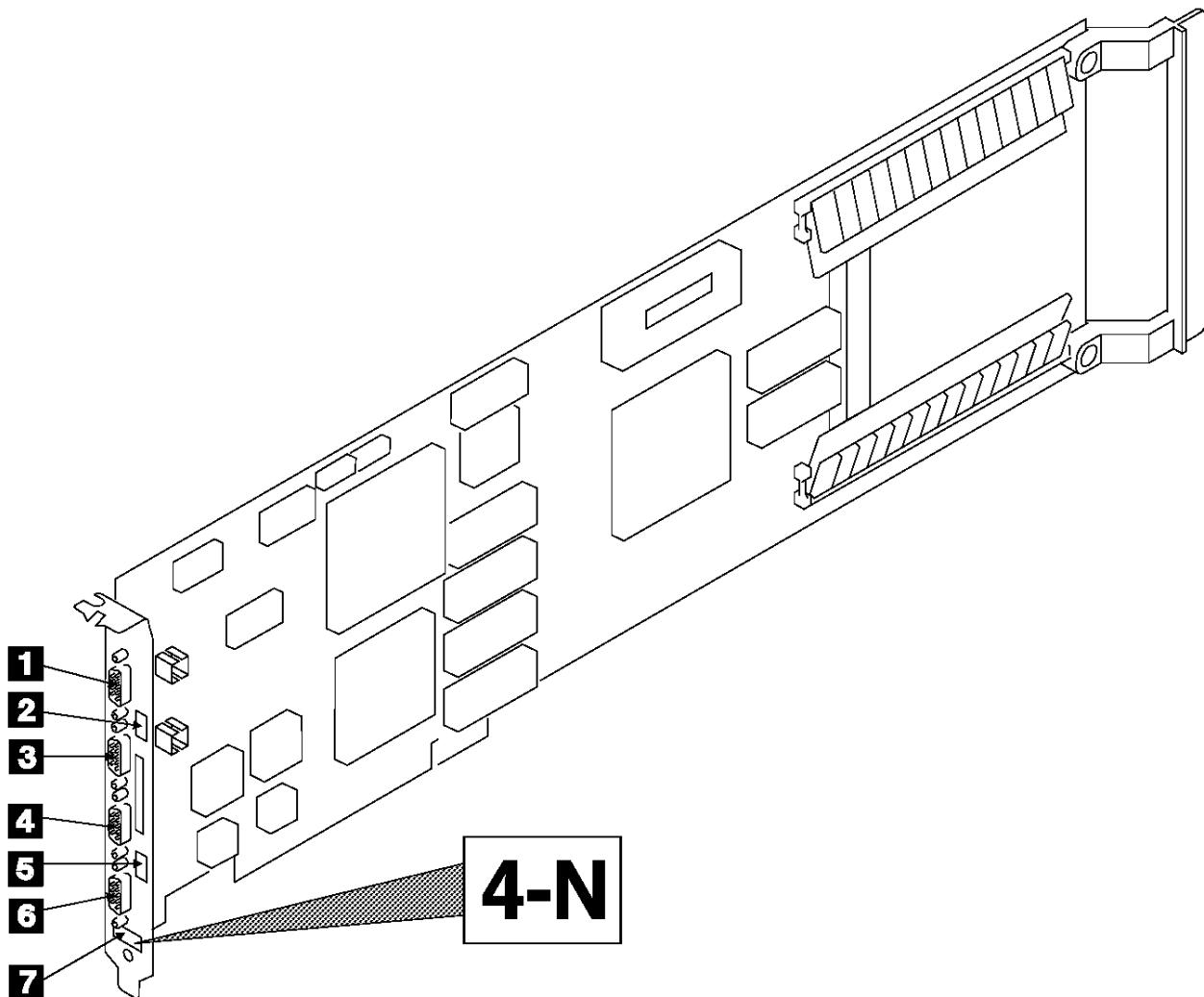
Figure 1-6. The PCI SSA Multi-Initiator/RAID EL Adapter Card (Type 4-N)
