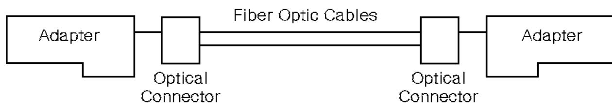
Figure 13-5. Five-Part Link between Two Adapters
