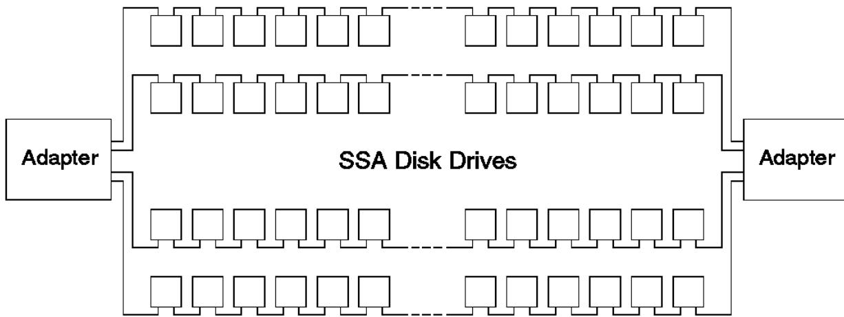
Figure 2-7. Two Loops with Two Adapters
