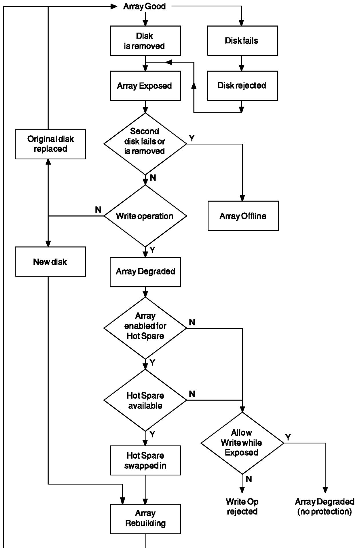
Figure 3-1. Array State Flowchart
