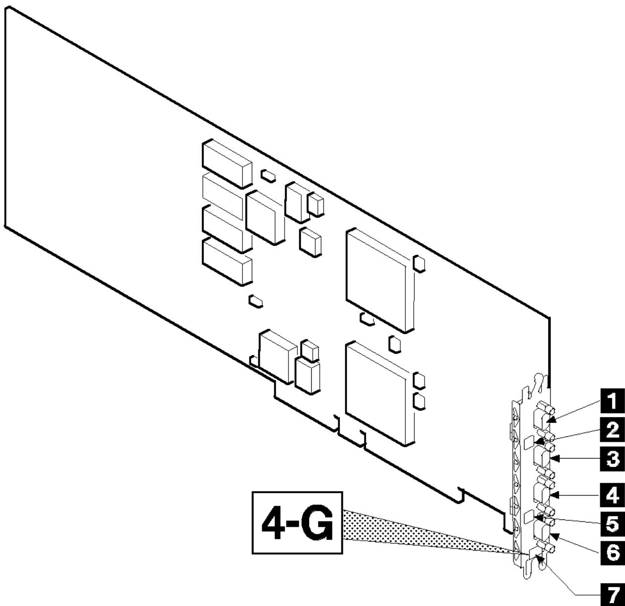
Figure 1-2. The Enhanced SSA 4-Port Adapter Card (Type 4-G)
