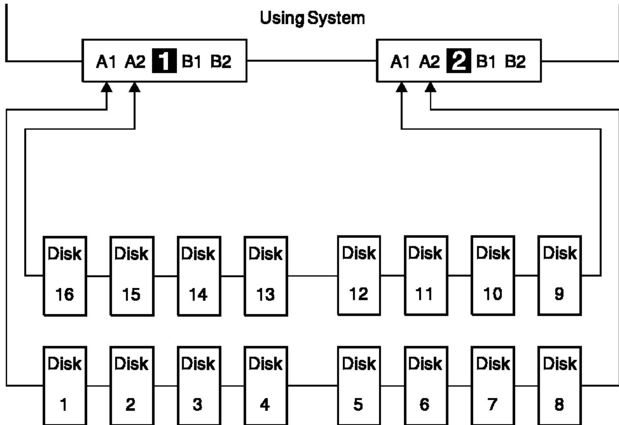
Figure 2-4. One Loop with Two Adapters in One Using System
