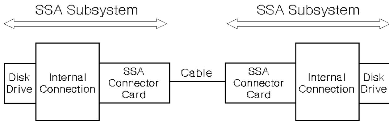
Figure 13-3. Seven-Part Link in Two Subsystems
