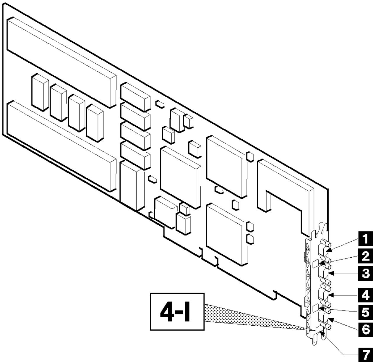
Figure 1-3. The SSA 4-Port RAID Adapter Card (Type 4-I)
