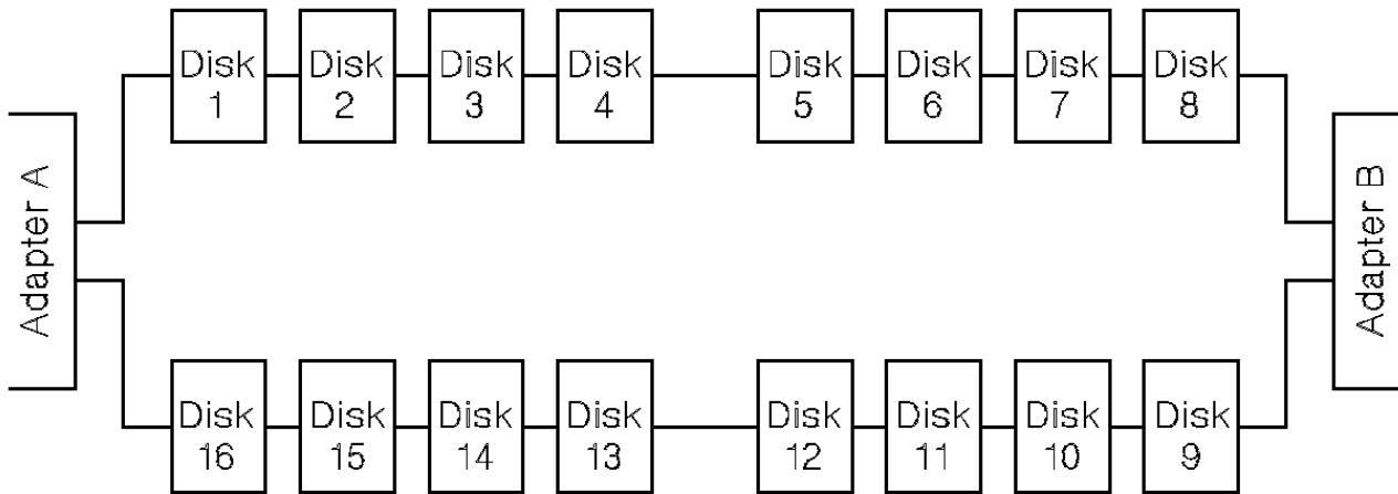
Figure 2-10. Pairs of Connectors in the Loop - Some Shared Data
