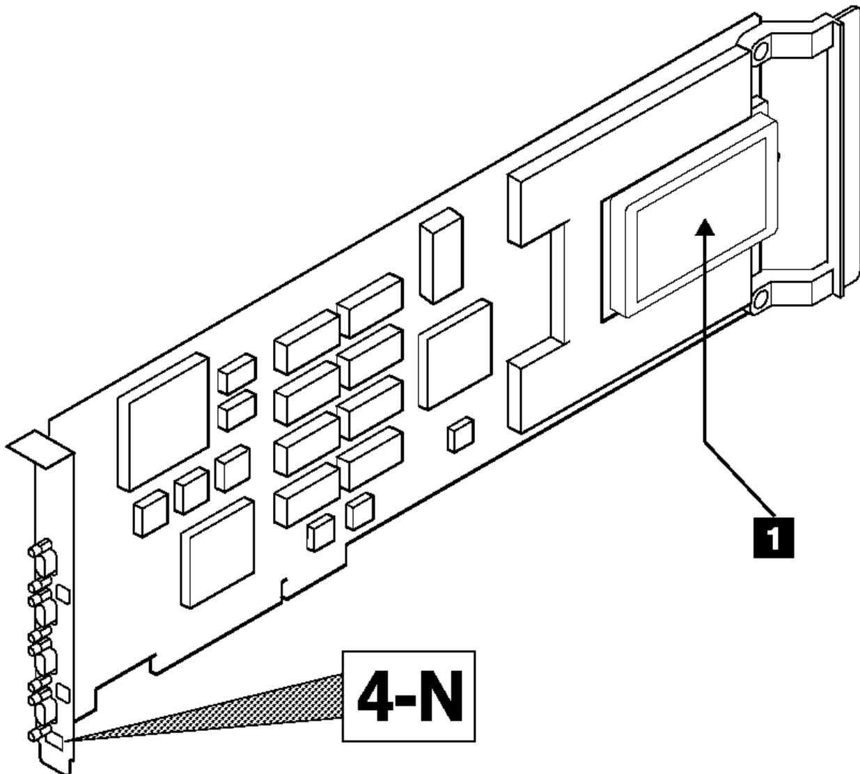
Figure 10-3. The SSA Fast-Write Option Card Installed on a PCI SSA Multi-Initiator/RAID EL Adapter
