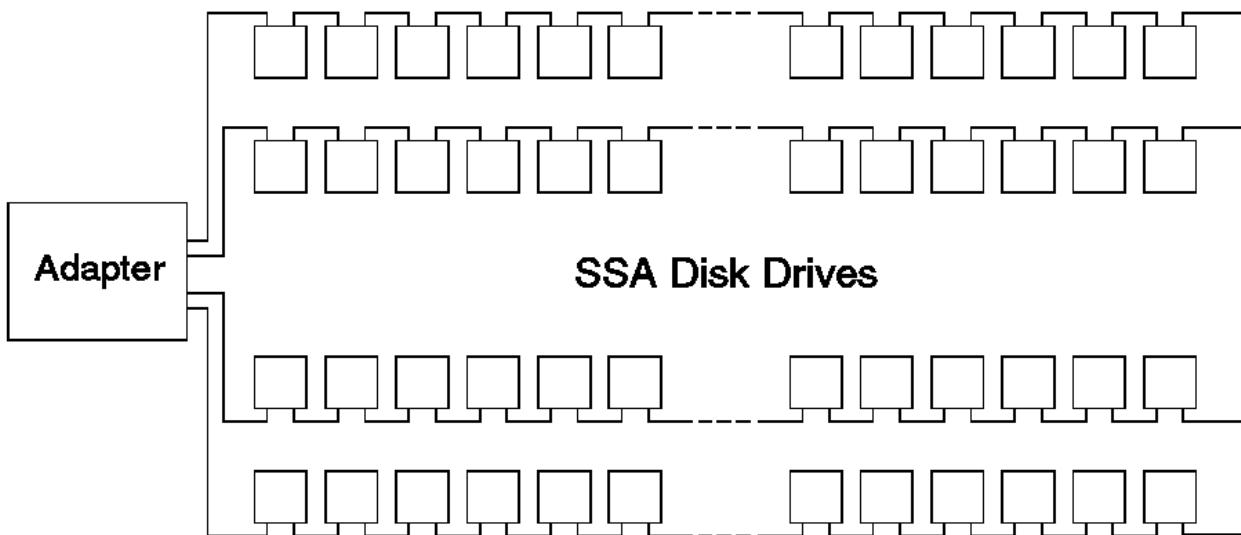
Figure 2-8. Two Loops with One Adapter
