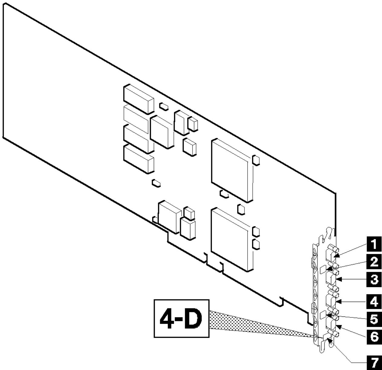
Figure 1-1. The SSA 4-Port Adapter Card (Type 4-D)
