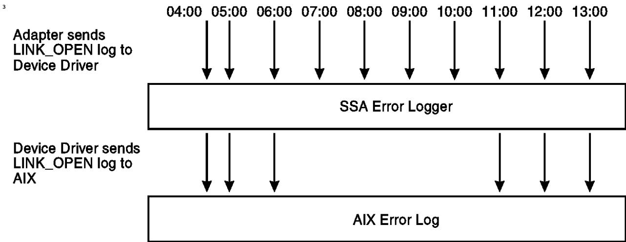
Figure 6-1. Example of an Open Link Error
