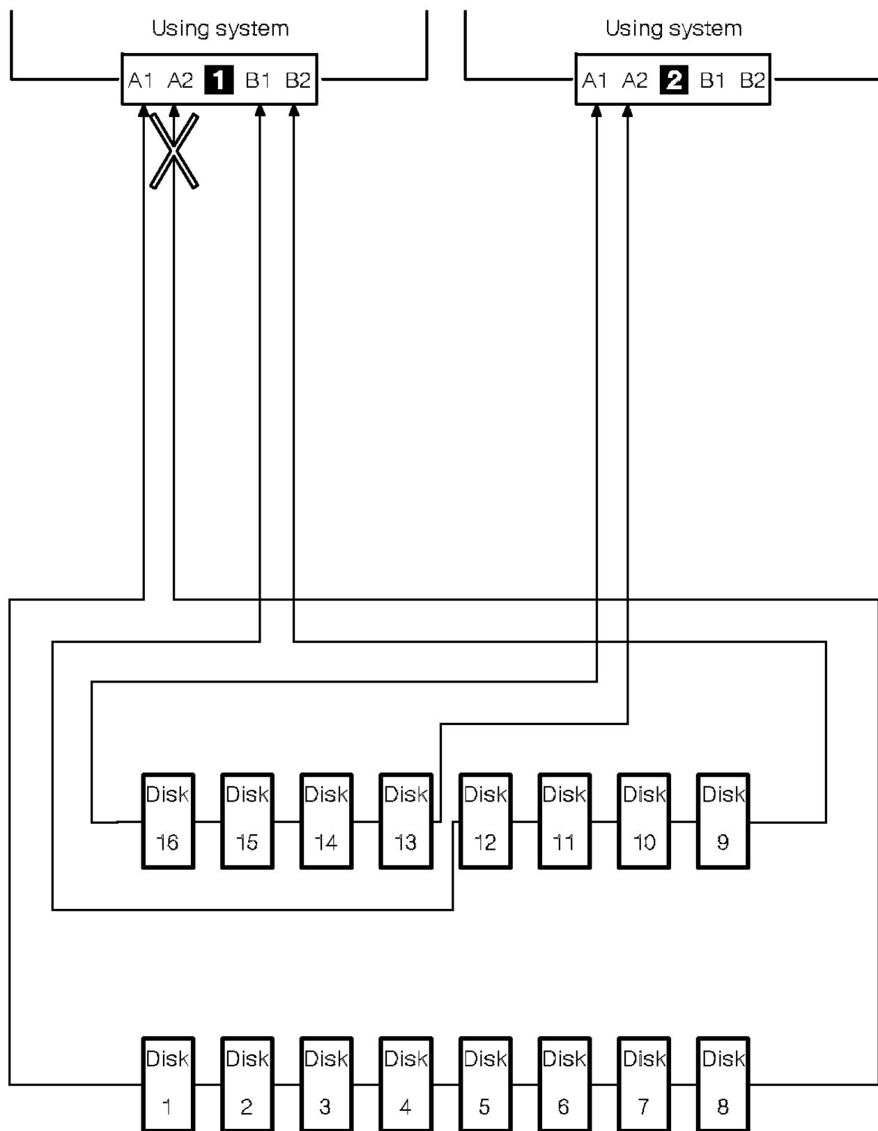
Figure 12-2. Broken Loop (Cable Removed)
