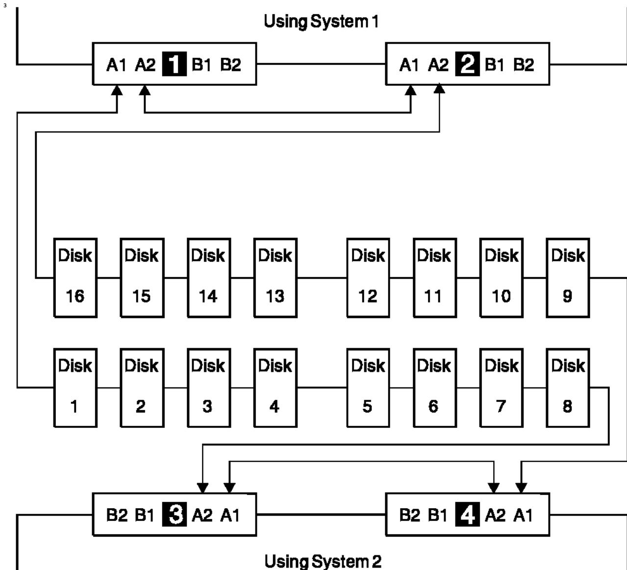
Figure 2-5. One Loop, Two Adapters in Each of Two Using Systems
