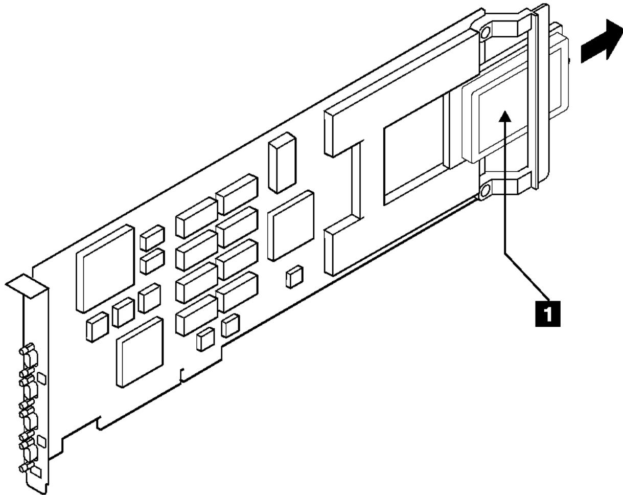
Figure 10-6. Removing the Fast-Write Cache Option Card from a PCI SSA Multi-Initiator/RAID EL Adapter
