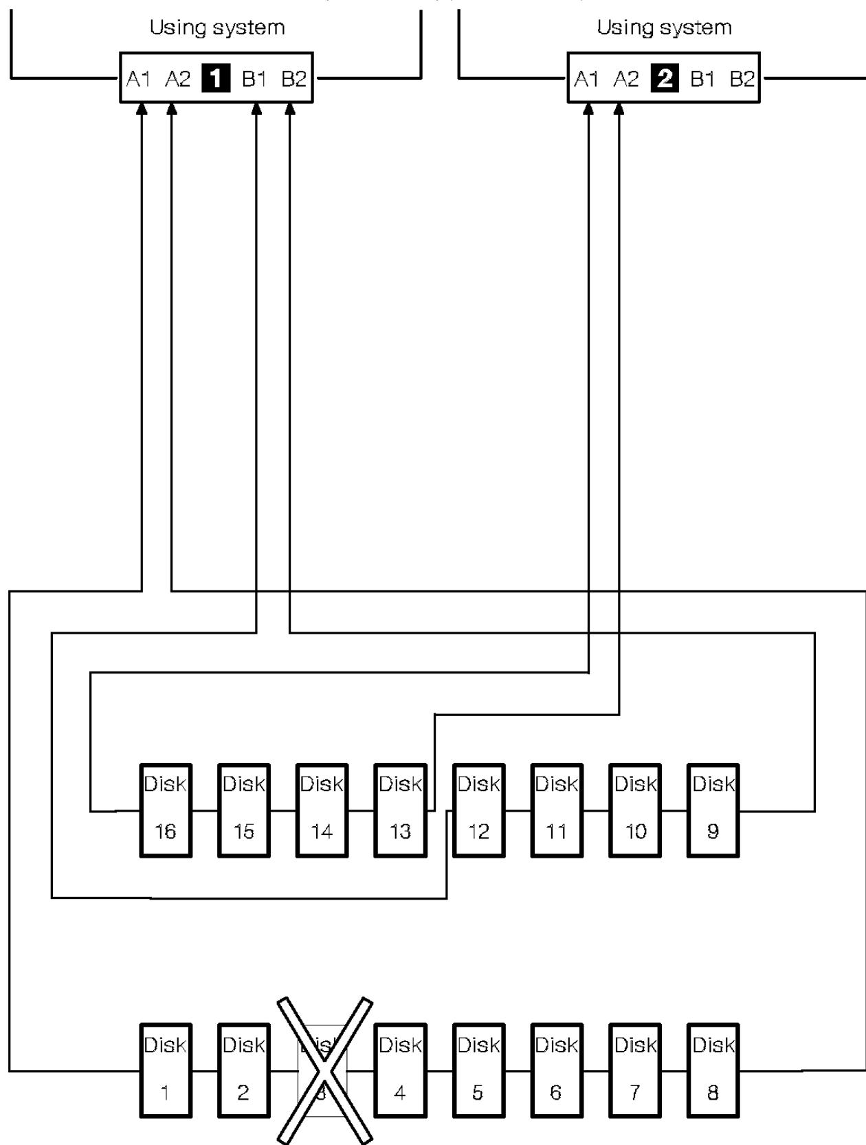
Figure 12-3. Broken Loop (Disk Drive Removed)
