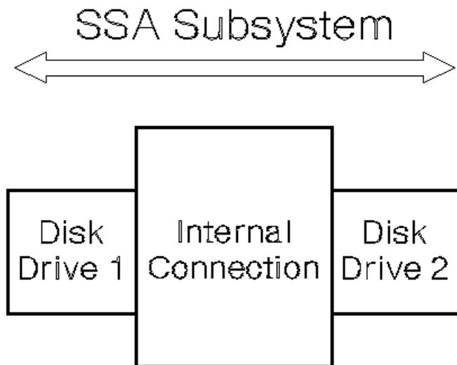
Figure 13-1. Three-Part Link in One Subsystem
