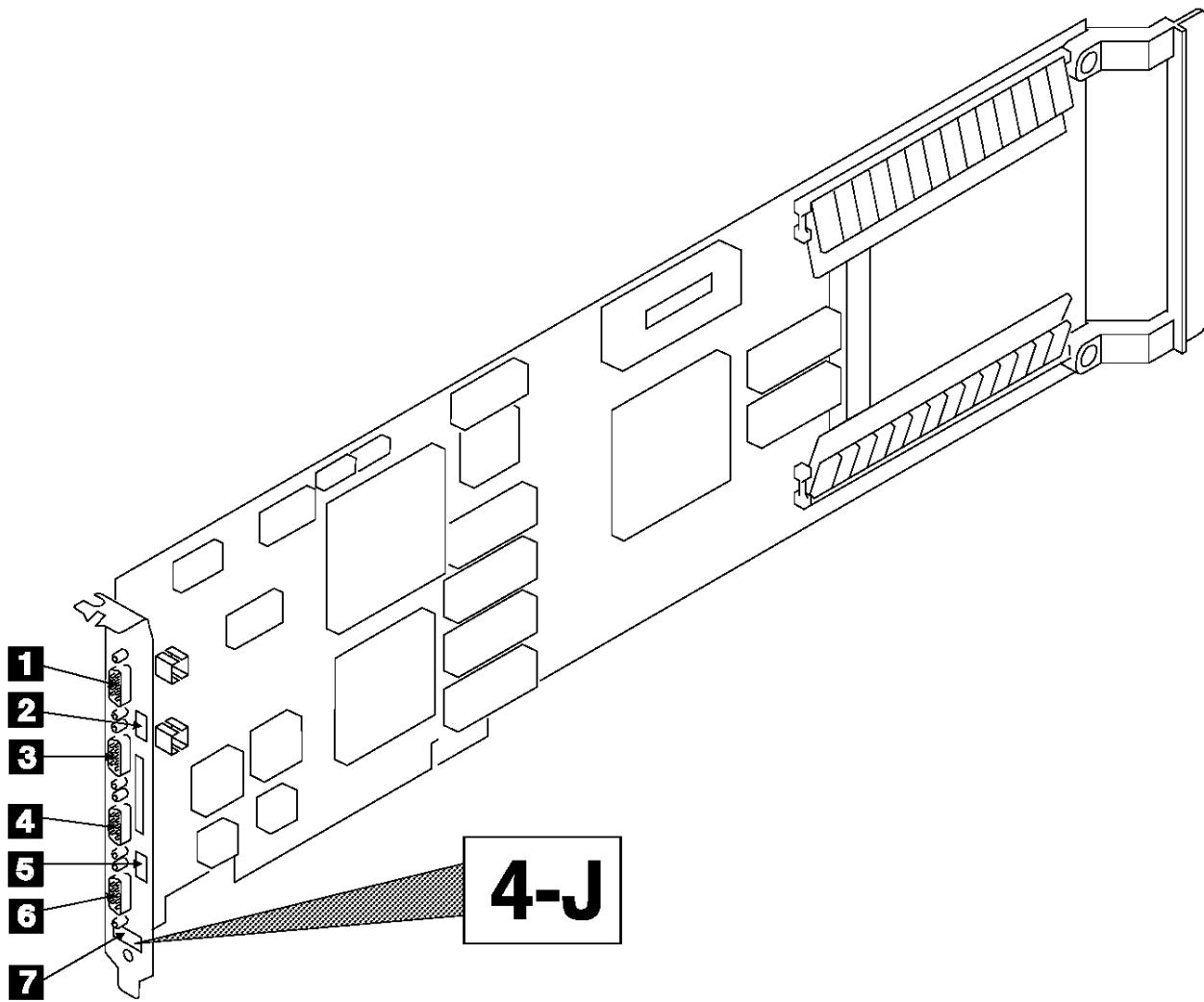
Figure 1-4. The PCI SSA 4-Port RAID Adapter Card (Type 4-J)
