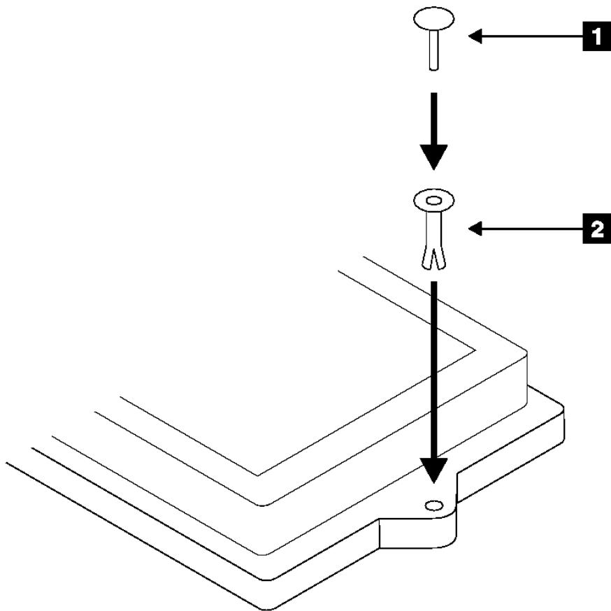
Figure 10-9. Installing the Collar and Pin of the Fast-Write Cache Option Card
