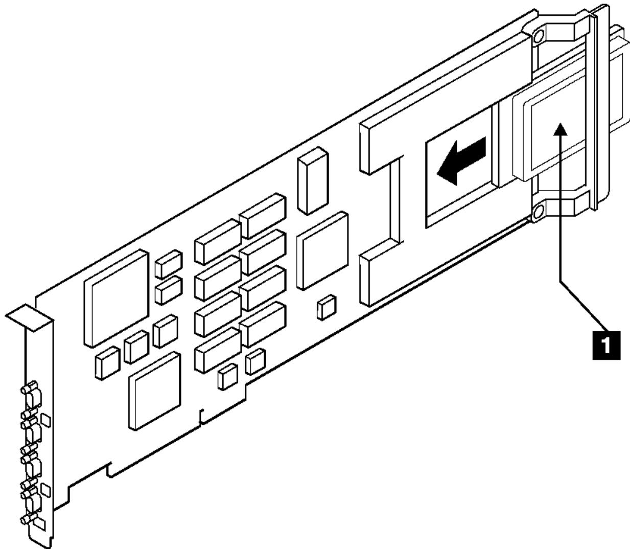
Figure 10-8. Installing the Fast Write Cache Option Card onto a PCI SSA Multi-Initiator/RAID EL Adapter
