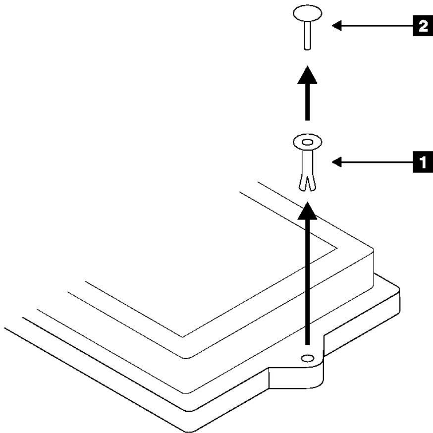
Figure 10-4. Releasing the Fast-Write Cache Option Card
