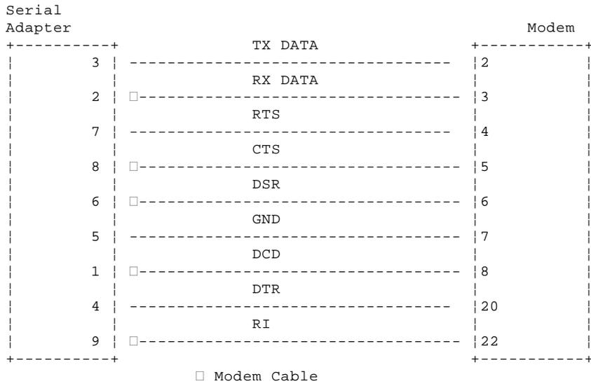
Figure 1. Example of the Serial Adapter Modem Connection
