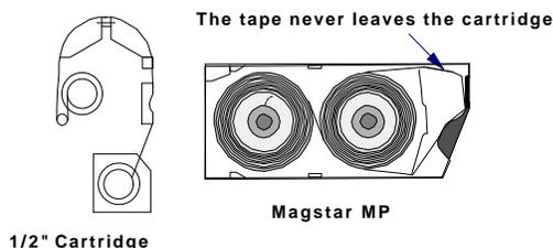
*Figure 4. Longitudinal recording tape paths*
