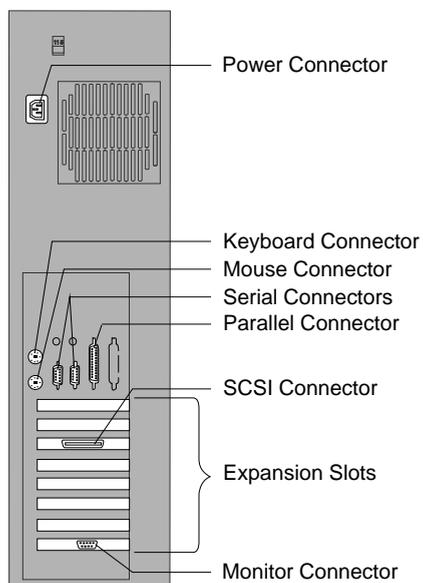
**Power Connector:** The power cable connects here.
