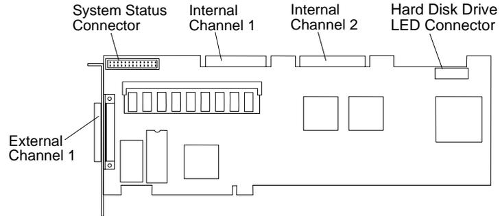
*Note:* Each device attached to the interface must conform to ANSI SCSI Standard X3.131-1986 or X3.131-1994 (SCSI-2). These standards specify the mechanical, electrical, and functional requirements and the command sets that must be used by devices in the SCSI subsystem.
