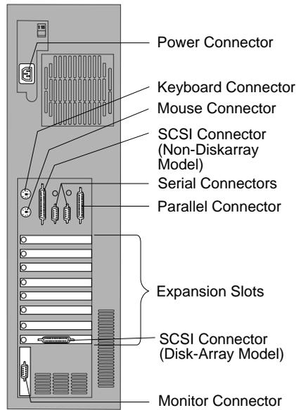
**Power Connector:** The power cable connects here.
