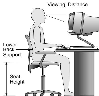
Adjust the monitor so the top of the screen is at, or slightly below, eye level. Place the monitor at a comfortable viewing distance, usually 51 to 61 cm (20 to 24 in.), and position it so you can view it without having to twist your body. Also position other equipment you use regularly, such as the telephone or a mouse, within easy reach.
