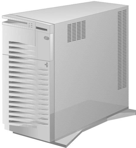
An example is the Model 3516 Hot-Swap Storage Expansion Enclosure, a mini tower that holds up to seven hot-swap hard disk drives. It is shipped without drives, so you must install at least one drive before you attach the enclosure to the server. To connect the enclosure to the external SCSI-2 connector on the server, you need a 68-pin to 68-pin external SCSI-2 cable.
