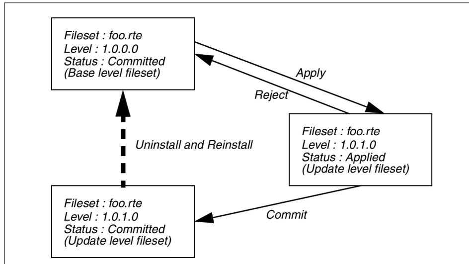
Figure 6-2 State diagram between applied and committed state
