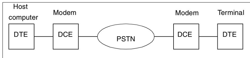
Figure 2-5 DTE and DCE
