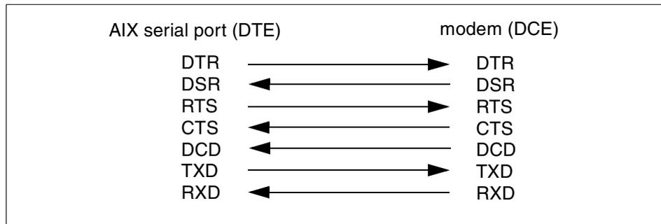
Figure 2-7 Straight serial cable connection
