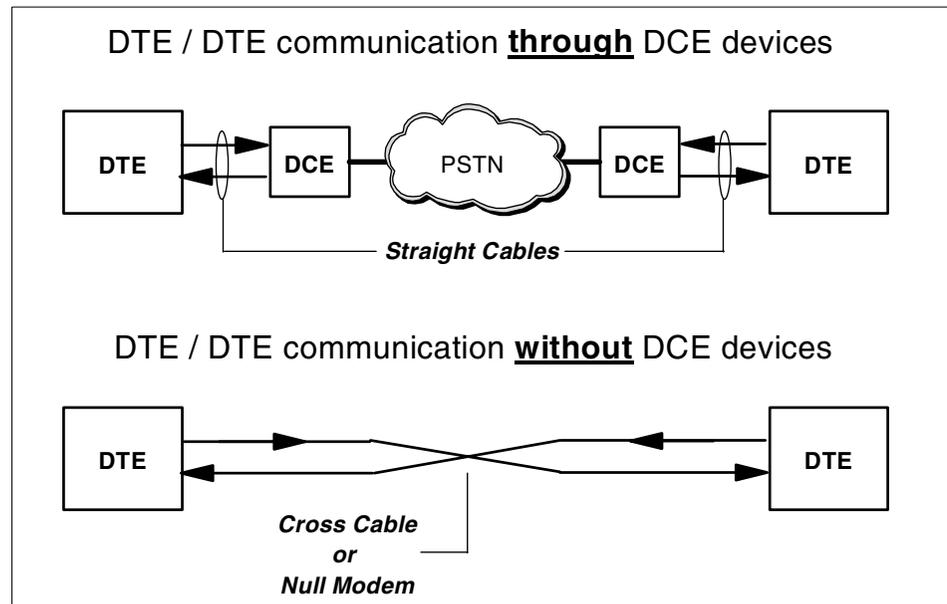
Figure 2-8 Basic concept of null-modem connection
