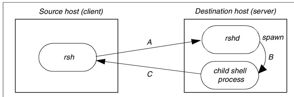
*Figure 4-1 Execution process flow of rsh*
