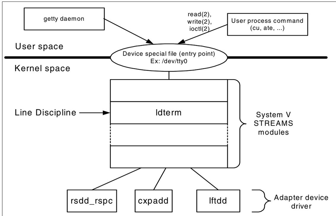
Figure 2-11 Software components used in serial connections on AIX
