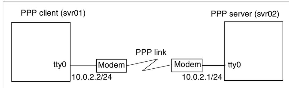
Figure 3-6 PPP sample configuration
