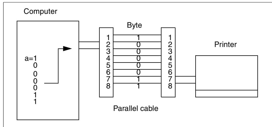
Figure 2-1 Parallel data transmission
