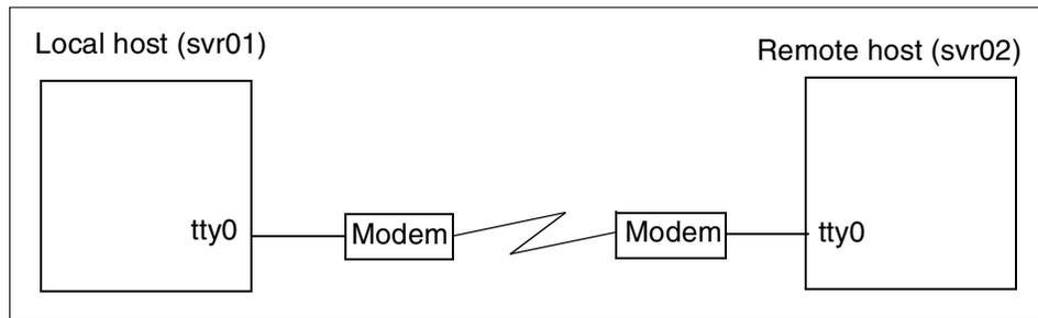
Figure 3-4 ATE connection configuration example
