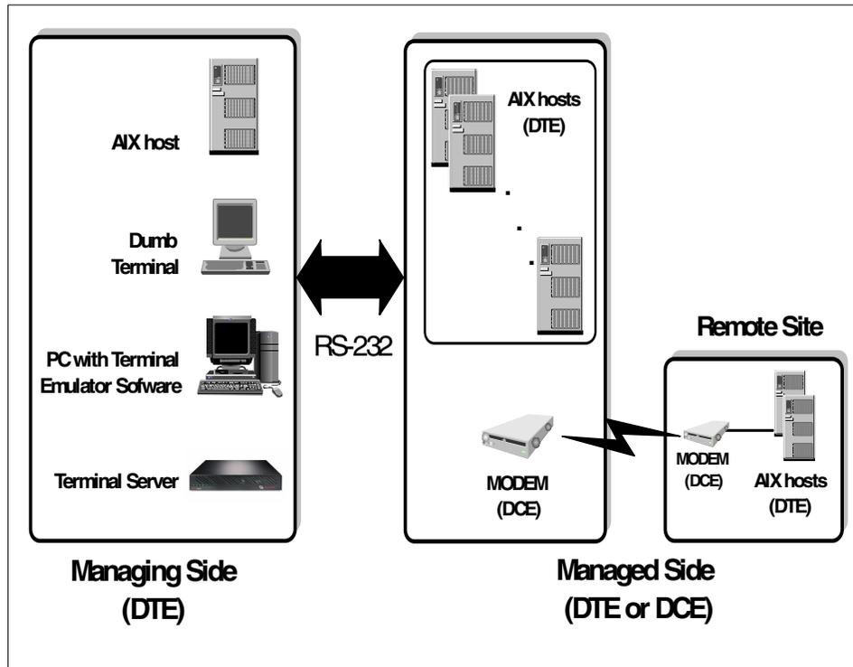
Figure 2-14 Serial device options
