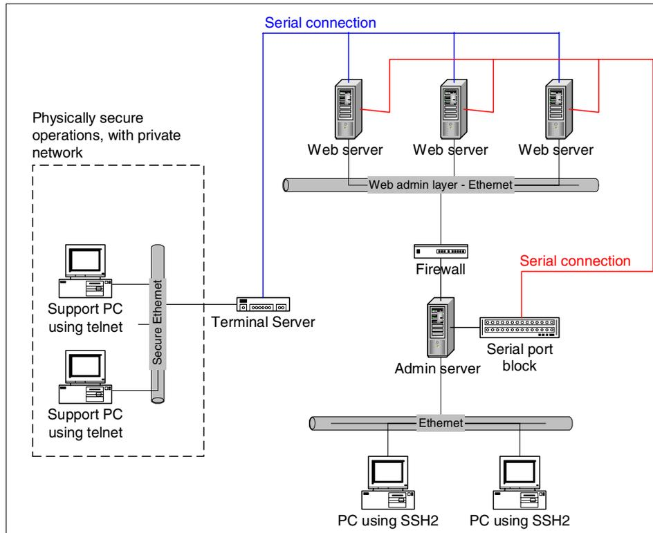
Figure 1-4 Serial connected devices
