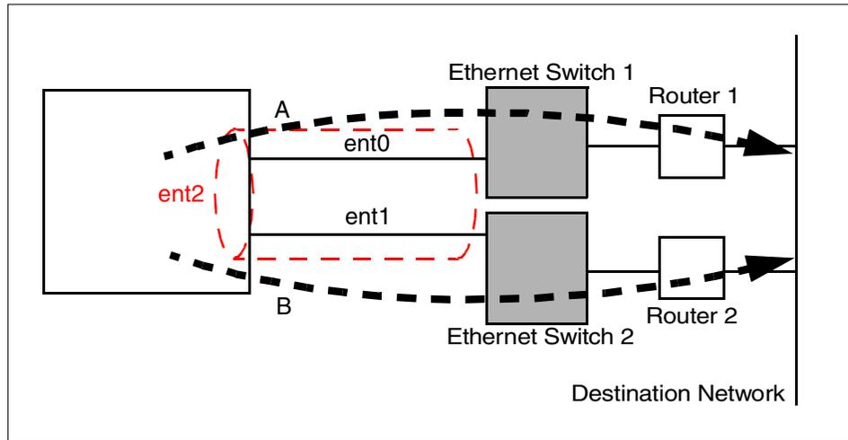
Figure 7-5 Network interface backup using two Ethernet switches
