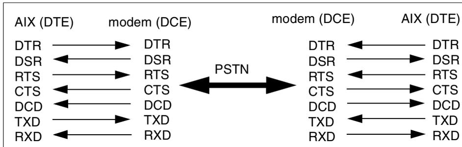
Figure 2-9 AIX to AIX connection over modems
