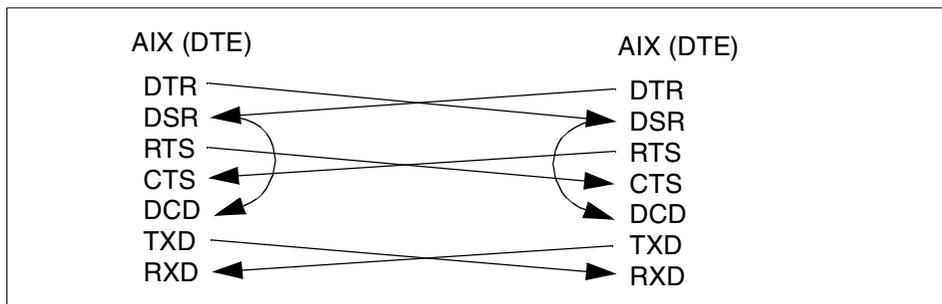
Figure 2-10 Example of null-modem cable connection
