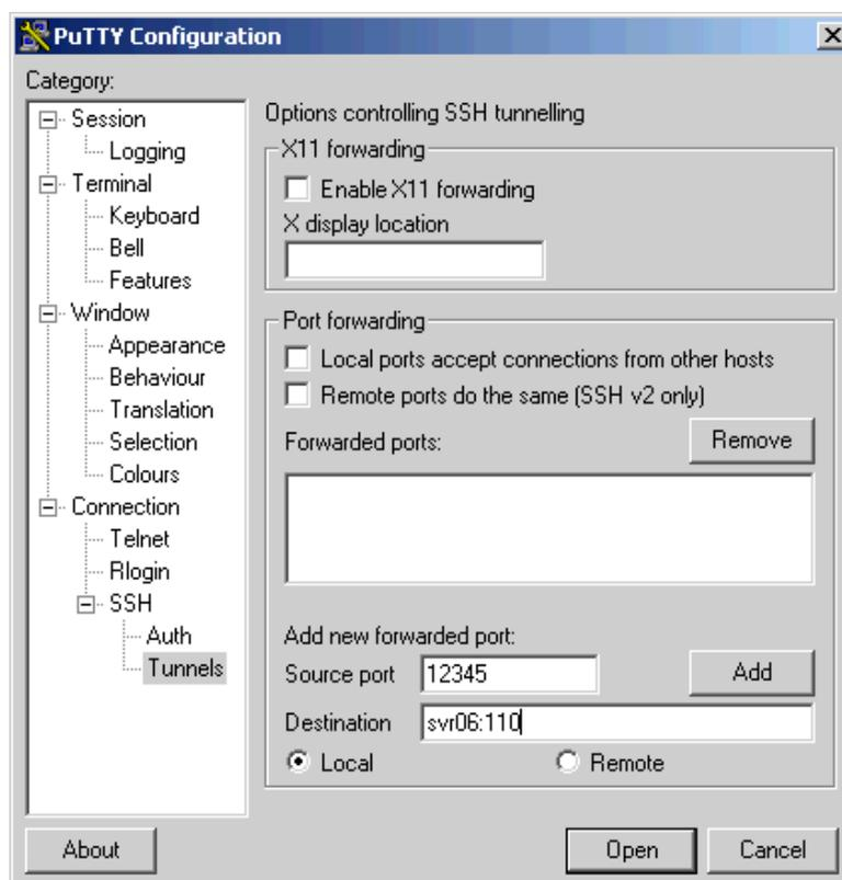
Figure 4-11 TCP/IP local forwarding with PuTTY
