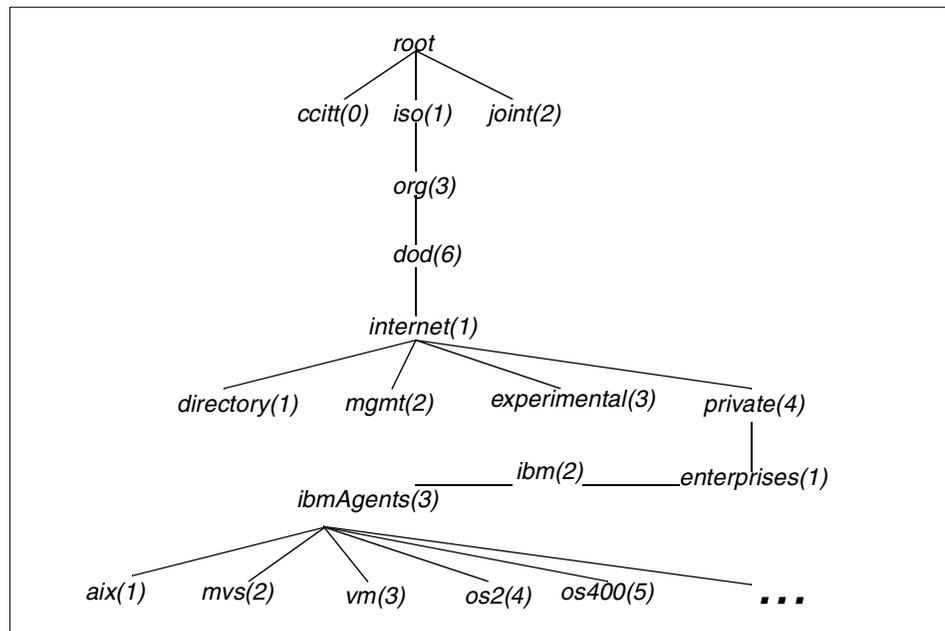
Figure 5-3 IBM MIB tree
