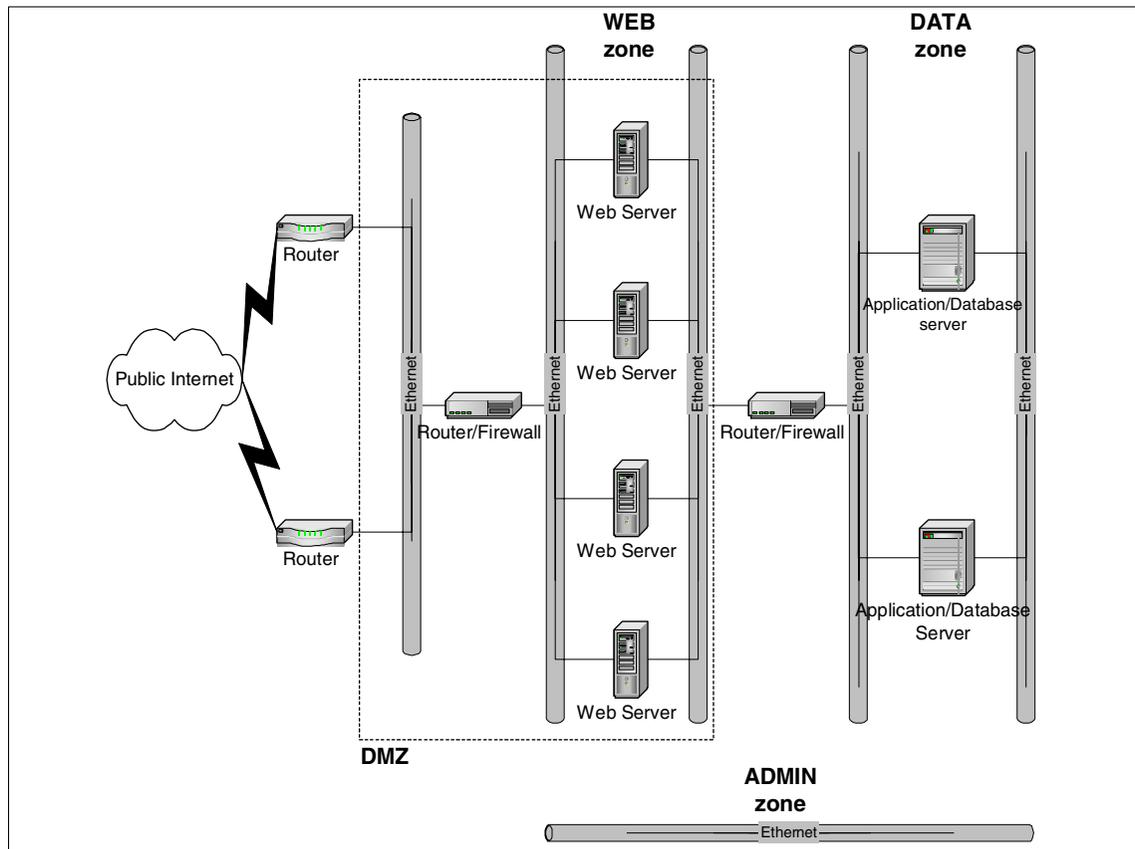
Figure 1-3 Logical network design with DMZ
