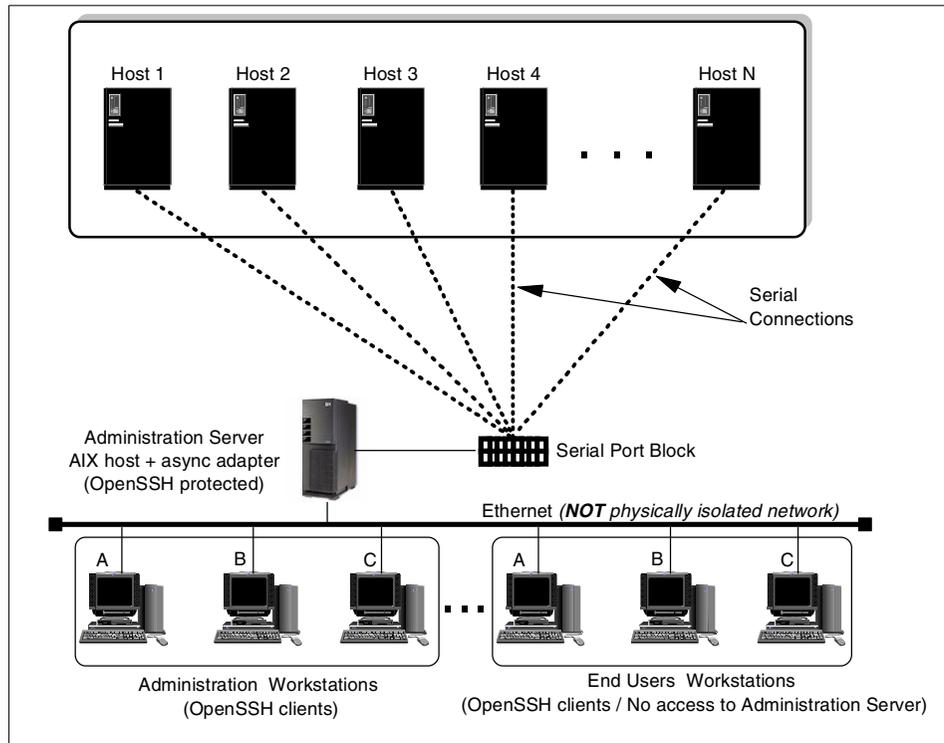
Figure 3-2 Implementing a terminal server using an AIX system
