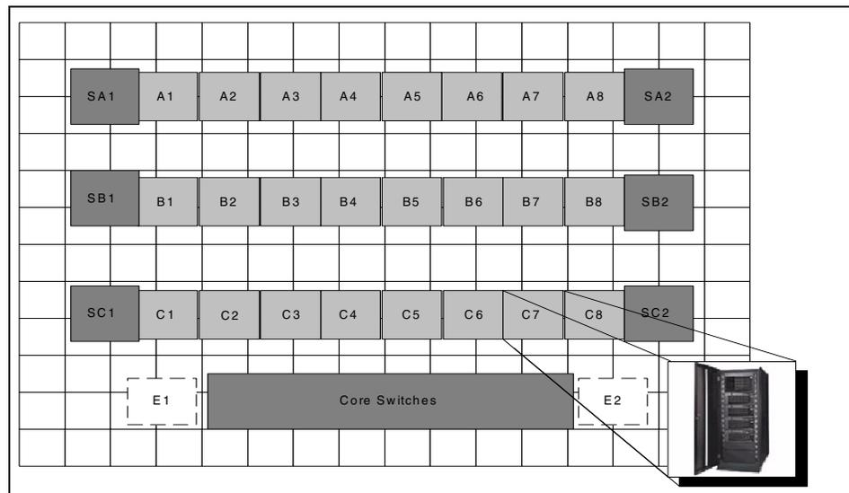
Figure 1-1 Physical racks layout for a large server farm
