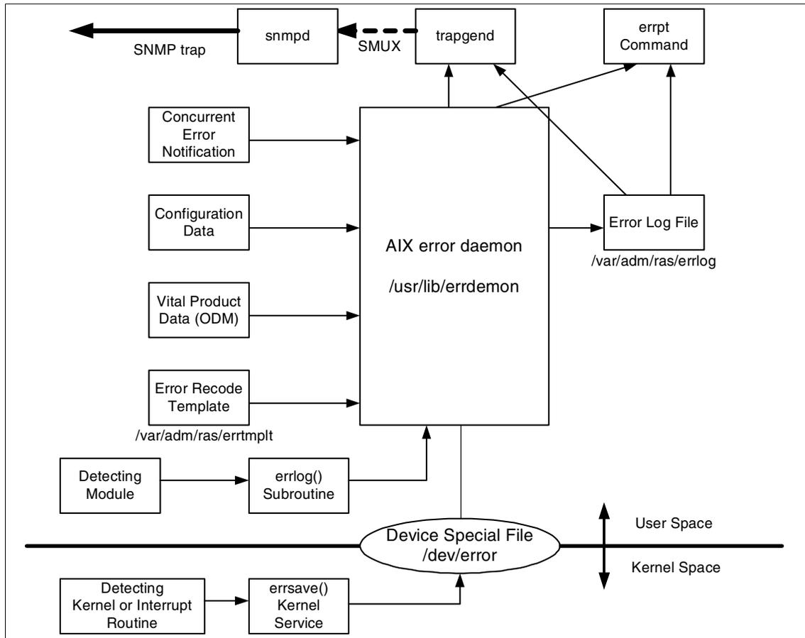
Figure 5-6 Sending an alertable error using trapgend
