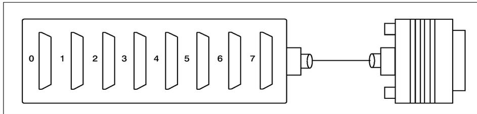
Figure 2-12 8-port asynchronous cable with fanout box
