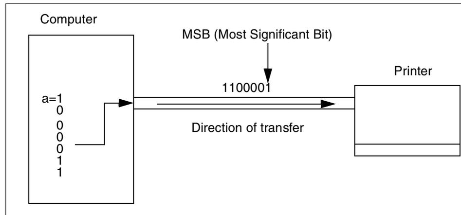
Figure 2-2 Serial data transmission
