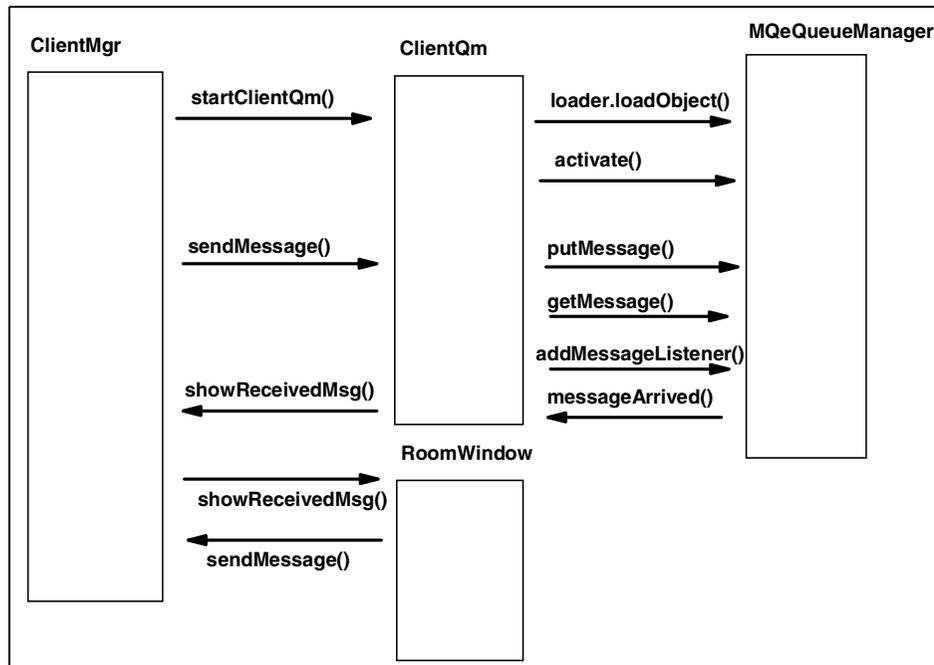
Figure 14-8 Class object interaction - client side
