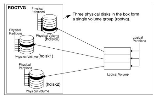
Figure 6-1 Relationship between logical storage components
