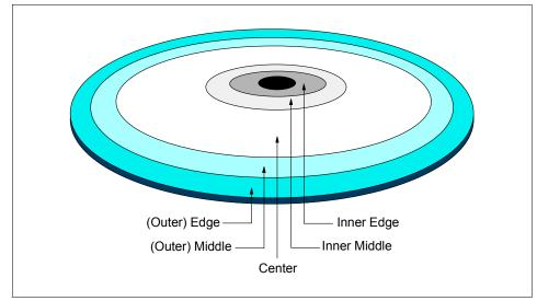
Figure 6-45 Physical partition mapping
