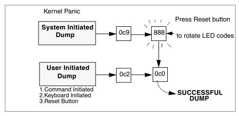
Figure 8-4 Successful system dumps - LED codes
