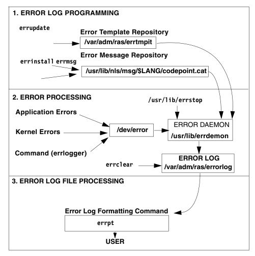
Figure 8-1 Error logging subsystem overview
