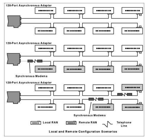
Figure 4-12 128-port asynchronous adapter connection combinations
