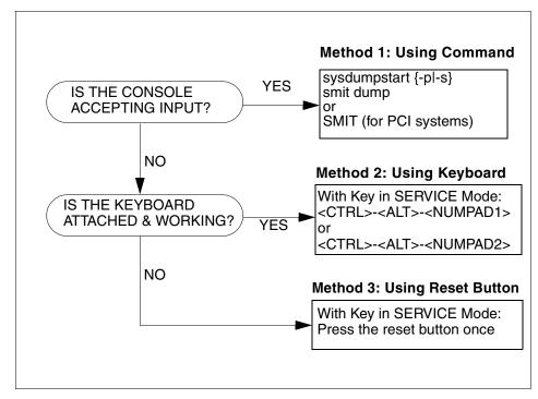
Figure 8-7 Method of user initiated system dump
