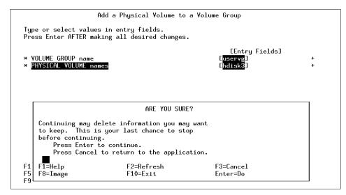
Figure 6-25 Add a Physical Volume to a Volume Group - confirmation screen
