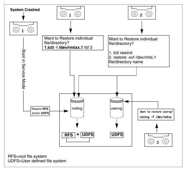
Figure 9-4 Flowchart for restoring information
