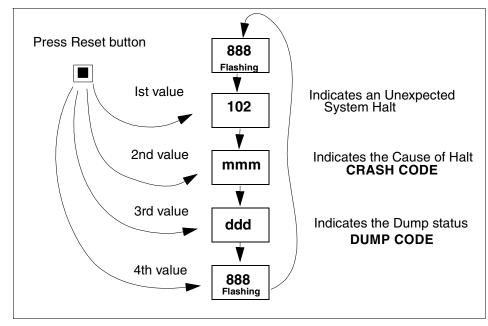
Figure 8-6 Unexpected system halt - Three-digit display string
