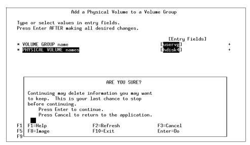
Figure 6-30 Add a Physical Volume to a Volume Group - confirmation screen
