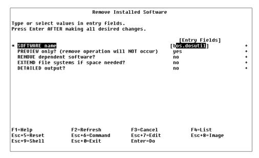
Figure 13. Removing software through SMIT
