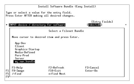
Figure 7. Installing user defined bundle
