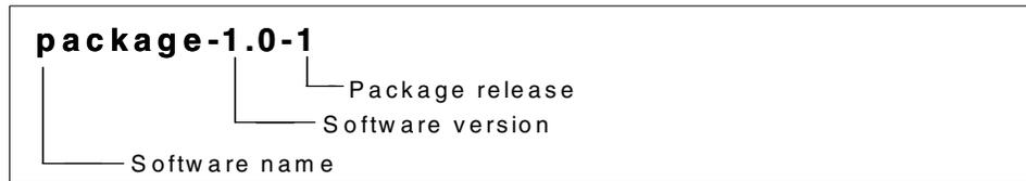
Figure 2-2 Sample of RPM package naming convention
