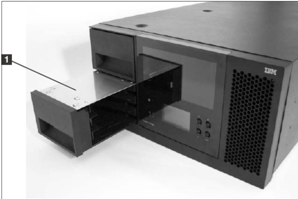
*Figure 8-8 I/O station of the TS3400*
