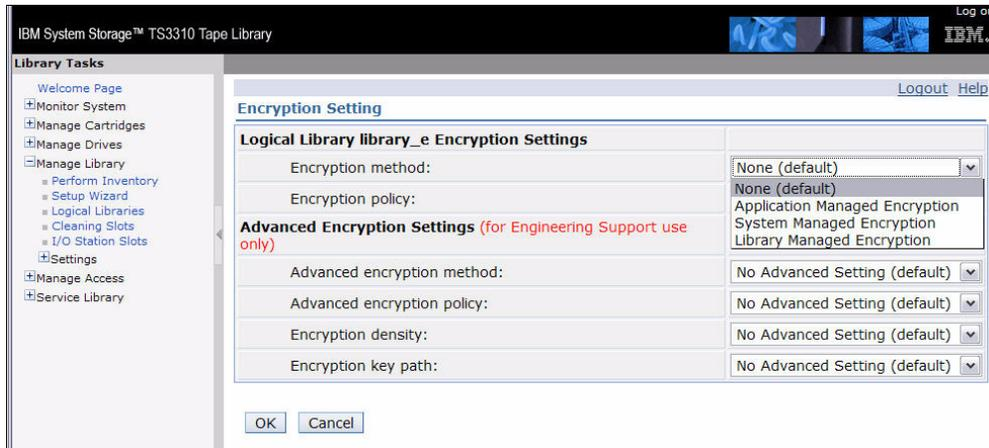
Figure 7-11 Selection Encryption method
