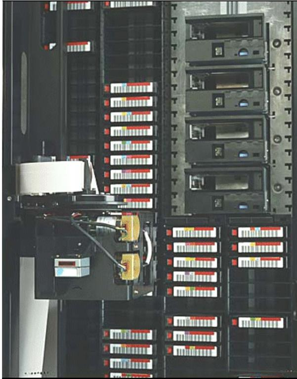
Figure 9-10 IBM TS3500 Tape Library accessor assembly
