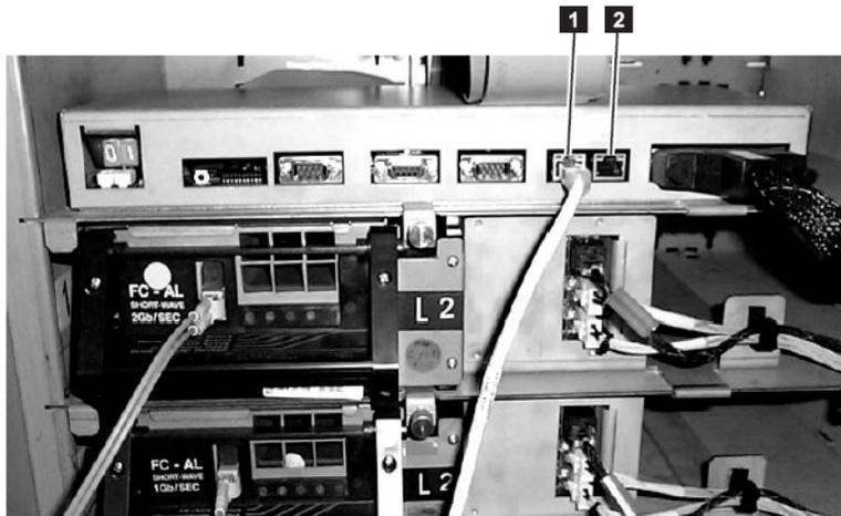
Figure 9-8 View of Medium Changer Assembly identifying the two Ethernet ports
