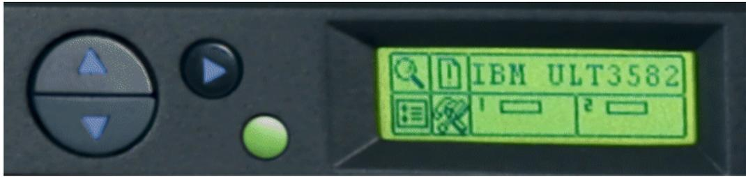
Figure 14-4 IBM 3582 Operator Panel
