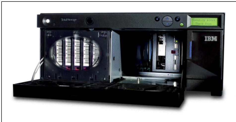
Figure 14-2 IBM 3582 seven-slot magazines
