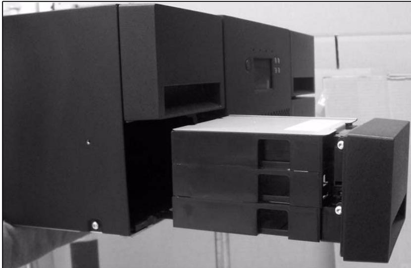
Figure 6-13 TS3200 I/O station in the lower left magazine
