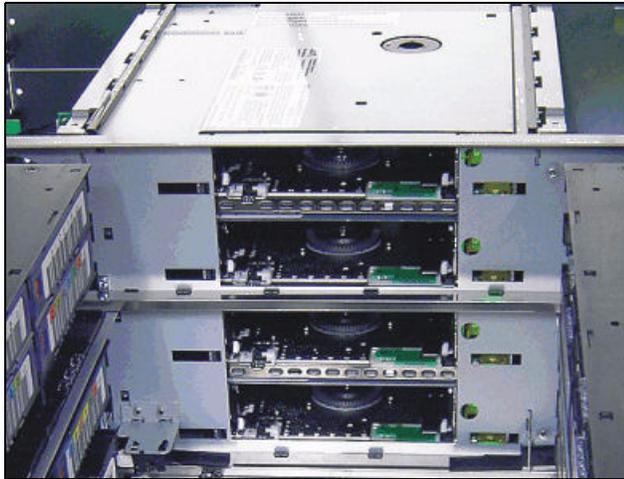
Figure 6-6 Interior of the TS3200 with four Ultrium 3 Half-High drives installed
