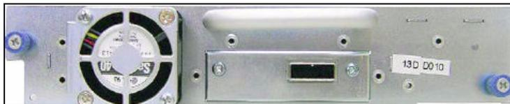
Figure 5-11 Back side of the SAS Half-High Tape Drive
