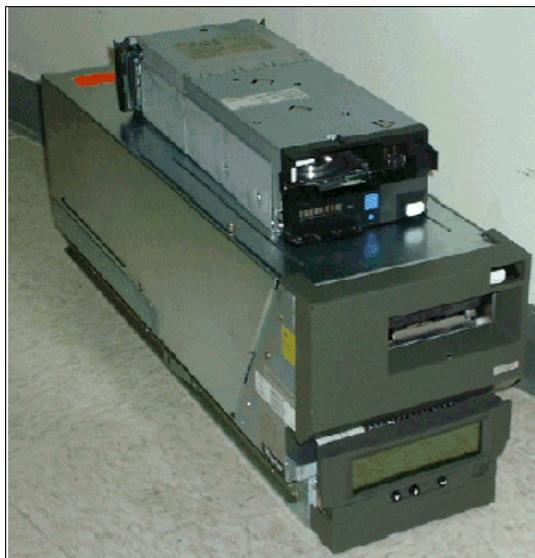
Figure 2-46 The IBM 3590 and IBM 3592 Tape Drive Model J1A
