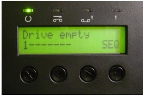
Figure 13-4 IBM 3581 2U Operator Control Panel
