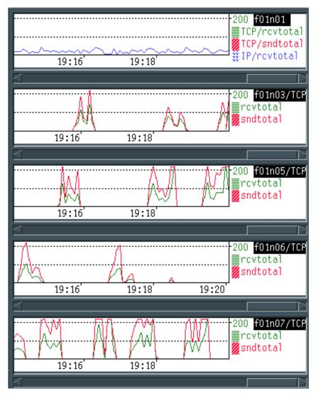
Figure 12. Network Traffic - ISS with Idle CPU ResourceType for Dynamic Pages
