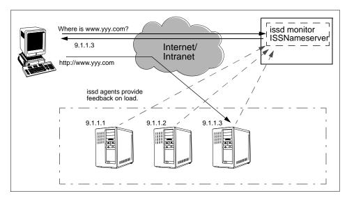
Figure 5. ISS Configured with an ISSNameserver Observer
