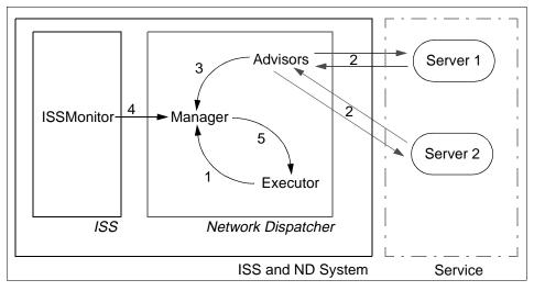
Figure 3. Typical Flow of Information in Network Dispatcher
