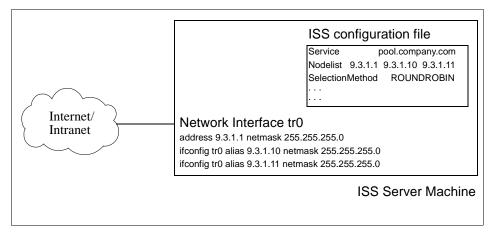
Figure 29. Example of Minimum Configuration for ISS in Round-Robin
