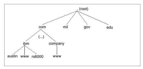
Figure 30. Example of Domain Structure
