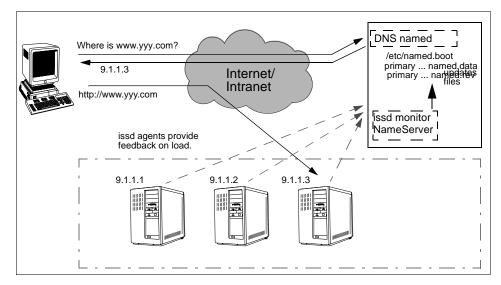
Figure 4. ISS Configured with a NameServer Observer
