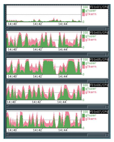
Figure 13. CPU Load Using Network Dispatcher for Dynamic WWW Pages
