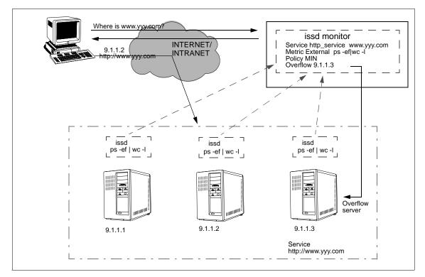
Figure 7. ISS Using an External Metric
