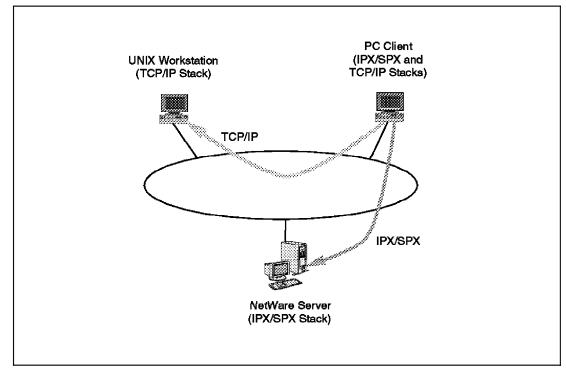
Figure 45. IPX/SPX and TCP/IP Stacks on one Machine
