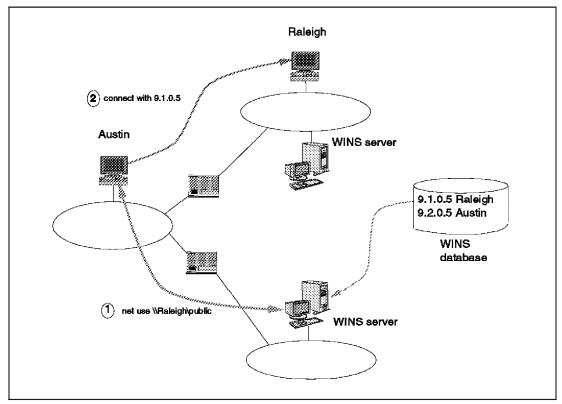
Figure 39. Request and Resolving of IP Address Mapping
