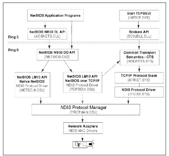
Figure 19. NetBIOS, NetBIOS over TCP/IP and TCP/IP Structure
