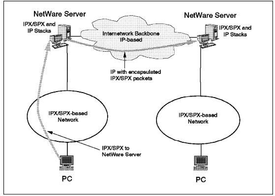
Figure 47. Tunneling IPX within IP
