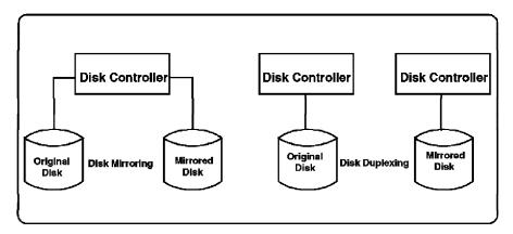
Figure 58. Disk Mirroring versus Disk Duplexing
