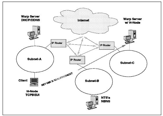
Figure 31. Ideal Solution with DHCP/DDNS plus NBNS
