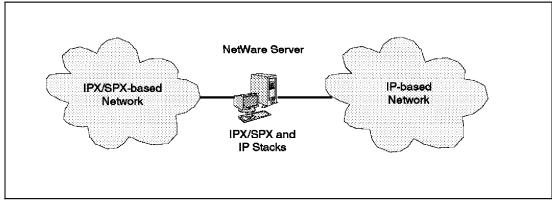
Figure 46. Different Network Protocols Connected via Gateway
