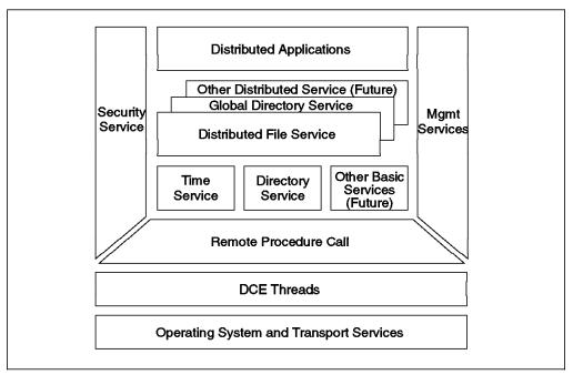
Figure 6. DCE Architecture
