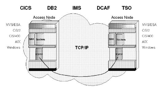
Figure 221 shows a scenario for SNA over TCP/IP.
