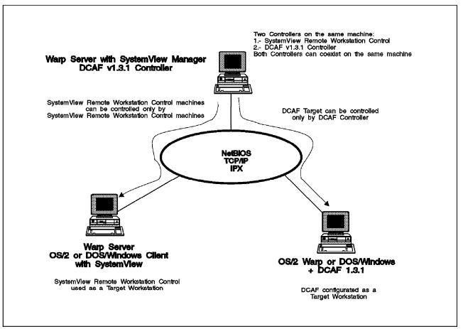
Figure 80. DCAF and SystemView: Rules for Coexistence and Interoperability
