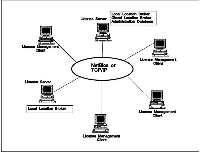
Figure 79. Cell with Two License Servers and Three Clients
