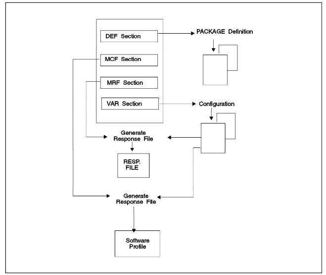
Figure 164. ADF File Schematic
