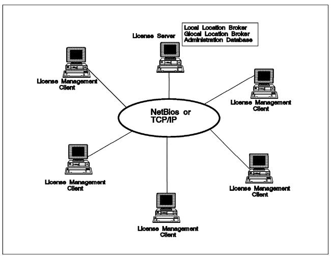
Figure 78. Simple NCS Cell - All Processes Run on One Server
