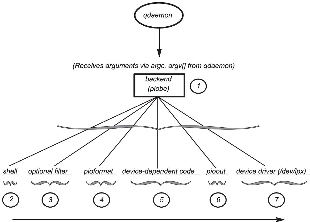
Figure 2. Datastream Flow for Common Print Jobs
