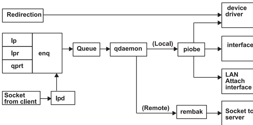
Figure 1. Printing with the Base Operating System
