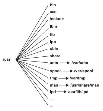
Figure 8. /usr File System. This diagram shows the major subdirectories of the /usr directory, which includes: /bin, /ccs, /lib, /lpp, /adm and its /var/adm subdirectory, and /man and its /usr/share/man subdirectory.
