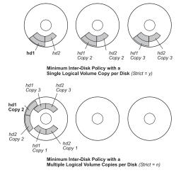
Figure 5. Minimum Inter-Disk Policy/Strict. This illustration shows that if the Strict option is equal to Yes, each copy of the logical partition is on a different physical volume. If Strict is equal to No, all copies of the logical partitions are on a single physical volume.
