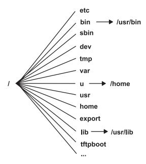
Figure 7. Root File System. This diagram shows the root file system and its subdirectories. The **/bin** subdirectory points to the **/usr/bin** directory. The **/lib** subdirectory points to the **/usr/lib** directory. The **/u** subdirectory points to the **/home** directory.
