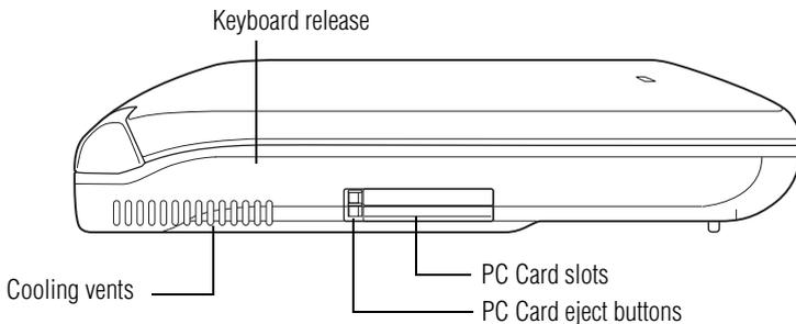
The **cooling vents** prevent the computer's central processing unit (CPU) from overheating so that it can continue to perform at its maximum speed.
