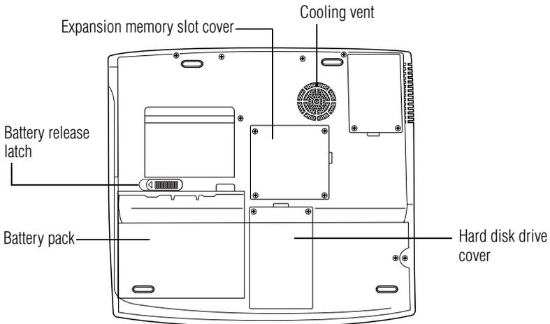
The **expansion memory slot cover** protects the slots where you insert additional memory. See “[Installing additional memory \(optional\)](#)” on page 57 for detailed information.
