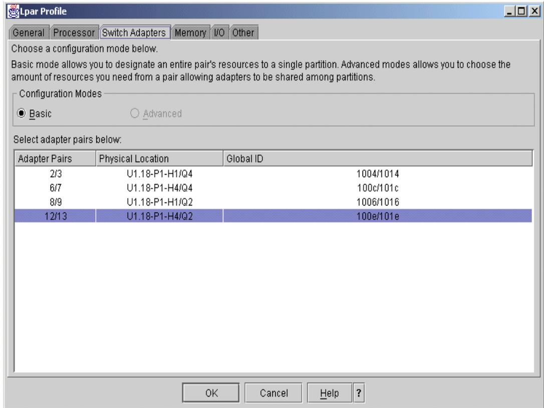
Figure 15 Adding the SNIs to an existing LPAR
