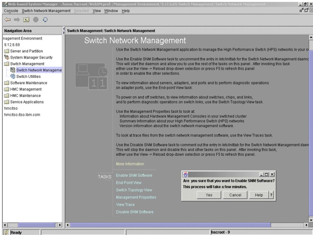
Figure 16 Enable the Switch Network Management software
