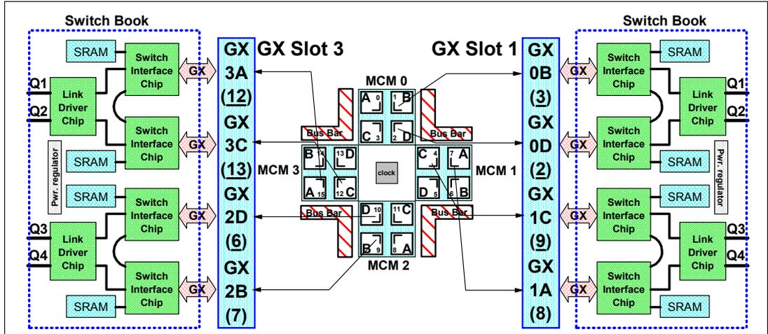
Figure 6 MCM to GX to switch adapter relationship
