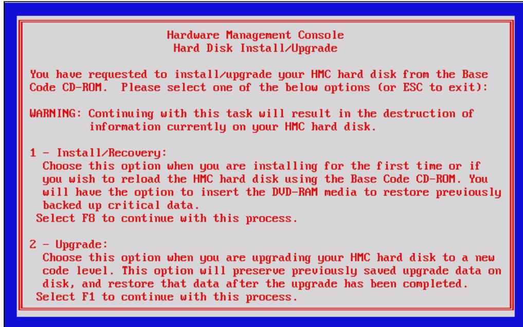
Figure 10 Install/Upgrade HMC screen
