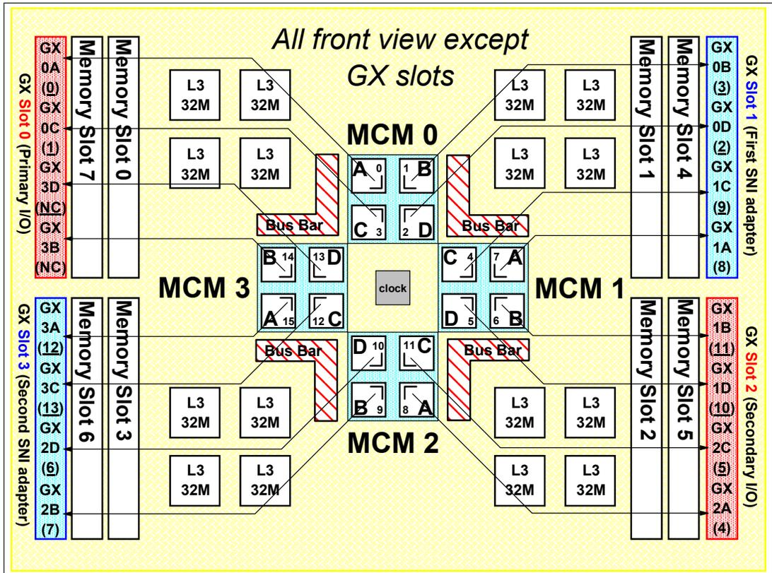
Figure 5 p690 MCM to GX bus activation chart
