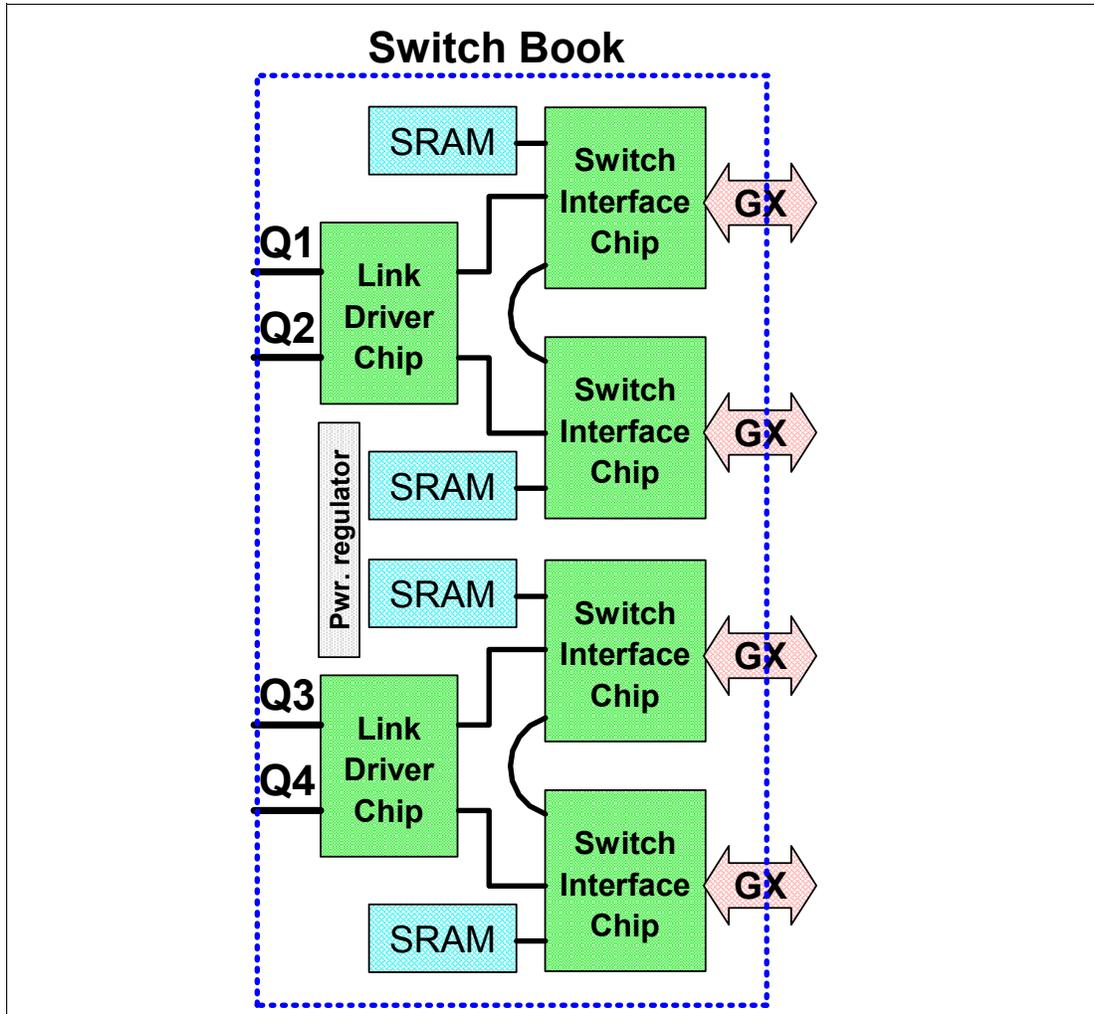
Figure 4 Switch Network Interface card diagram
