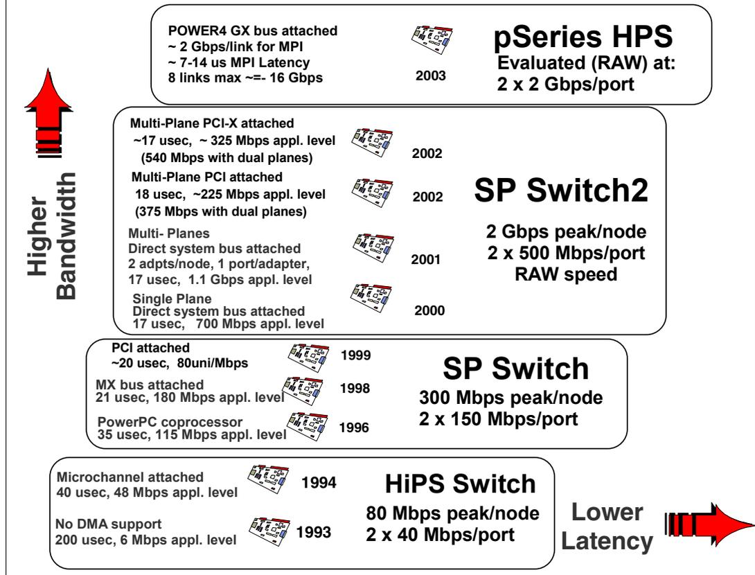
Figure 1 IBM switch evolution
