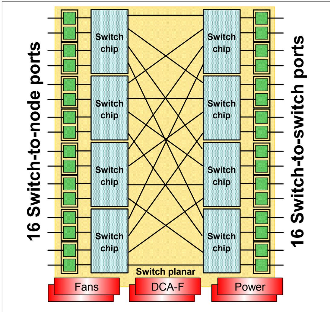
Figure 2 HPS board: 1 plane, 32-port topology
