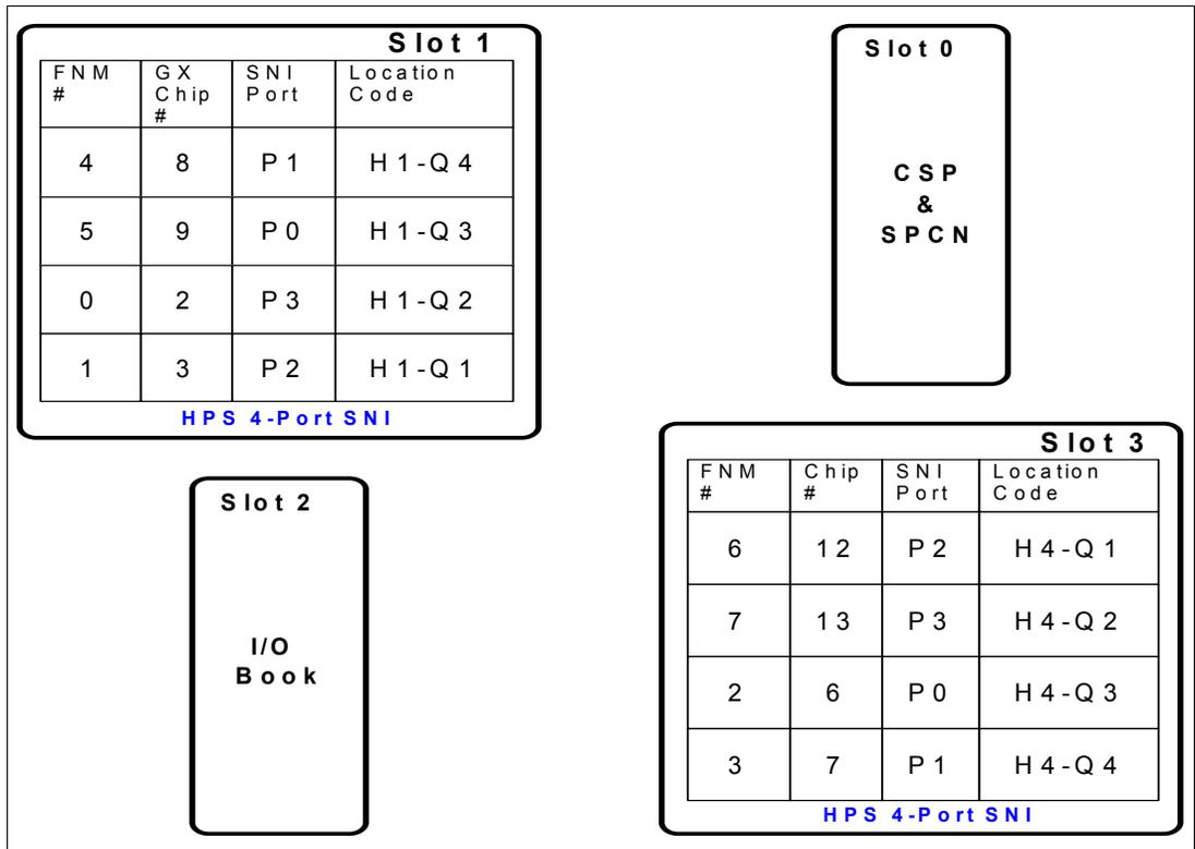
Figure 7 SNI to GX bus map: Physical location codes
