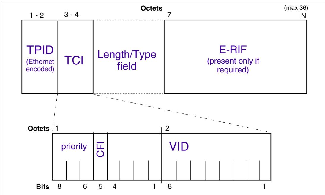
Figure 2 VLAN tag format for Ethernet
