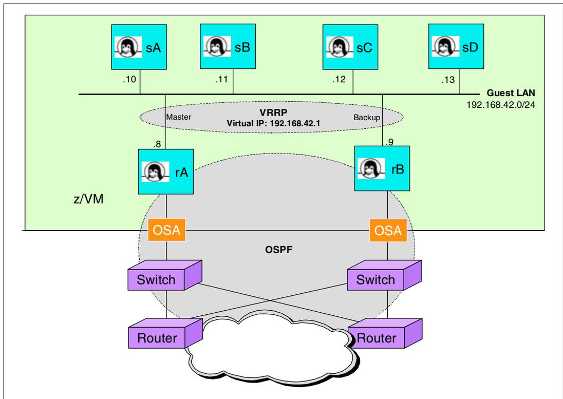
Figure 4 Connectivity based on Linux routers
