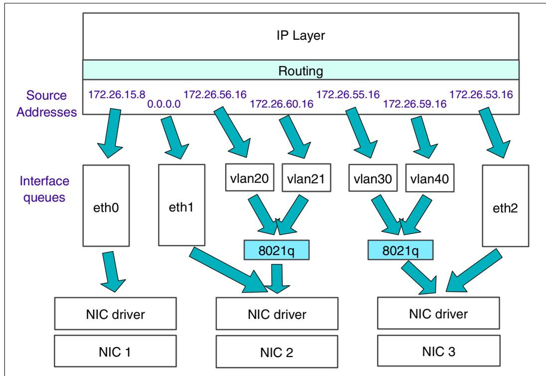
Figure 3 Layer diagram for VLAN-capable devices
