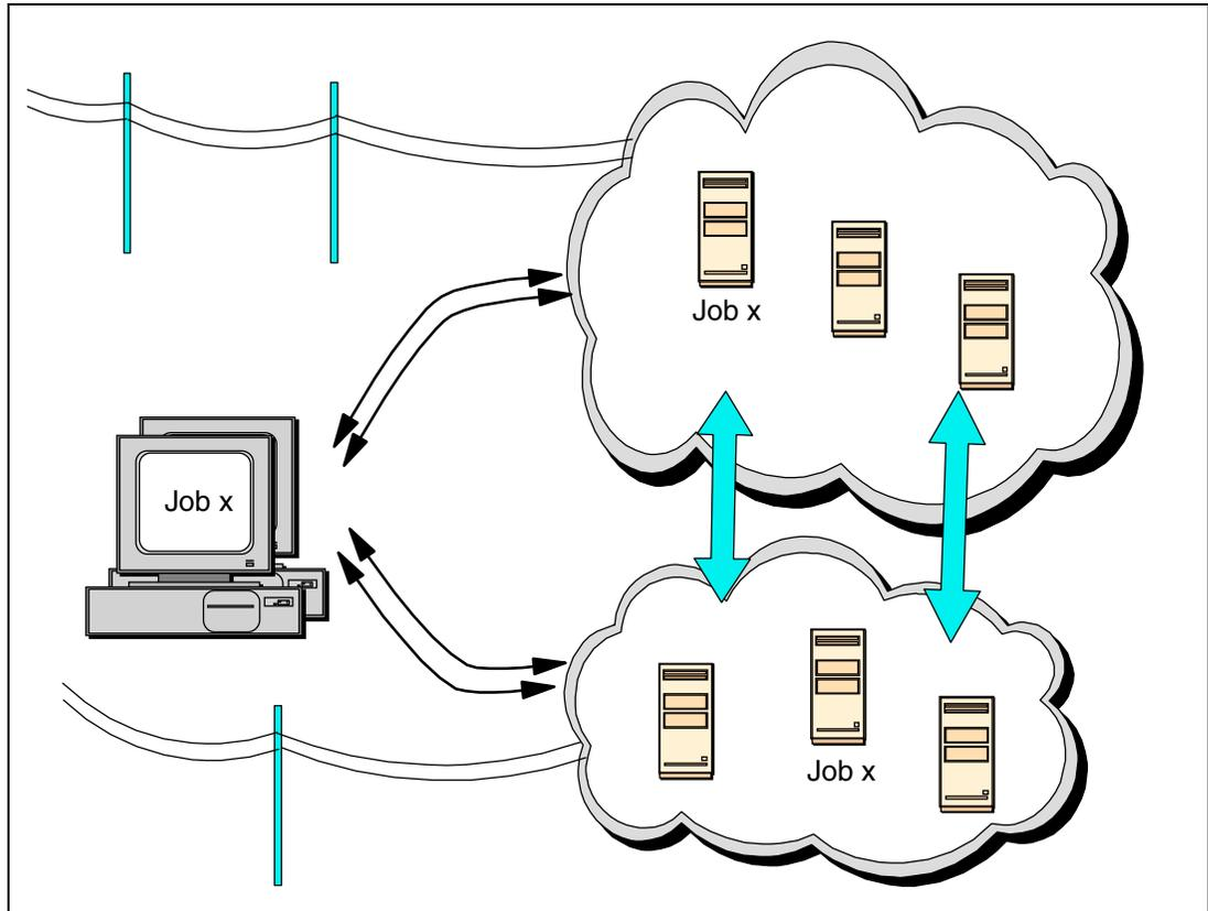
Figure 3 Redundant grid configuration and redundant job submission used to achieve high reliability
