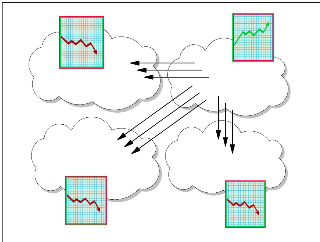
*Figure 2 Jobs are migrated to less busy parts of the grid to balance resource loads and absorb unexpected peaks of activity in a part of an organization*
