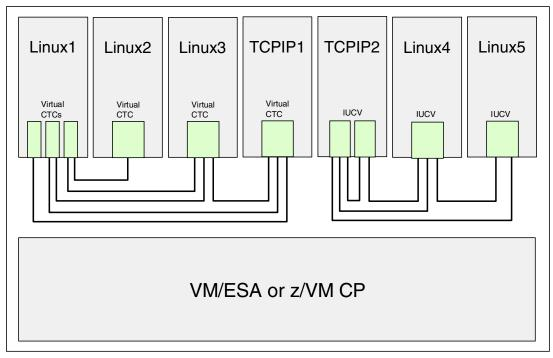
Figure 1 VM point-to-point connections
