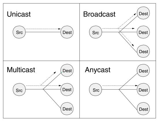
Figure 3 IP packet delivery modes (showing delivery from source to destination)
