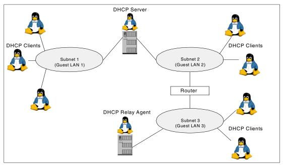
Figure 4 DHCP network components
