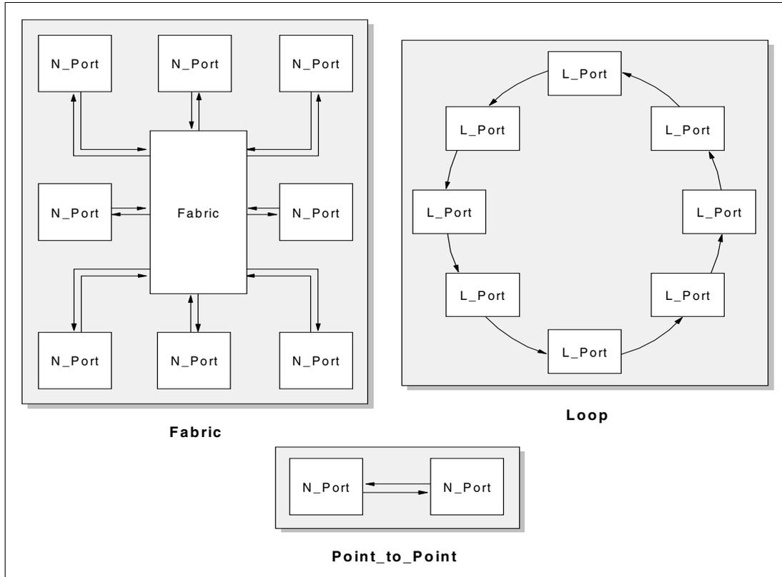
Figure 1-2 Fibre Channel topologies
