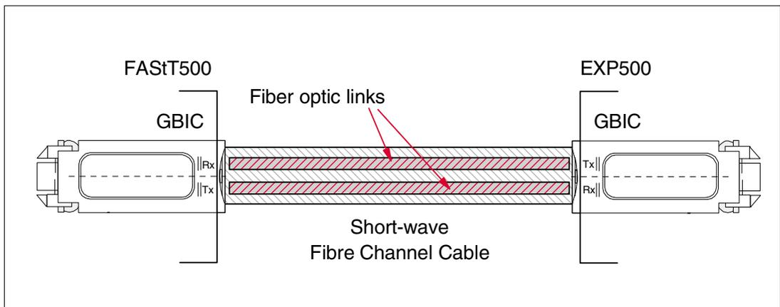
Figure 2-6 Cable diagram
