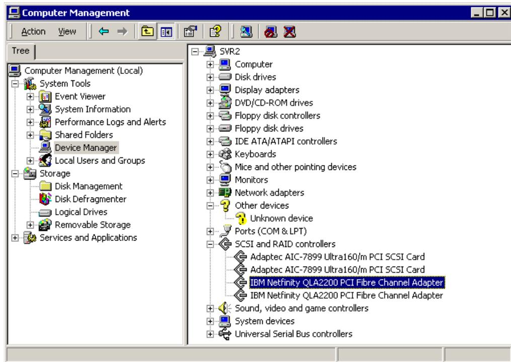
Figure 3-3 Windows automatic device detection
