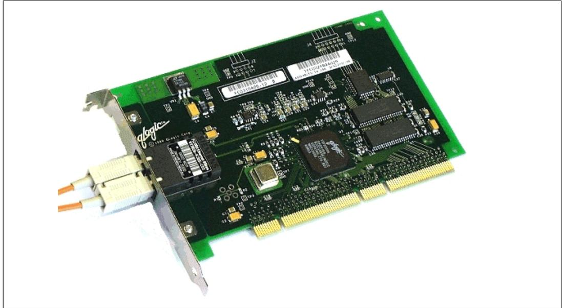
Figure 2-4 FASTT Host Bus Adapter
