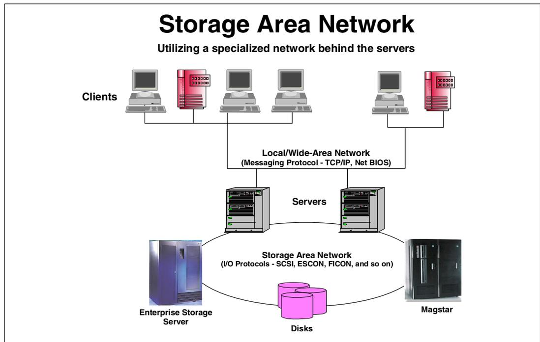
Figure 1-1 Topology of a network using SAN storage
