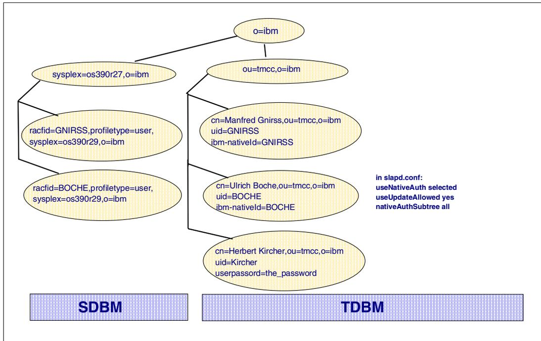
Figure 7 Mixed authentication methods within one subtree
