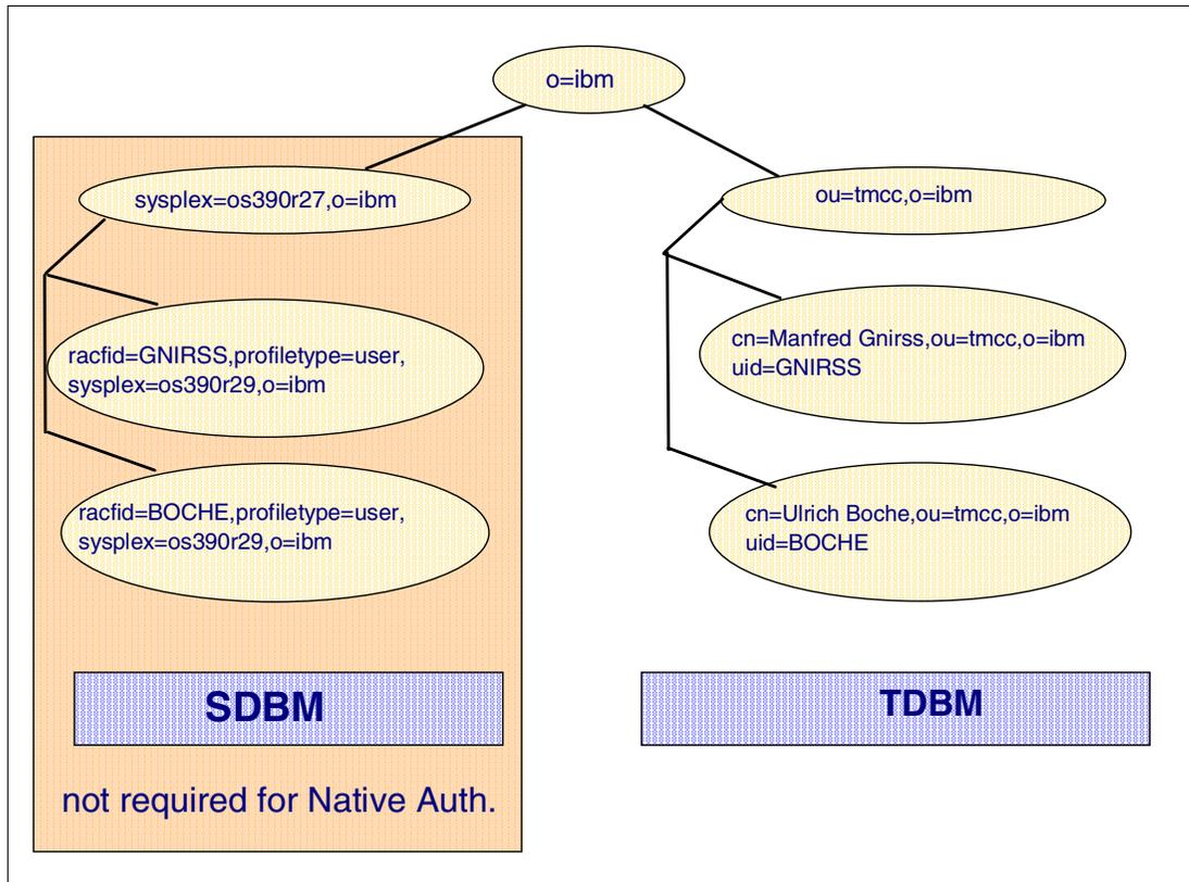
Figure 5 Native authentication and identification using TDBM
