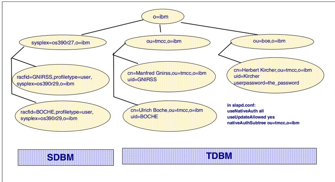
Figure 8 Mixed authentication methods in separate subtrees
