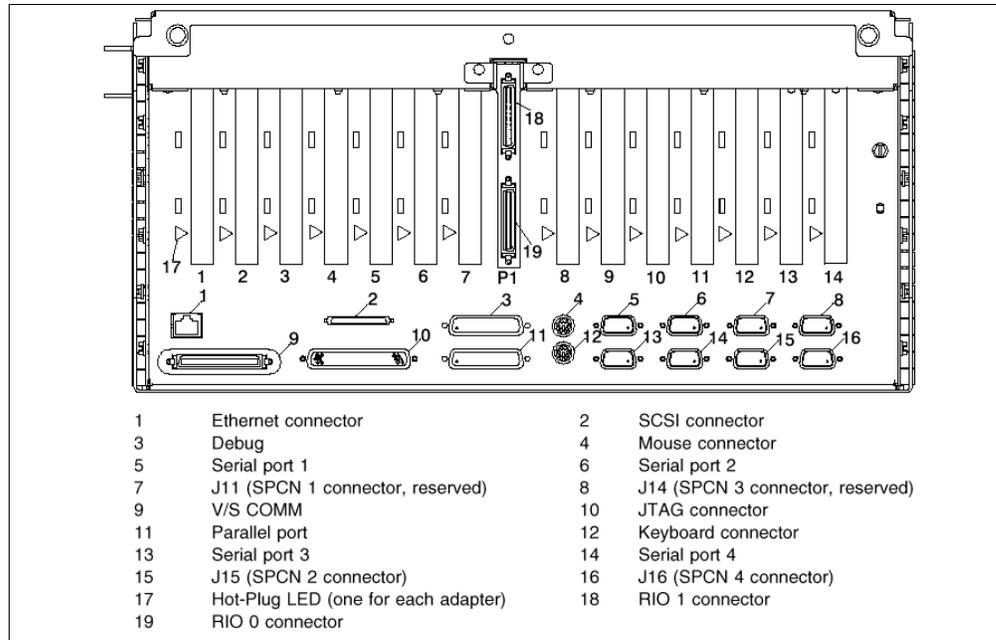
Figure 5. I/O Drawer Rear View
