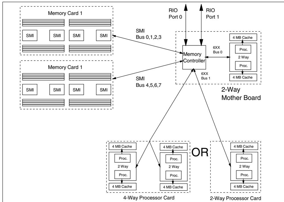
Figure 2. Model 6H1 System Schematic for 2-, 4-, or 6-Way 600 or 668 MHz SMP within the CEC
