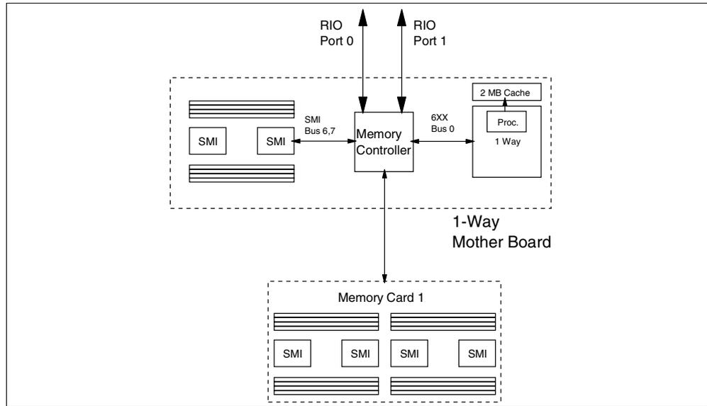
Figure 3. Model 6H1 System Schematic for 1-Way Processor within the CEC
