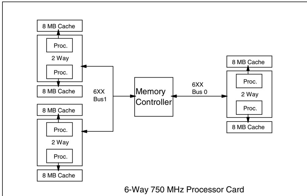
Figure 4. pSeries 660 Model 6H1 System Schematic for 6-Way Processor 750 MHz
