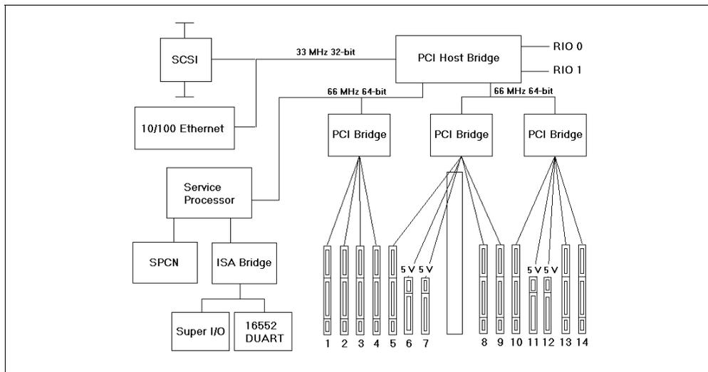
Figure 7. Slot Layout of the I/O Drawer
